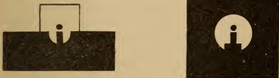
FIGURE 10. Correct Appearance of the Open and Peep Sights in Aiming.
