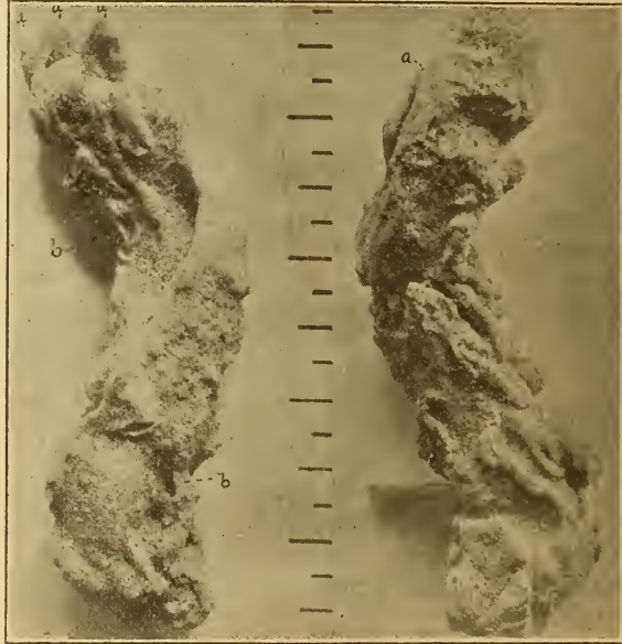
FIG. 1. Spiral fulgurite from Cutler, Wisconsin, showing opposite sides. The units in the scale are inches. a, a, a , in the figure at the left, horn-like protuberances terminating the fulgurite. b of the same portion of the figure, corrugations broken open and exhibiting thin-walled tubes. a in figure at the right, point of emergence of main channel (hidden in the view).
