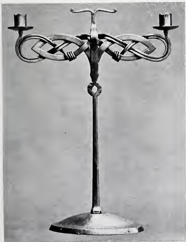
Candlestick, showing the use of plaited strands of iron, a method employed before the eleventh century, also filed and tooled work.
