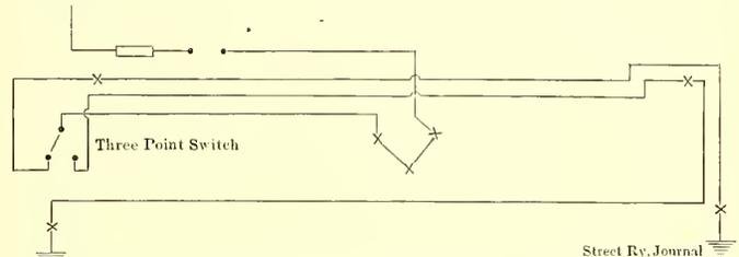
FIG. 2.—WIRING DIAGRAM TO ACCOMPLISH THE SAME PURPOSE AS IN FIG. 1, BUT USING THREE-POINT SWITCH
