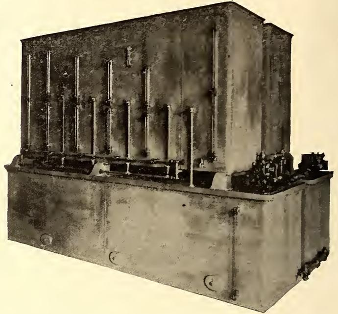
FIG. 2.—EXTERIOR VIEW OF OIL FILTER, 600-GAL. CAPACITY
