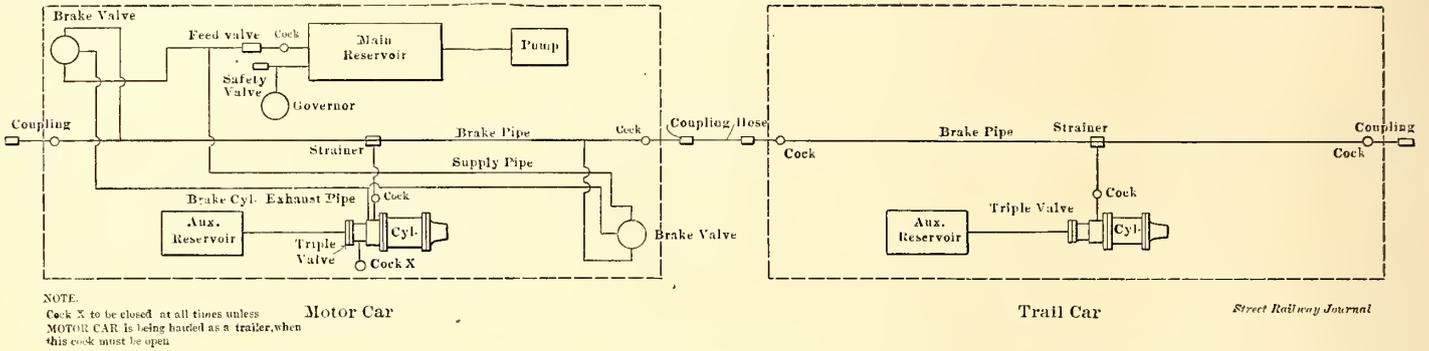
FIG. 1.—SHOWING GENERAL ARRANGEMENT OF BRAKE FIXTURES AND PIPING ON ONE MOTOR AND ONE TRAIL CAR
