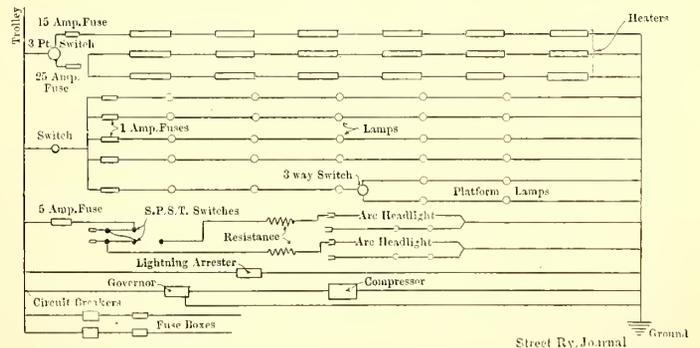
FIG. 16.—SCHEMATIC DIAGRAM OF CAR WIRING
