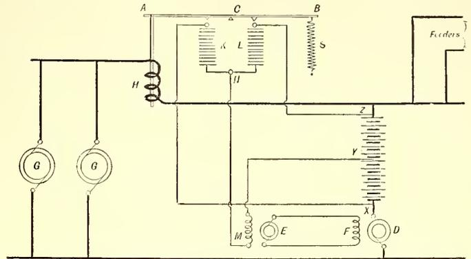
ELECTRICAL CONNECTIONS FOR STORAGE BATTERY REGULATOR
