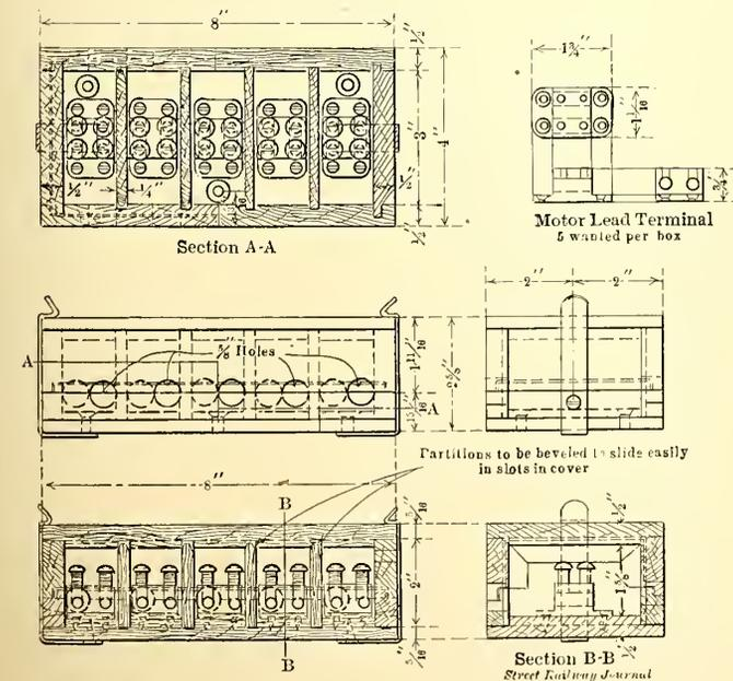
FIG. 14.—SECTIONS OF JUNCTION BOX FOR MOTOR LEADS
