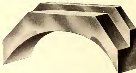
FIG. 3.—SECTIONAL VIEW OF CAR JOURNAL BEARING AFTER RUNNING 72,000 MILES
