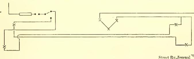
FIG. 4.—SECOND WIRING SCHEME, WHERE HOOD HEADLIGHTS ARE USED, USING A THREE-POINT SWITCH ON THE TROLLEY SIDE OF THE CIRCUITS
