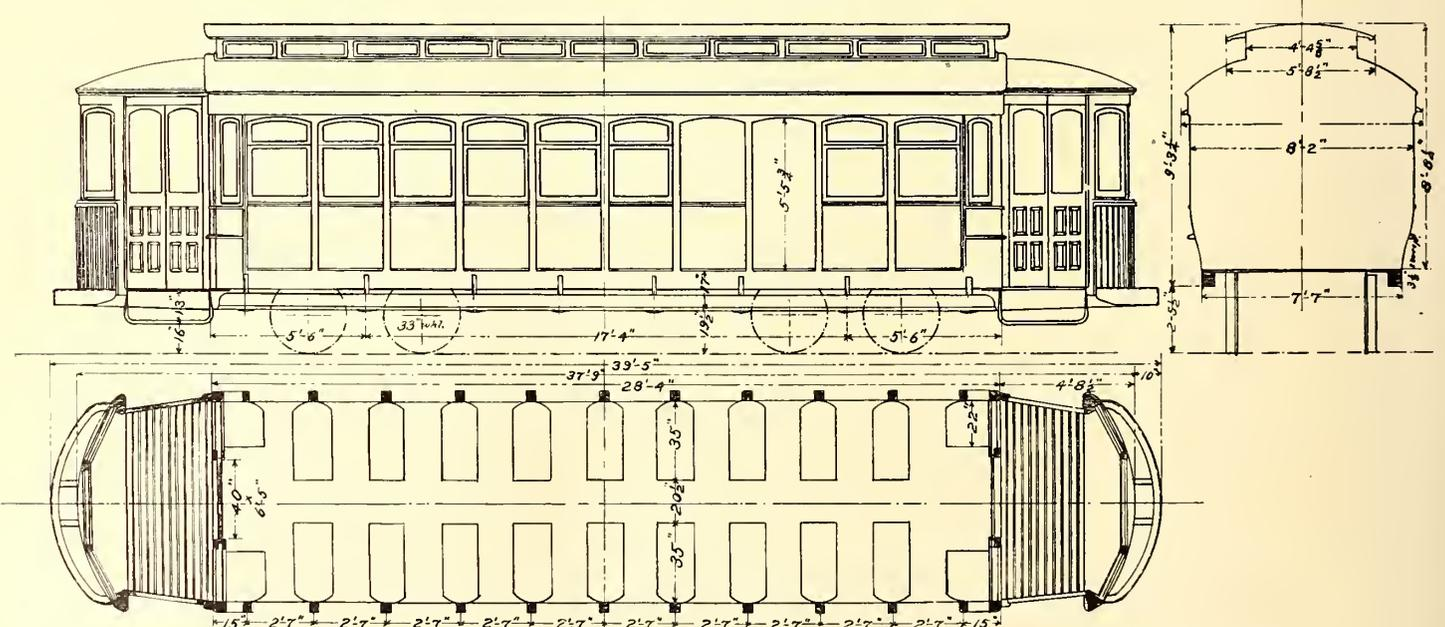
FIG. 2.—PLAN, SIDE ELEVATION AND END ELEVATION OF STANDARD DOUBLE-TRUCK CONVERTIBLE CAR
