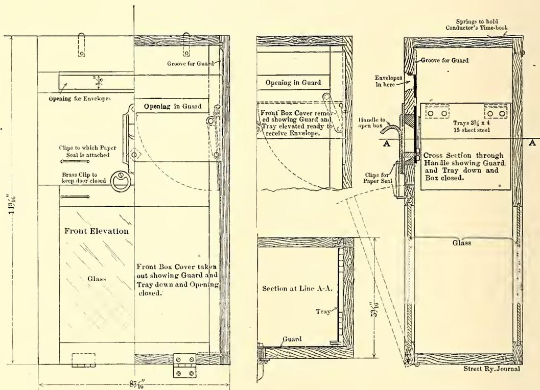
DETAIL DRAWING, SHOWING CONSTRUCTION AND OPERATION OF RECEIPT BOX FOR TRANSFER ENVELOPES PLACED IN THE CARS OF THE BROOKLYN RAPID TRANSIT COMPANY
