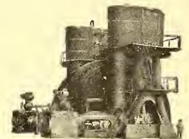
Twin Horizontal and Vertical Corliss Engine
