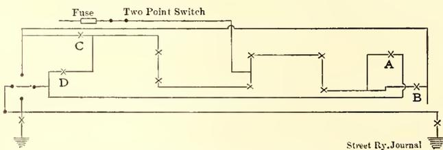
FIG. 6.—WIRING ARRANGEMENT ADAPTED TO PERMIT THE USE OF A 32-CP HEADLIGHT
