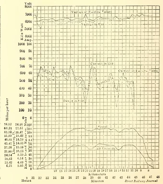
FIG. 11.—CURVES OBTAINED FOR SPEED, AIR PRESSURE, CURRENT, VOLTAGE AND POWER, WITH CAR S (WEIGHT, 77,900 KG)
