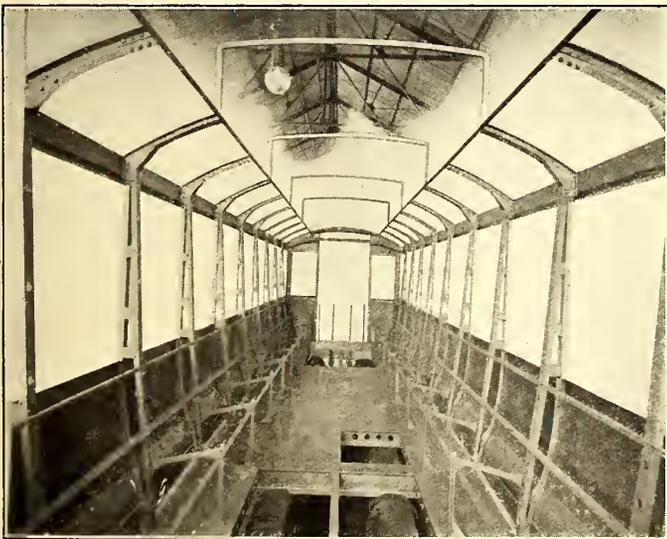
VIEW OF UNFINISHED INTERIOR, SHOWING THE GENERAL CONFIGURATION OF THE STEEL CAR FRAMING
