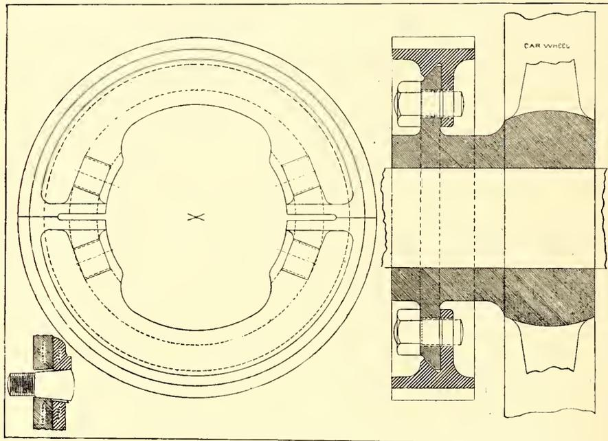
ILLUSTRATIONS SHOWING DETACHABLE RIM GEAR APPLIED TO EXTENDED HUB OF CAR WHEEL
