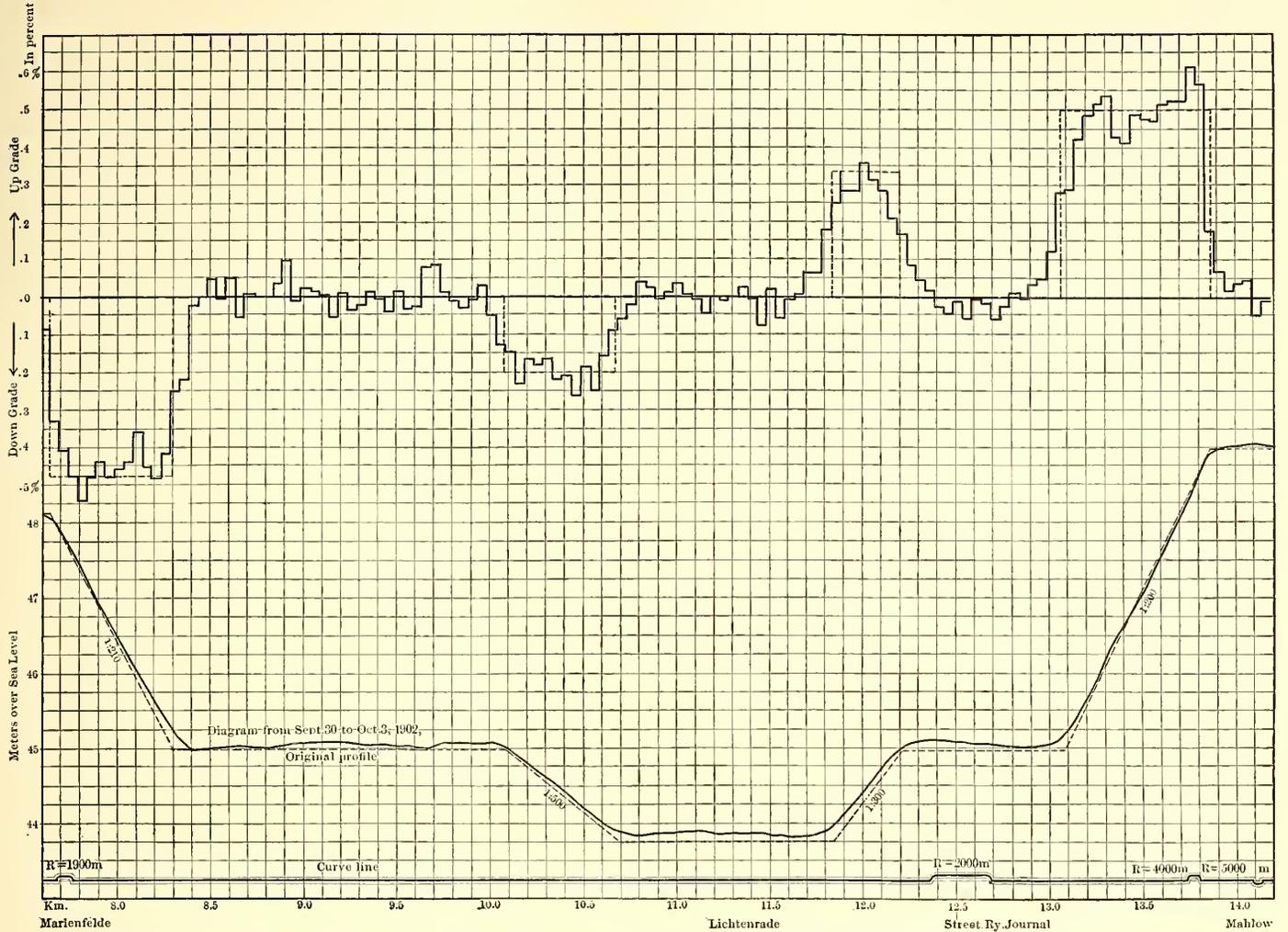
FIG. 1.—PROFILE OF THE EXPERIMENTAL TRACK BETWEEN MARIENFELDE AND MAHLOW
