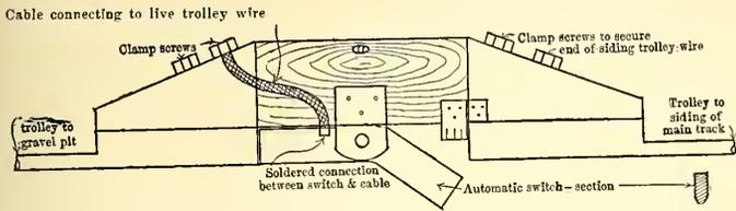
AUTOMATIC OVERHEAD SWITCH FOR GRAVEL ROADS
