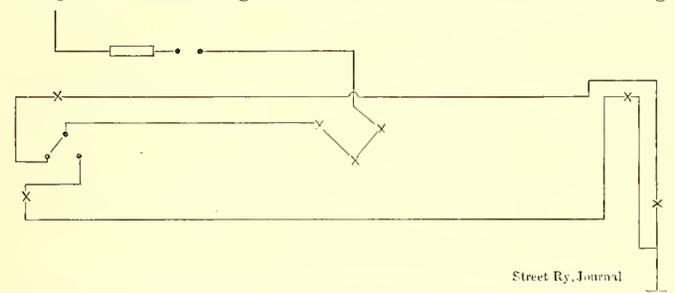
FIG. 3.—ILLUSTRATING THE CONNECTION USED WHEN THE HEADLIGHTS ARE PLACED ON THE HOODS
