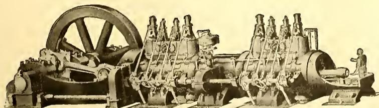
Allis-Chalmers Four-Cycle, Double-Acting Gas Engine
