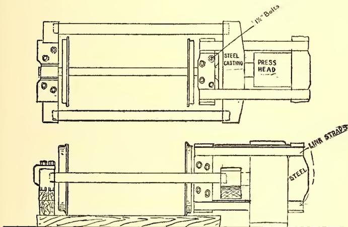
FIG. 1.—ARRANGEMENT OF WHEEL COMPRESSOR FOR TESTING AXLES
