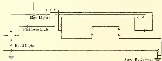
FIG. 5.—SHOWING WIRING DIAGRAM WHERE TWO CIRCUITS ARE EMPLOYED, AND WHERE HEADLIGHTS, PLATFORM LIGHTS AND SIGN LIGHTS ARE INTERCHANGED
