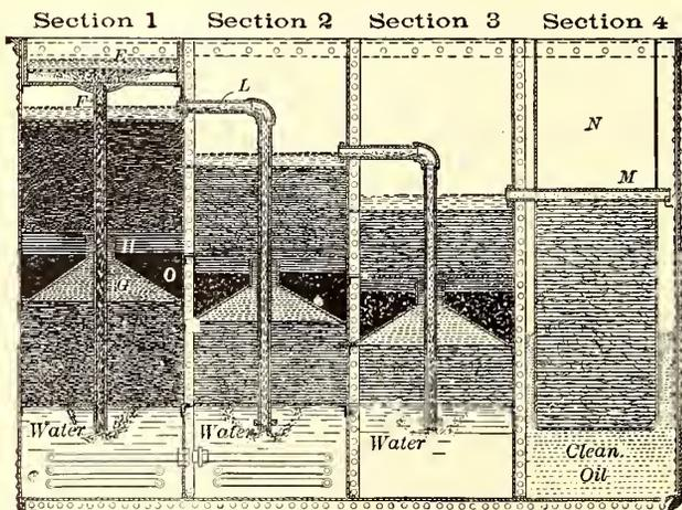
FIG. 1.—SECTIONS OF OIL FILTER TO ILLUSTRATE ITS OPERATING PRINCIPLES
