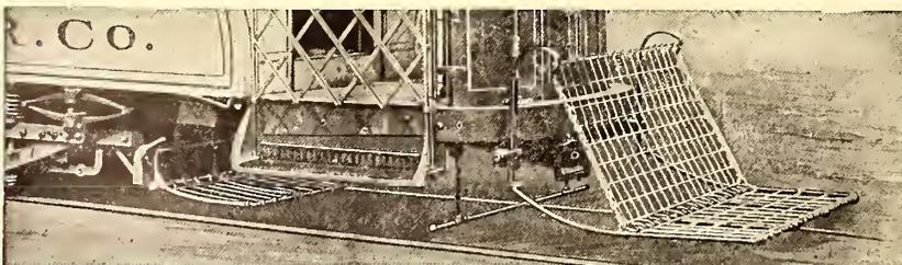
Are life-saving devices which cannot fail. Fender can be dropped at the will of motorman. Readily folded and transferred. Light, effective, durable. Wheel Guard is automatic and can be used in connection with fenders or independently. Easily adjusted.
