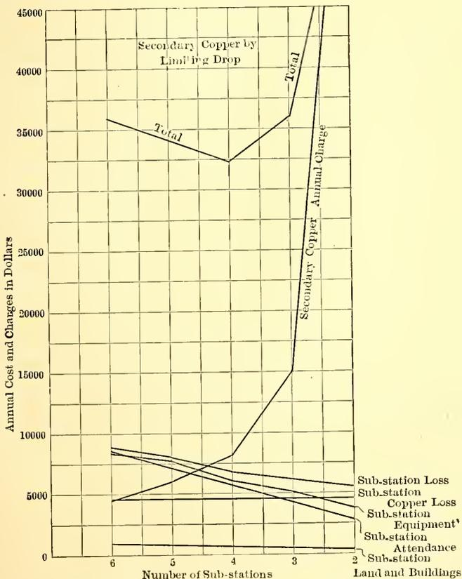
FIG. 2.—CURVE SHOWING RESULTS OF COMPUTING SAME PROBLEM BY LIMITING DROP METHOD
