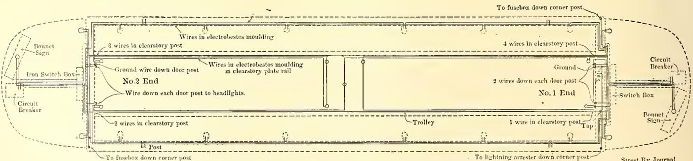
FIG. 19.—PLAN OF LIGHT WIRING
