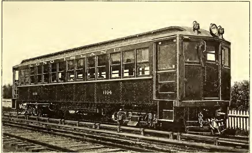
VIEW OF STEEL MOTOR CAR, SHOWING CONTACT RAIL PROTECTION
