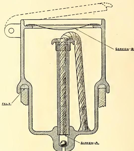
TYPE OF OIL CUP USED ON OLD-STYLE MOTORS, WITH GRAVITY GREASE CUPS
