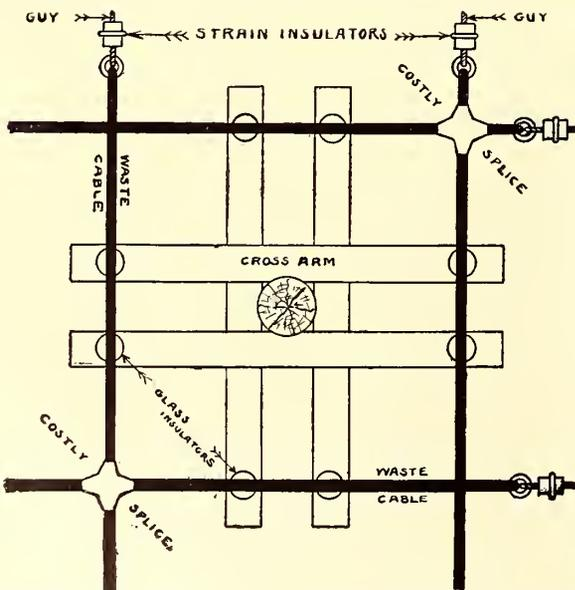
FIG. 2.—OLD METHOD OF MAKING SPLICES AT CORNERS
