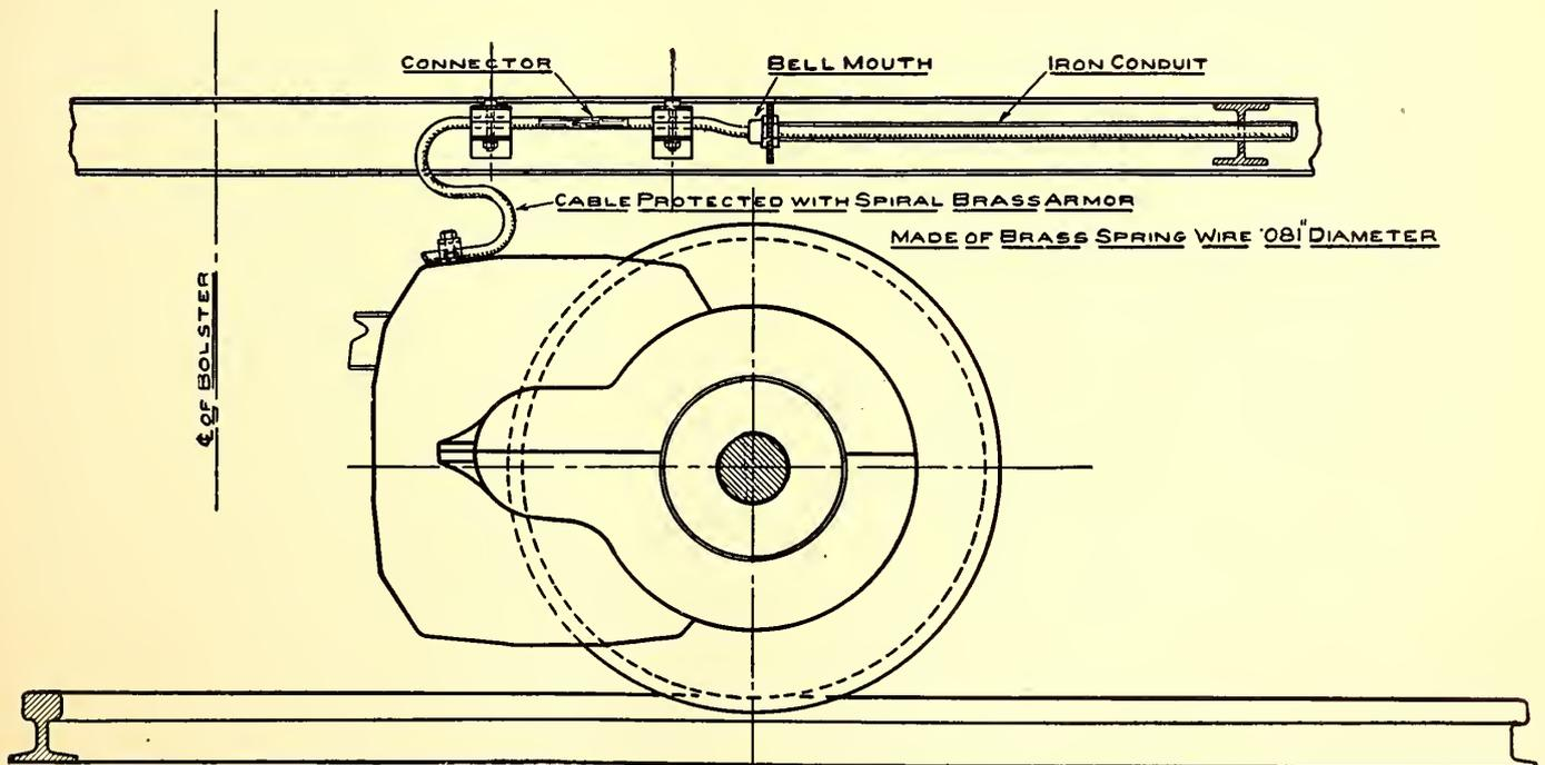
METHOD OF SECURING THE HEADS WHERE BELL-MOUTH IS USED WHEN WIRES ARE LAID IN IRON CONDUIT
