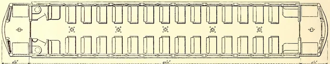
SEATING PLAN OF NEW STEEL MOTOR CAR FOR THE NEW YORK CENTRAL RAILROAD
