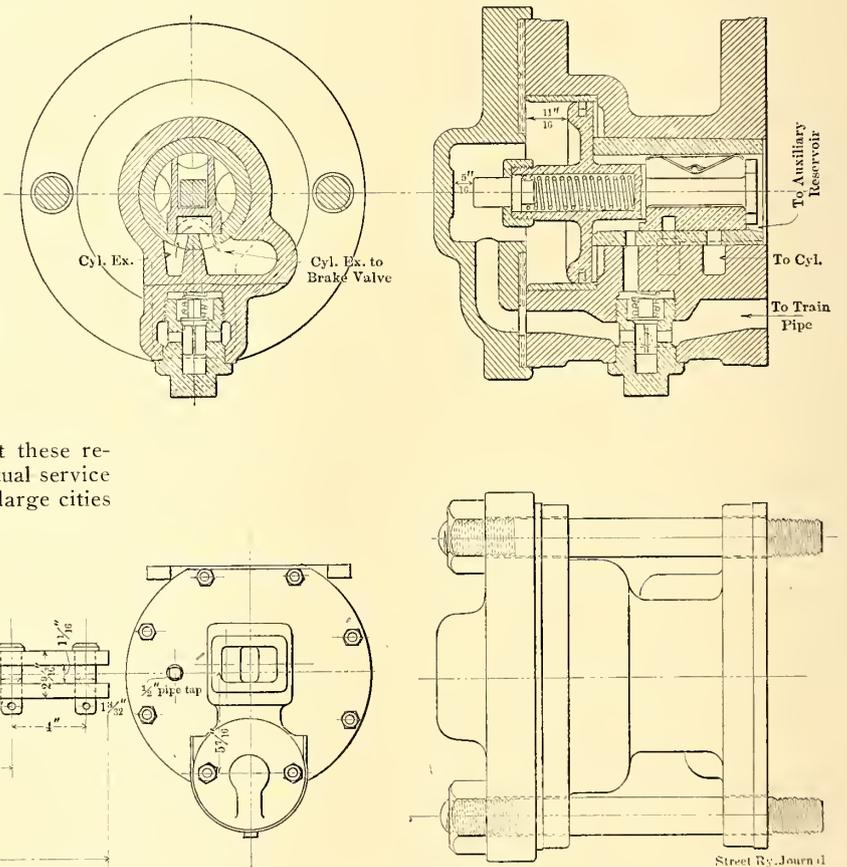
FIG. 2.—SECTIONS AND OTHER DETAILS OF SURFACE TRACTION TRIPLE VALVE
