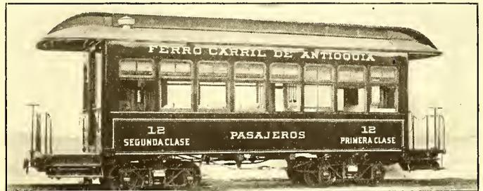
EXTERIOR VIEW OF CAR FOR ANTIOQUIA, COLOMBIA, FITTED WITH FIRST AND SECOND-CLASS COMPARTMENTS
