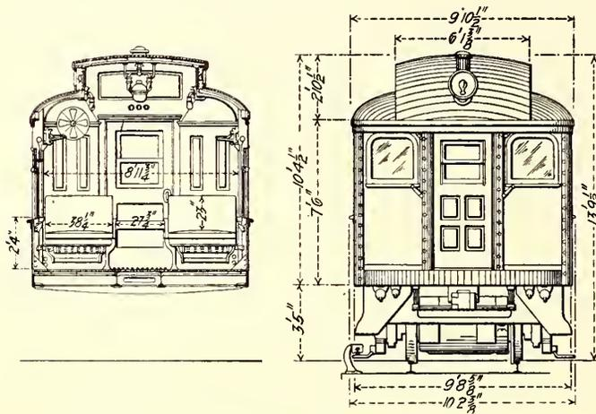
CROSS-SECTION AND END VIEW OF NEW YORK CENTRAL STEEL MOTOR CAR
