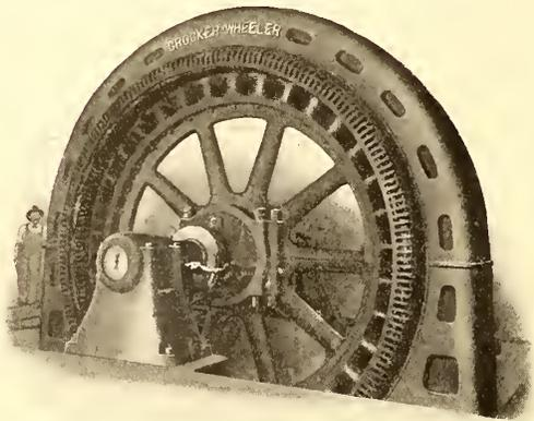
4000 K.V.A ENGINE TYPE A.C. GENERATOR
