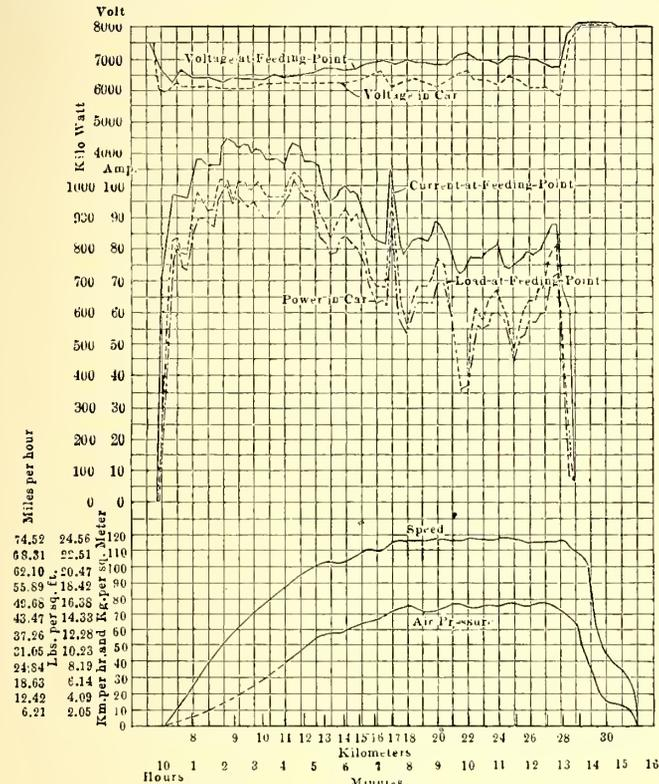
of this tube, extending from 3 to 5 meters before the front end of the car, the air pressure was the same as that recorded near the front end of the car, and, as was also noticed in the present experiments, a cone of compressed air was formed before the mouth of each tube. Equal air pressures were obtained when the mouths of the tubes were placed out of the center line of
