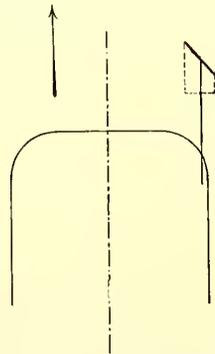
FIG. 14.—PRESSURE-MEASURING DISC
