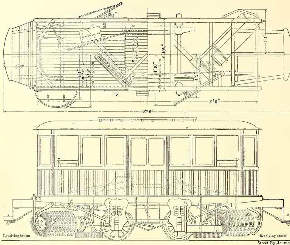
FLOOR PLAN AND SIDE ELEVATION OF PHILADELPHIA SNOW SWEEPER, SHOWING THE LOCATION OF THE SNOW-FIGHTING APPARATUS, BRACING AND OTHER DETAILS
