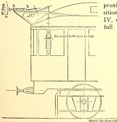
FIG. 13.—SPECIAL AIR-PRESSURE MEASURING APPARATUS
