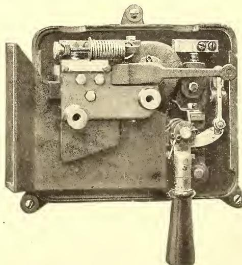
The arc is broken in a powerful magnetic field which effectually opens the circuit under the most severe conditions of short circuit, and reduces damage to the arcing contacts to a minimum. The contacts where the arc occurs when the circuit is opened, are surrounded by a shield of insulating and arc resisting material, which prevents the arc from being communicated to any part of the breaker or case.
