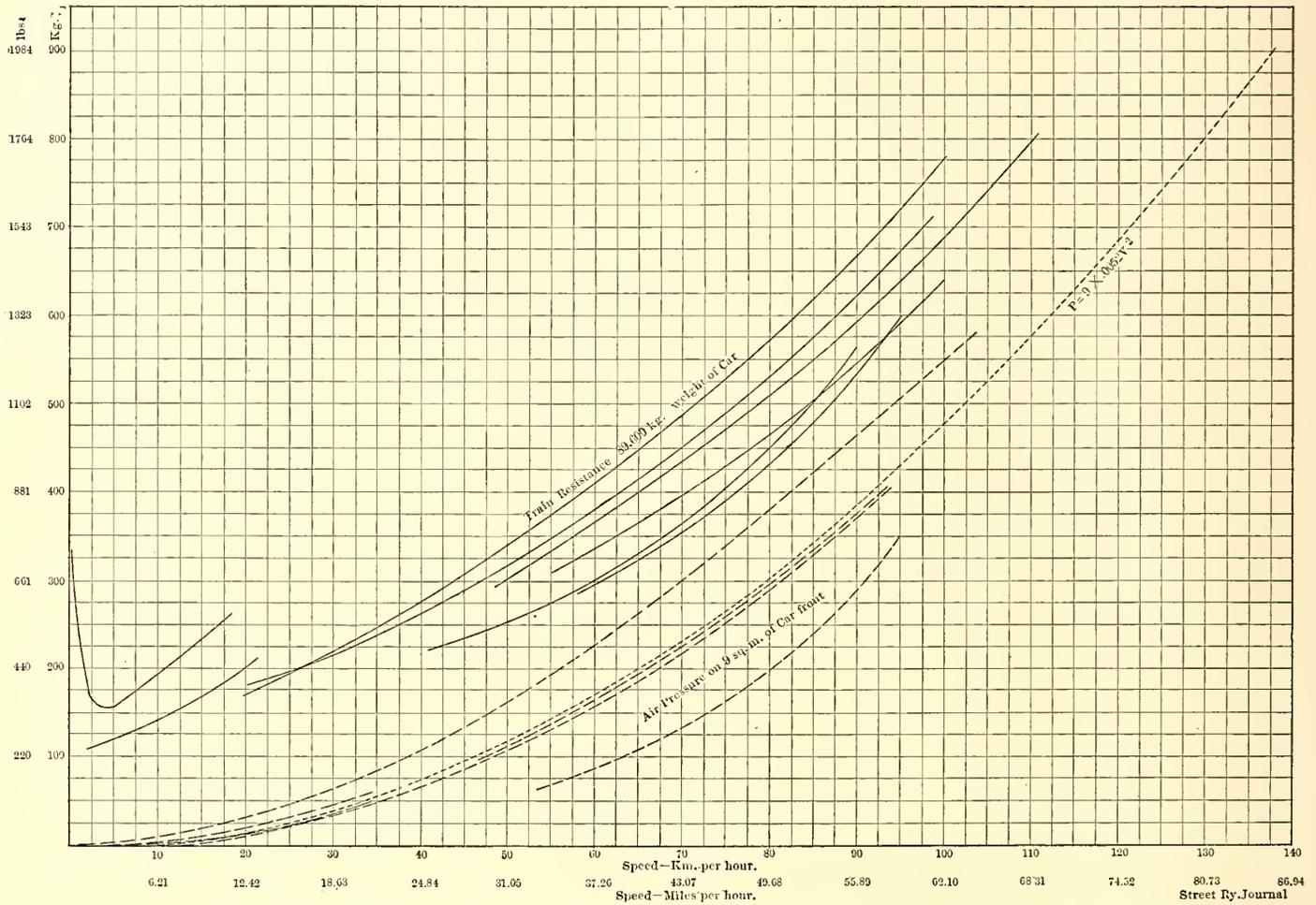
FIG. 4.—RESISTANCE OF CAR A, DETERMINED BY THE COASTING RUNS IN THE FALL OF 1902
