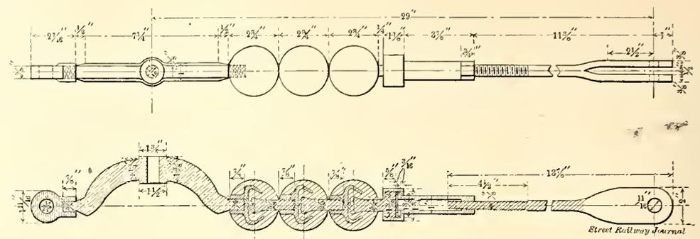
FIG. 4.—OVERHEAD CONSTRUCTION FOR SURFACE LINE UNDER ELEVATED STRUCTURE
