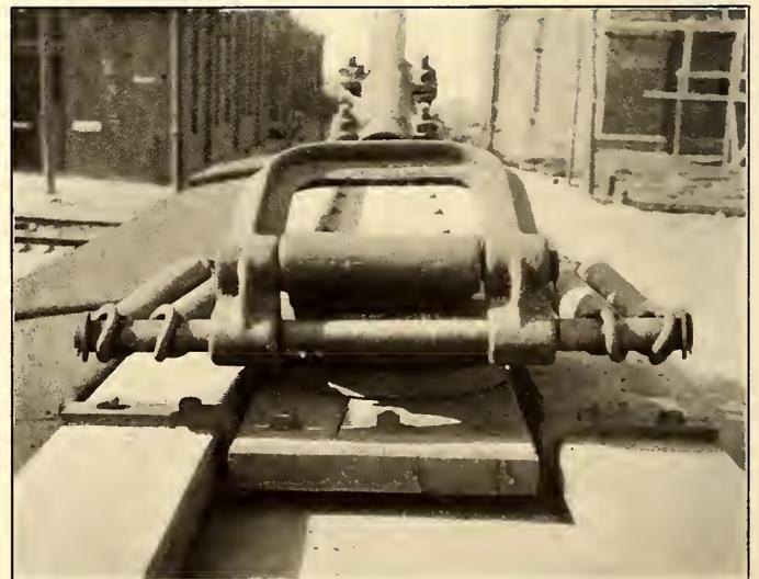
FIG. 10.—ROOF OF CAR, SHOWING METHOD OF SECURING TROLLEY BASE BLOCK TO RUNNING BOARDS
