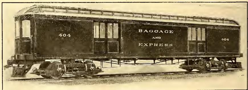
Heaviest type used in interurban service. Length over body, 56-ft. Mounted on Brill No. 27-E-3 Trucks.
