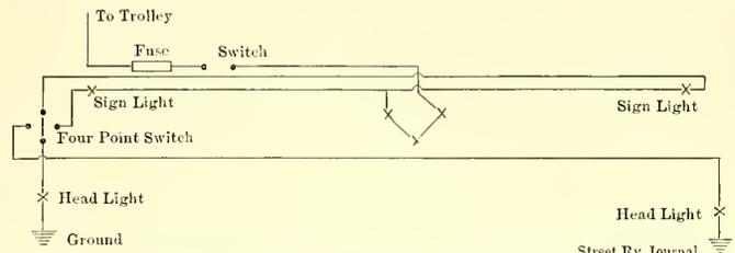
FIG. 1.—WIRING DIAGRAM FOR FIVE-LIGHT CIRCUIT, WITH FOUR-POINT SWITCH FOR HEADLIGHTS AND PLATFORM LIGHTS
