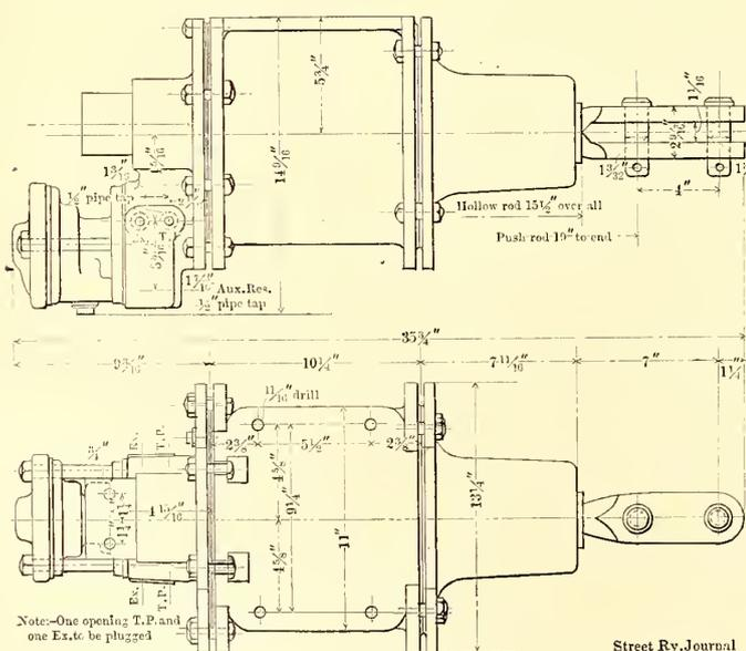
FIG. 3.—BRAKE CYLINDER FOR SURFACE TRACTION, INDICATING PIPE CONNECTIONS IN THE PRESSURE HEAD
