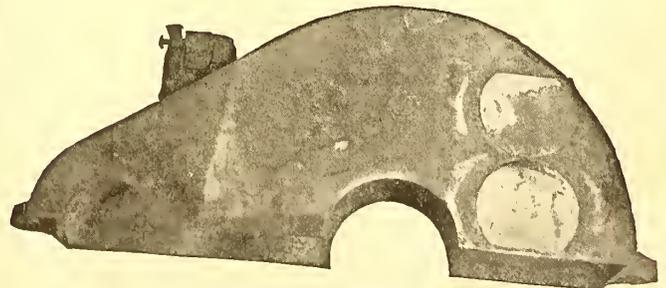
Broken Gear Case which we repaired.
