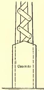
FIG. 3.—METHOD OF PLACING CONCRETE ABOUT BASE OF LATTICED POLE
