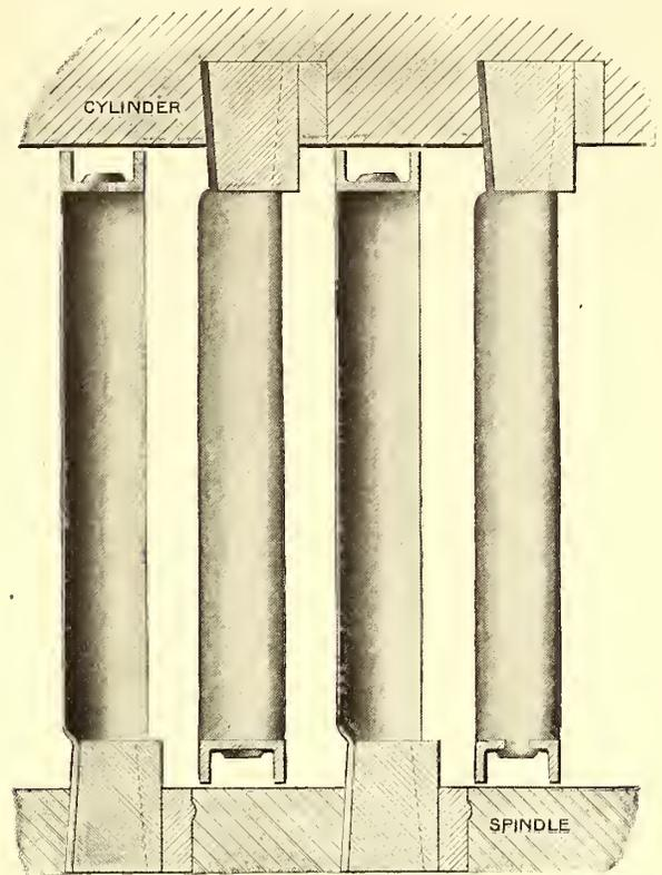
FIG. 2.—ILLUSTRATING THE METHOD OF FASTENING THE BLADES AS WELL AS THE CHANNEL-SHAPED SHROUD RING
