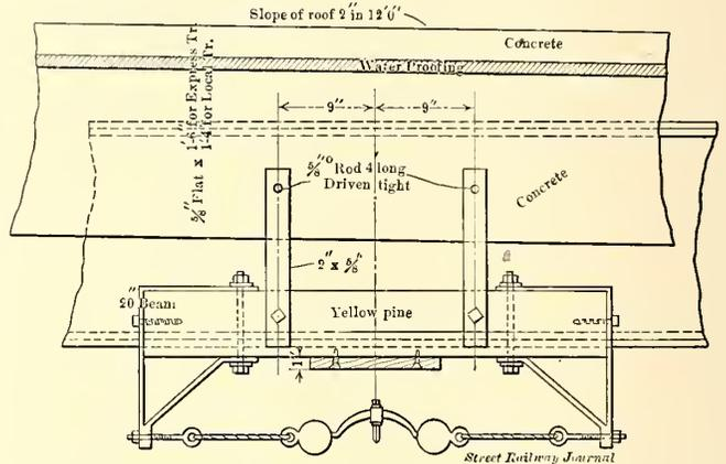
FIG. 5.—OVERHEAD CONSTRUCTION FOR SUBWAY LOCAL TRACKS
