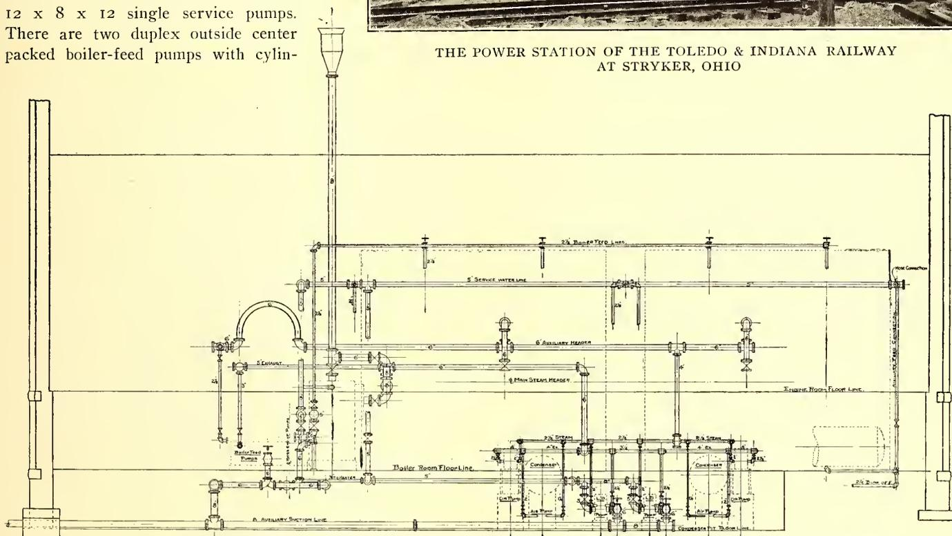
LONGITUDINAL ELEVATION OF PIPING, AS VIEWED FROM BOILER ROOM WITH PARTITION WALL REMOVED
