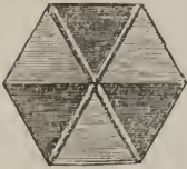
Tessellated appearance of a plate of sulphate of potash seen by polarized light.
