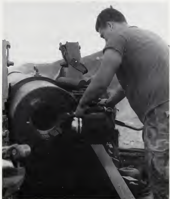
Department of Defense Photo (USMC) A372603 A Marine gunner cleans the breech of his 175mm gun after firing. The M107 175mm gun had a range of 32,000 meters, the longest in the Marine inventory.
