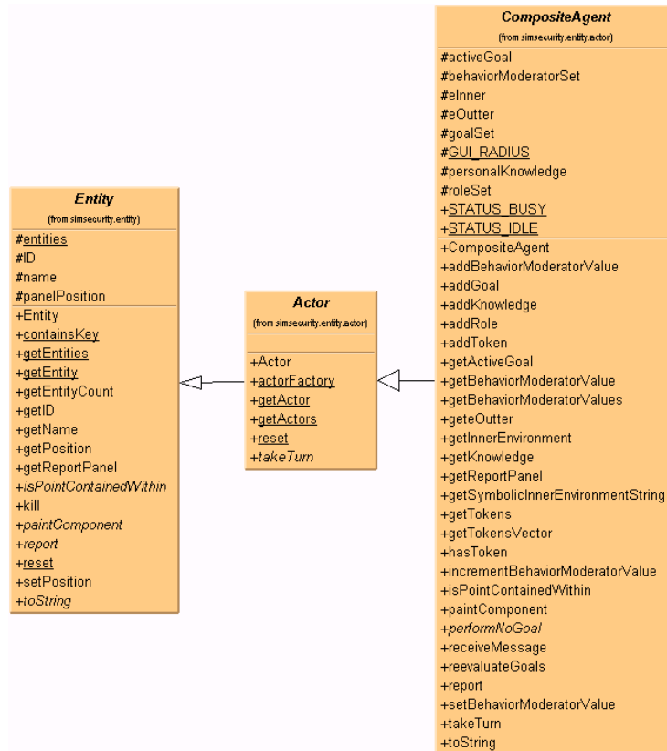
Figure 43. The main classes in the actor package are the Actor and CompositeAgent classes, which inherit from the Entity class.
