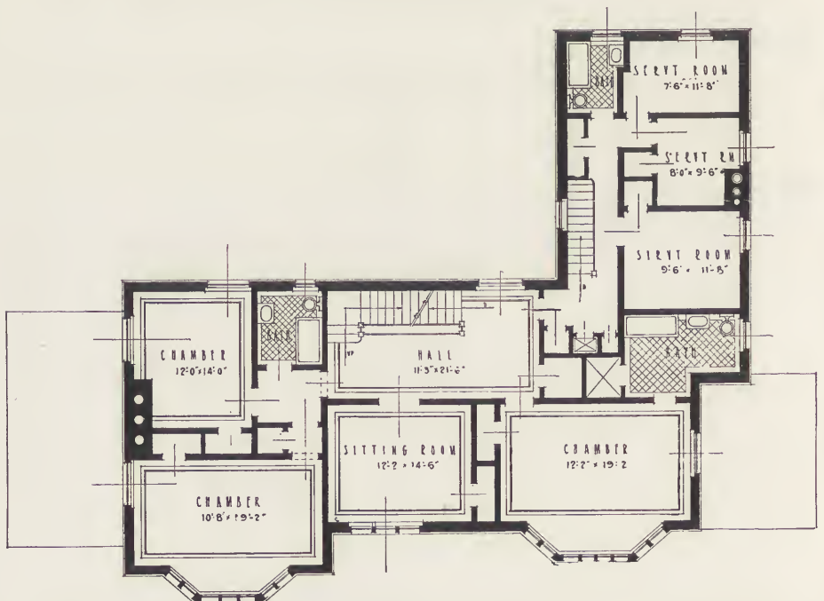
FIG. 78. SECOND FLOOR PLAN—RESIDENCE OF JOHN B. VAN HAELEN, ESQ., HARTSDALE, N. Y. Frank J. Forster, Architect.
