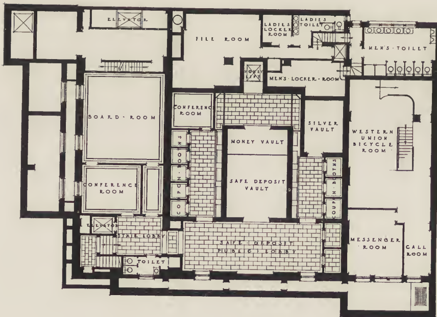
BASMENT PLAN COMMERCIAL NATIONAL BANK BUILDING, WASHINGTON, D. C. Waddy B. Wood, Architect.
