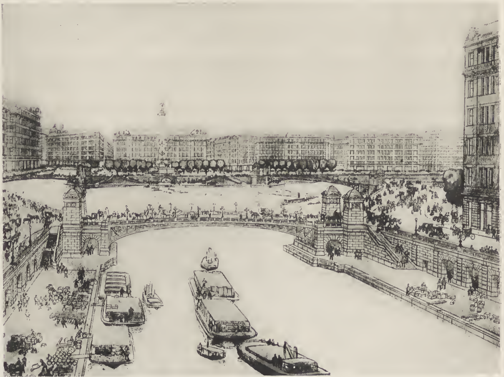
SHOWING ARRANGEMENT OF STREETS AND WAYS FOR TEAMING AND RECEPTION OF FREIGHT BY BOAT, AT DIFFERENT LEVELS, ON THE CHICAGO RIVER AT LAKE MICHIGAN.
