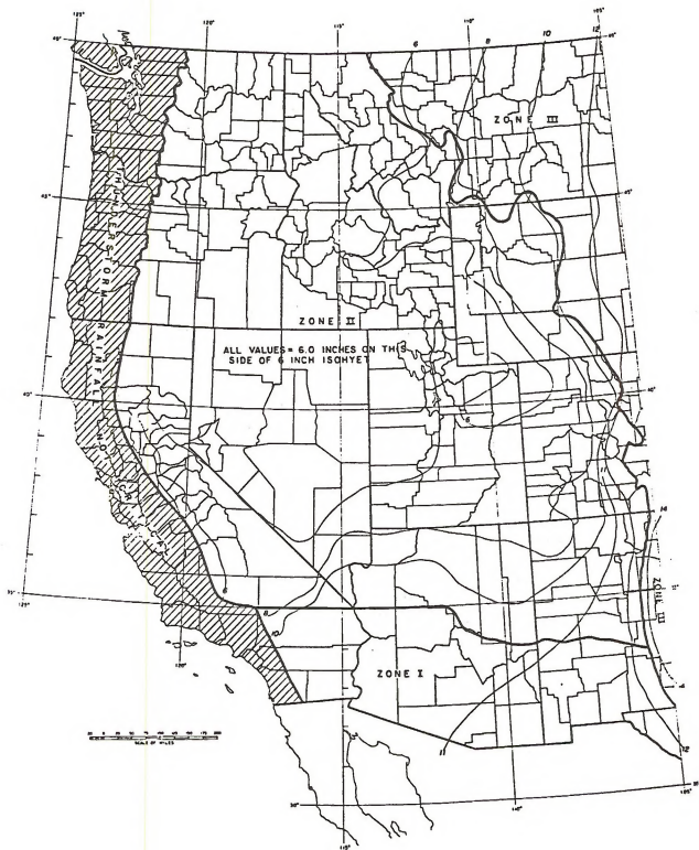
Figure II-7 Probable maximum thunderstorm 1-hour rainfall (point values in inches) for area west of 105° meridian. (USER, 1973)
