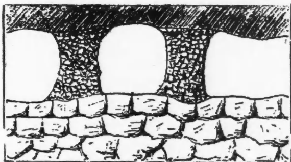
Supports in a gallery in Laurion.
