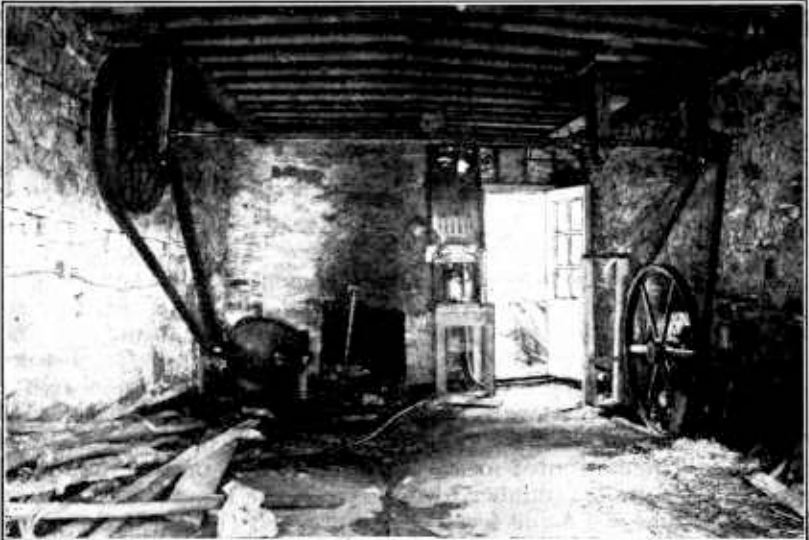
FIGURE 10.—Stepping up the speed of a 10 by 3 foot steel overshot wheel in New Jersey. The large sprocket wheel at the right is keyed to the axle of the water wheel outside the wall and is connected by chain drive with a small sprocket wheel on the overhead line shaft, which in turn is belted to a 7-kilowatt generator at the left
