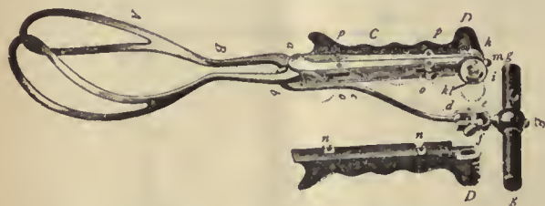
Fig. 8.—A, blade; B, shanks; C, handle; DD, detachable rubber side pieces; E, the axis traction attachment; a, socket between shanks for hook b, of traction rod; d, ball end of rod; e, clamp socket for d; f, thumb-screw for screwing the ball and socket joint; gg, the rubber cross bar; h, the ordinary Elliot wheel and threaded bar; l, an additional wheel with a half-threaded slot on opposite side, which both form the lock; KI, a quarter-circle slot and piece limiting the motion of lock-wheel or small knob on lock-wheel; n, n, metallic lugs which hold side pieces in place; oo, grooves in the metal for the reception of the lugs; pp, screws passing antero-posteriorly through the metal and flat where they pass through the grooves; a quarter turn of these screws, locks or unlocks the side pieces securely to the metallic portion.
