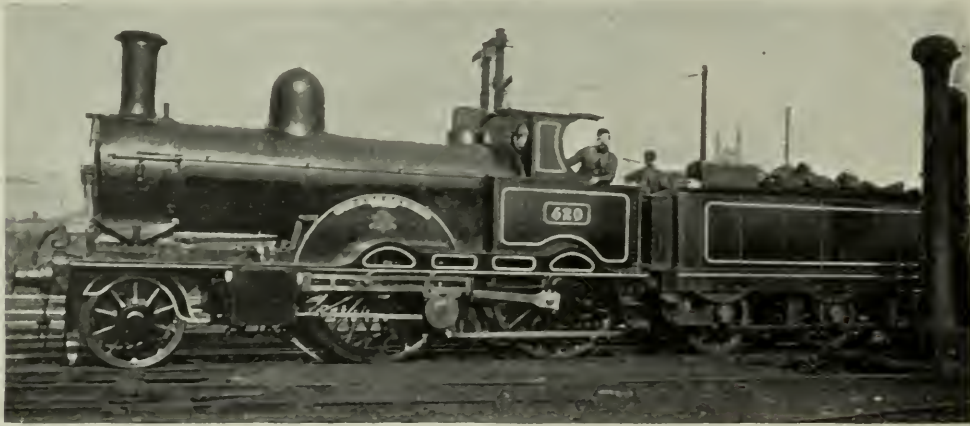
Compound Engine used on London and North Western.
