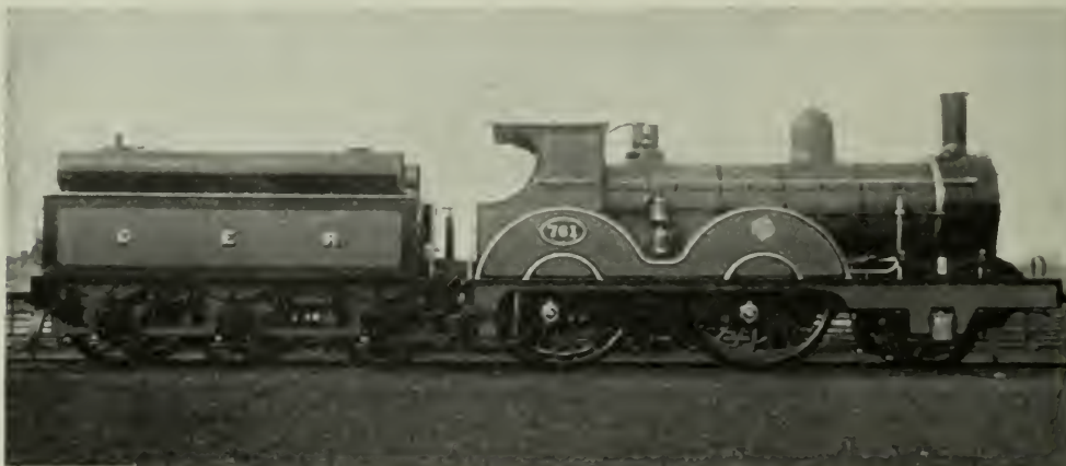
Oil-burning Engine on the Great Eastern Railway.
