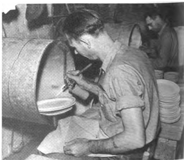
Spraying is another process that requires local exhaust ventilation to protect the worker against the toxic vapors. Photograph by courtesy of the Tennessee Conservation Department.
