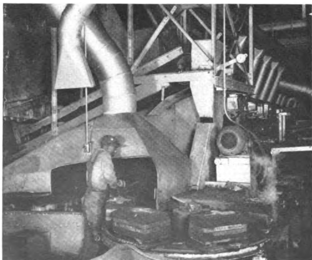
This well-enclosed and ventilated shakeout station in the Chevrolet-Grey Iron Foundry at Saginaw, Mich. has an inward flow of air from 200 to 250 linear feet per minute. Photograph by courtesy of General Motors Corp.
