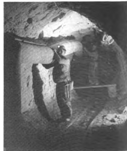
A ventilating tube at the working face of a copper mine provides cool, fresh air for the miners. Photograph by courtesy of Anaconda Copper Mining Co.
