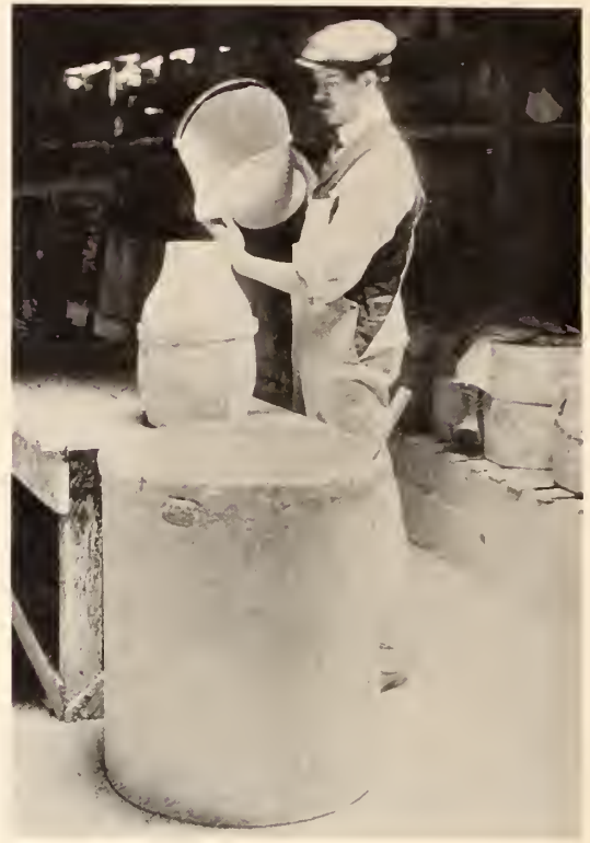
Pouring "Slip" into the Mould
