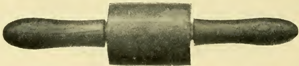
FIG. 5.—HAND ROLLER FOR FLATTENING THE STRAW.
