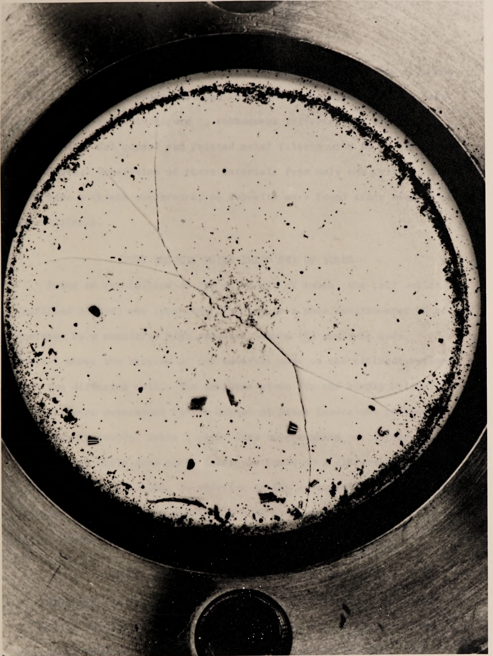
FIGURE 1.— In-Line Filter, Showing Black Iron Powder and Brass Turnings. (3.5 X)
