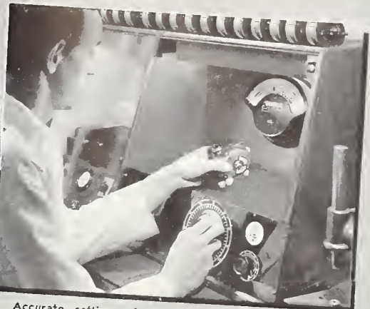
Accurate setting of the 5 speeds of the Revere Camera is determined by synchronizing the shutter with the stroboscope.
