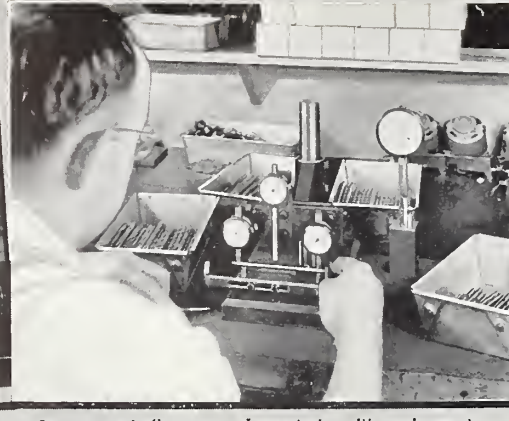
Revere spindles are inspected with micrometer gauges and must not vary more than .0025 of an inch.
