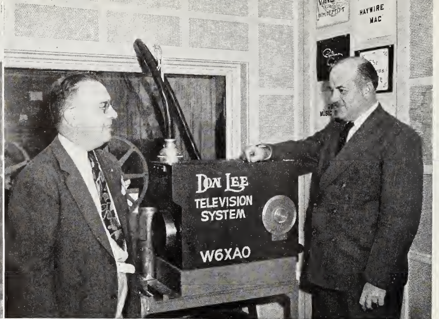
• Another view of movie telecasting apparatus showing close hook-up of projector with television camera. Pictures are projected directly into camera.
