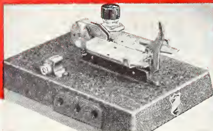
B&H FILM SPLICER, MODEL 136 (above, left). Splices all 16mm. and 8mm. film faster because each film end is positioned but once, and because ends are sheared in same operation that brings bonding areas together. Makes exclusive B&H diagonal splice —strong and pliable—quiet in sound film projectors. Is the basis of the Add-A-Unit line. Price, $14.65.
