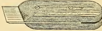
FIG. 98.—Knife for freezing microtome, made from the blade of a carpenter's plane.
