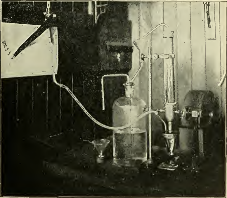
FIG. 7.—The Churn Elutriator (Hilgard's) for the physical analysis of soils.
