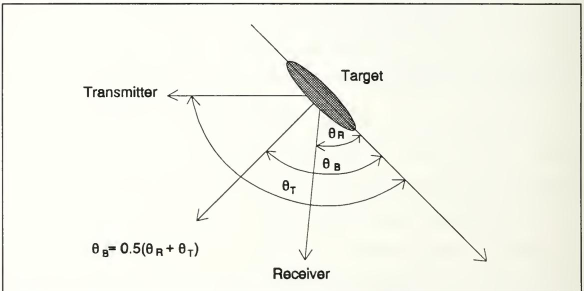
Figure 3. Bistatic angle for target strength calculation.
