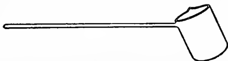
FIG. 155.—A dipper made entirely of glass and holding 17.5 cubic centimeters for measuring the acid.
