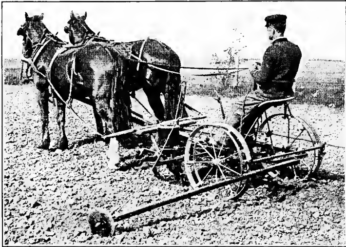
FIG. 39. — A two-row corn-planter arranged with wire to drop the kernels into hills.
