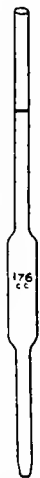
FIG. 153.—Pipette holding 17.6 cubic centimeters, used in measuring milk in the Babcock test.
