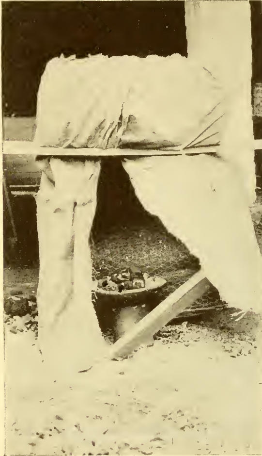
FIG. 81.—Apparatus for drying specimens. The bundle of plants rests upon two poles. From this, cloth is draped about the charcoal-burning heater, being lined with woven wire to prevent its being blown into the fire.
