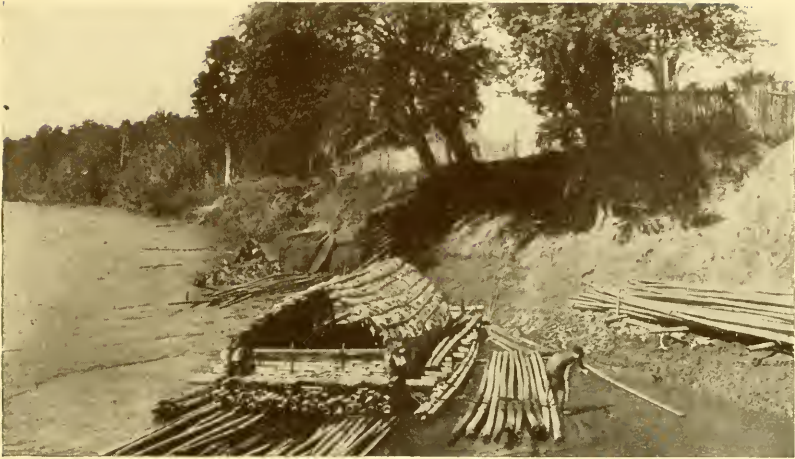
FIG. 75.—Raft-building on the Cauca River, Colombia. The ever-present bamboos and palms supply the material needed.
