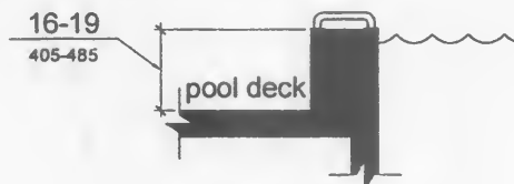
Figure 1009.4.2 Transfer Wall Height
