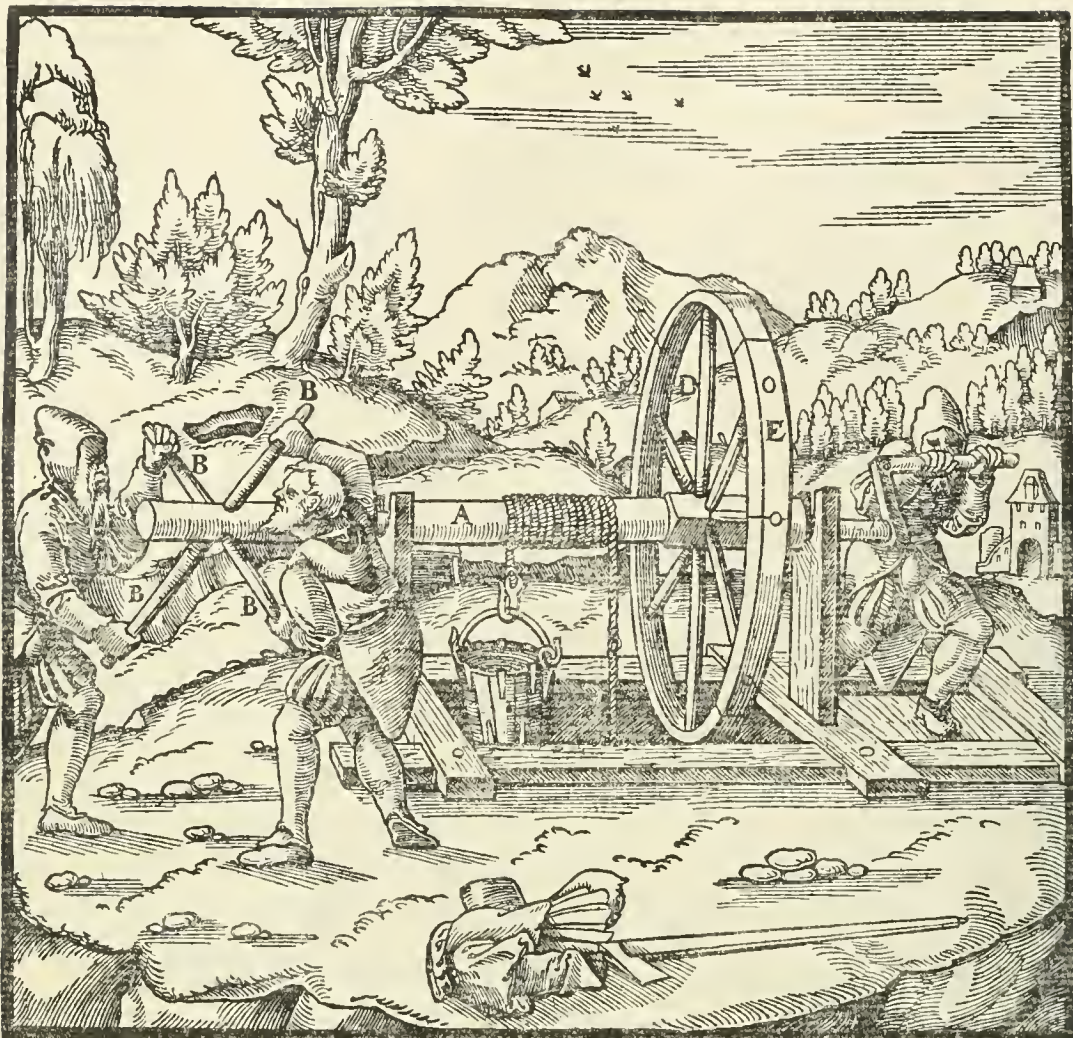
A—BARREL. B—STRAIGHT LEVERS. C—USUAL CRANK. D—SPOKES OF WHEEL. E—RIM OF THE SAME WHEEL.
