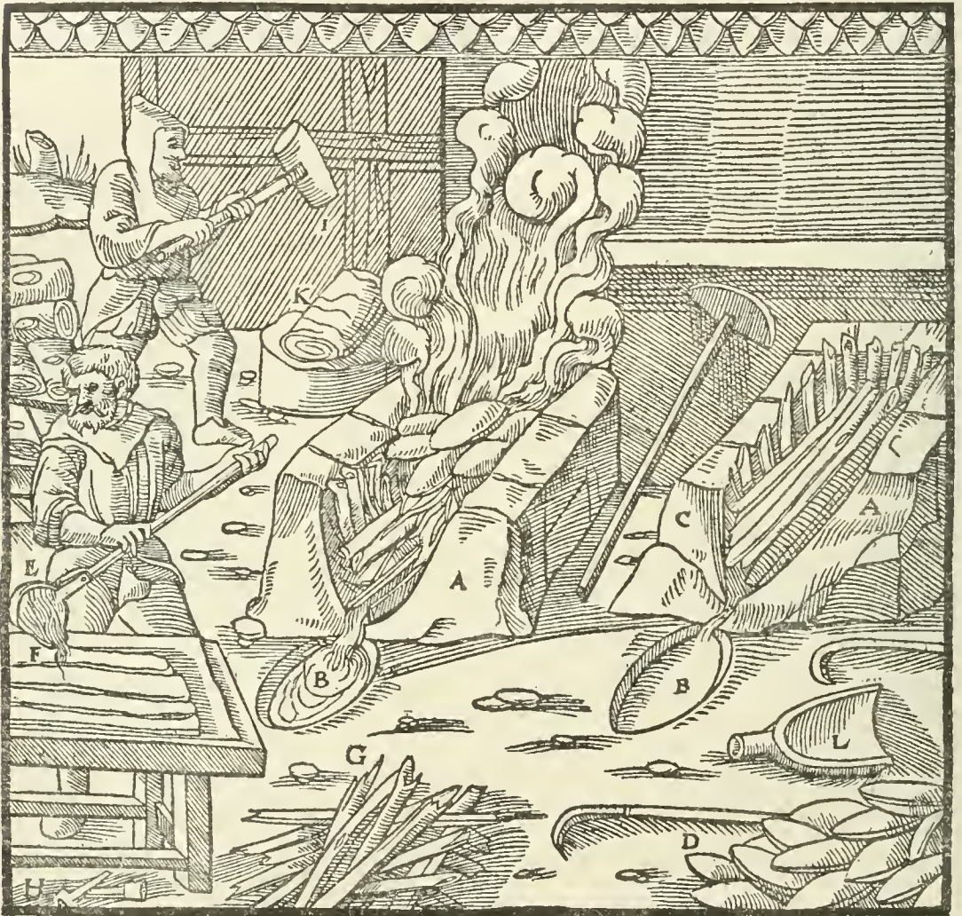
A—HEARTH. B—DIPPING-POTS. C—WOOD. D—CAKES. E—LADLE. F—COPPER PLATE. G—LATTICE-SHAPED BARS. H—IRON DIES. I—WOODEN MALLET. K—MASS OF TIN BARS. L—SHOVEL.
