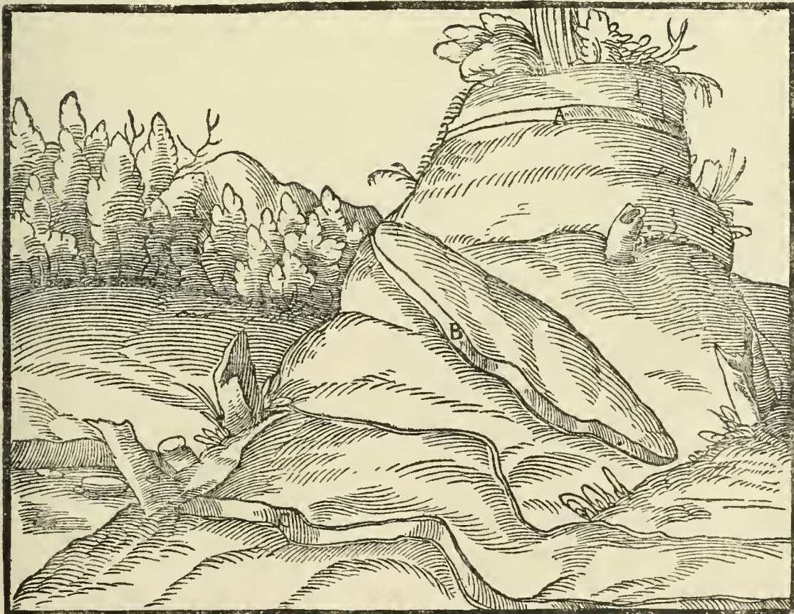
A—HORIZONTAL vena dilatata . B—INCLINED vena dilatata . C—CURVED vena dilatata .
