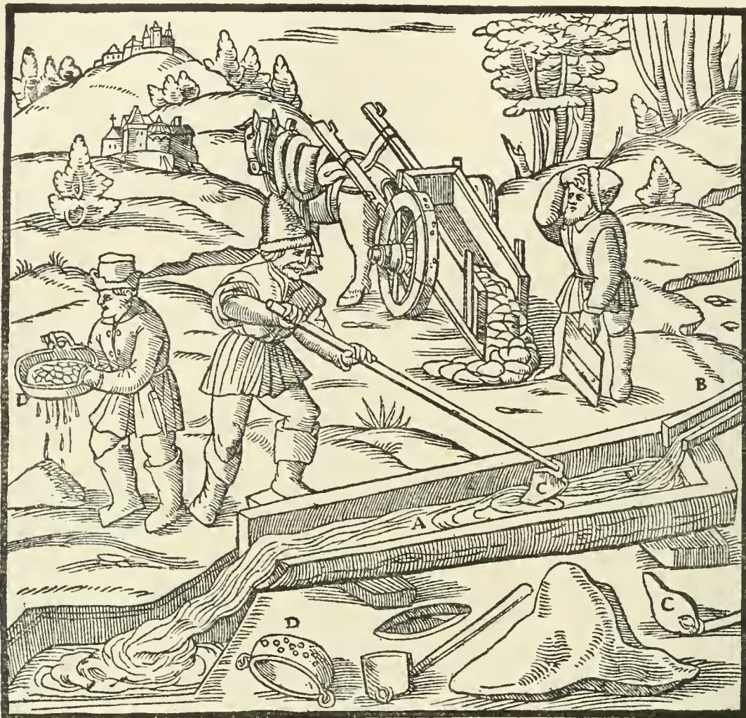
A—TROUGH. B—LAUNDER. C—HOE. D—SIEVE.
