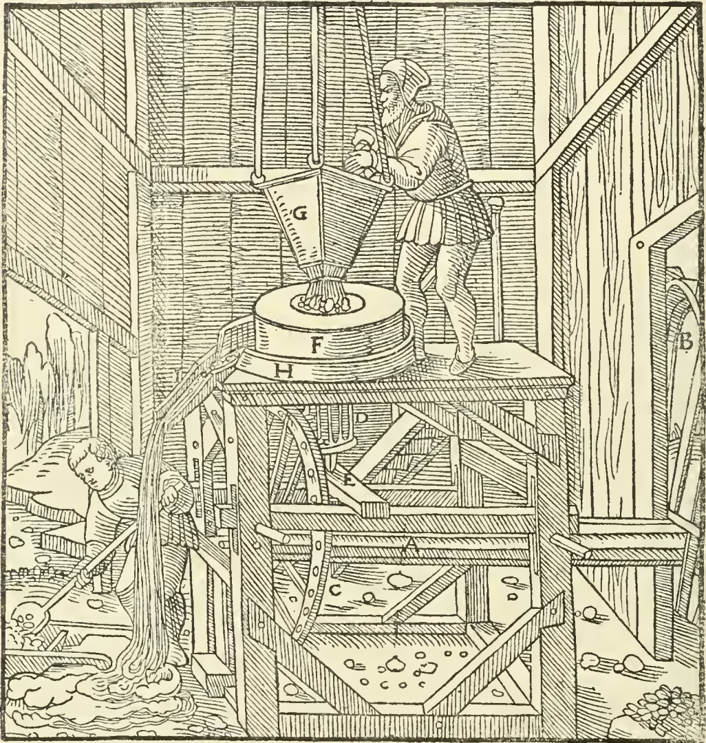
A—AXLE. B—WATER-WHEEL. C—TOOTHED DRUM. D—DRUM MADE OF RUNDLES. E—IRON AXLE. F—MILLSTONE. G—HOPPER. H—ROUND WOODEN PLATE. I—TROUGH.
