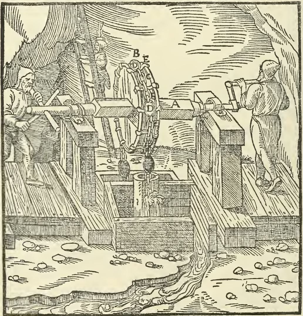
A—AXLE. B—DRUM. C—DRAWING-CHAIN. D—BALLS. E—CLAMPS.
