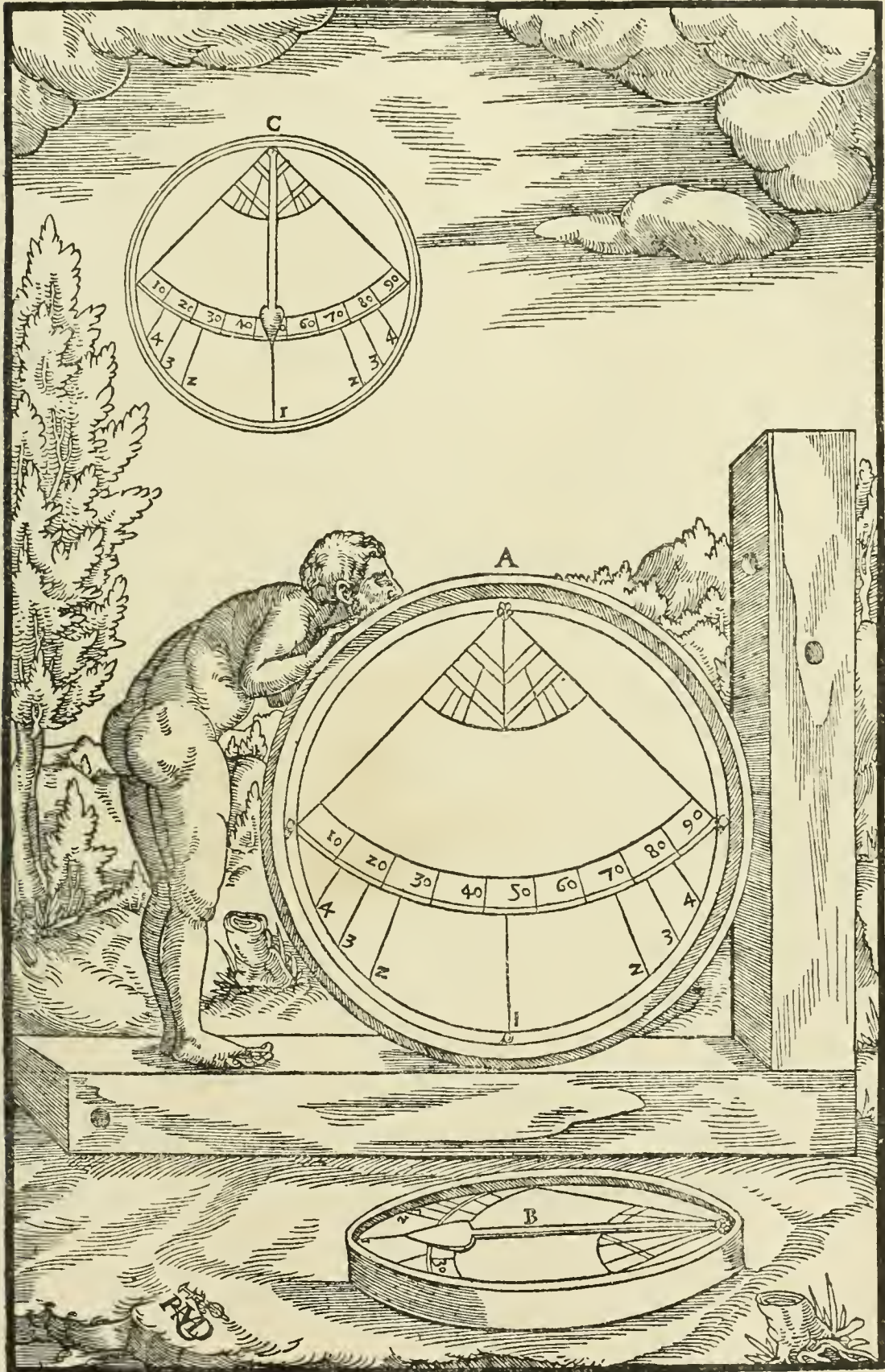
A—STANDING PLUMMET LEVEL. B—TONGUE. C—LEVEL AND TONGUE.
