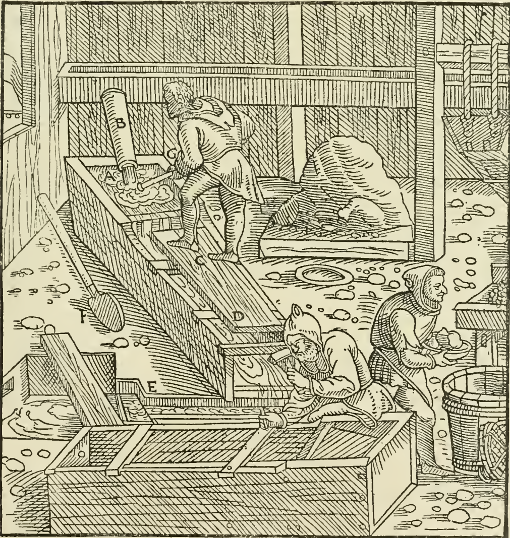
A—HEAD OF BUDDLE. B—PIPE. C—BUDDLE. D—BOARD. E—TRANSVERSE BUDDLE. F—SHOVEL. G—SCRUBBER.
