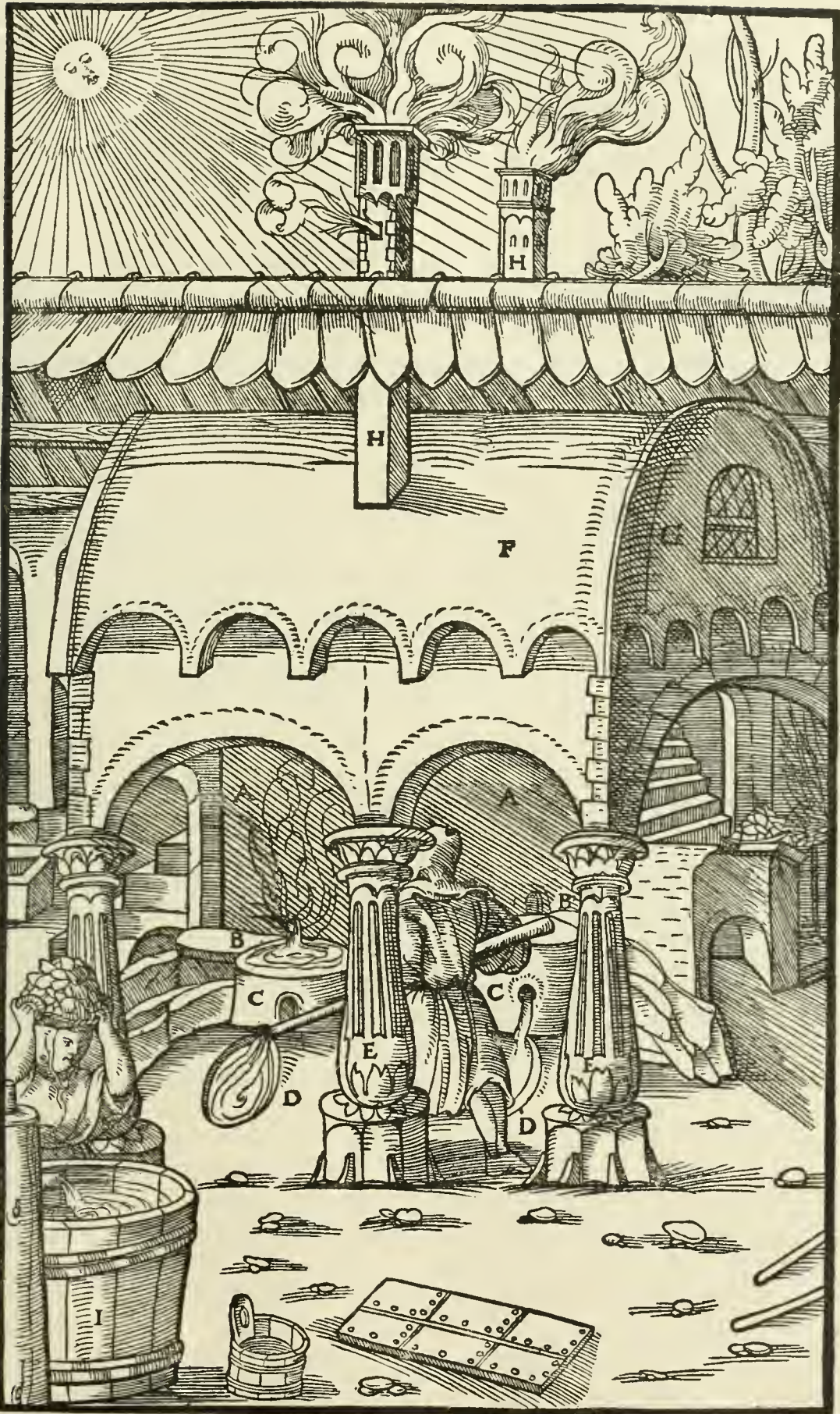
A—FURNACES. B—FOREHEARTHES. C—THEIR TAP-HOLES. D—DIPPING-POTS. E—PILLARS. F—DUST-CHAMBER. G—WINDOW. H—CHIMNEYS. I—TUB IN WHICH THE COALS ARE WASHED.
