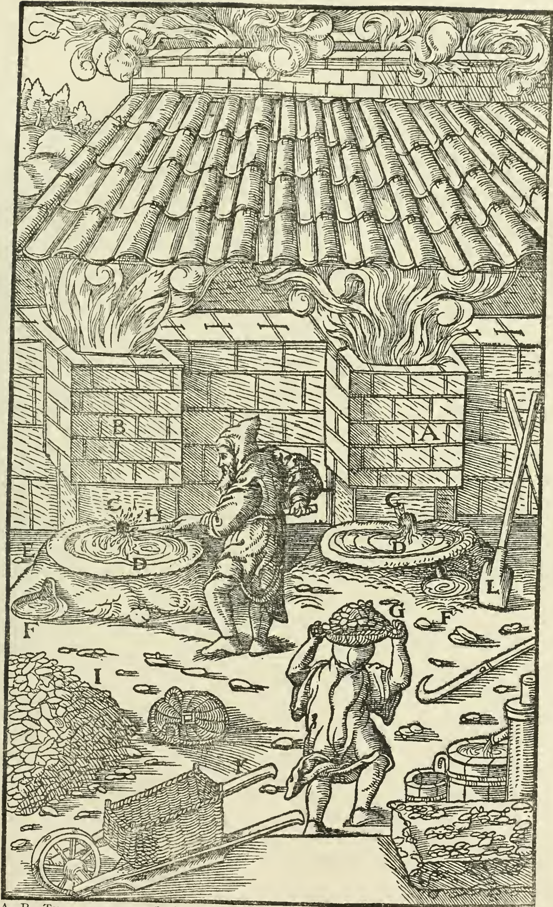
A, B—Two FURNACES. C—TAP-HOLES OF FURNACES. D—FOREHEARTHES. E—THEIR TAP-HOLES. F—DIPPING-POTS. G—AT THE ONE FURNACE STANDS THE SMELTER CARRYING A WICKER BASKET FULL OF CHARCOAL. AT THE OTHER FURNACE STANDS A SMELTER WHO WITH THE THIRD HOOKED BAR BREAKS AWAY THE MATERIAL WHICH HAS FROZEN THE TAP-HOLE OF THE FURNACE. H—HOOKED BAR. I—HEAP OF CHARCOAL. K—BARROW ON WHICH IS A BOX MADE OF WICKER WORK IN WHICH THE COALS ARE MEASURED. L—IRON SPADE.
