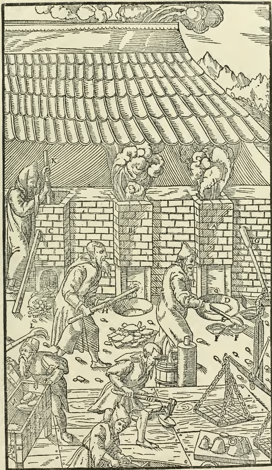
A, B, C—THREE FURNACES. AT THE FIRST STANDS THE SMELTER, WHO WITH A LADLE POURS THE ALLOY OUT OF THE FOREHEARTH INTO THE MOULDS. D—FOREHEARTH. E—LADLE. F—MOULDS. G—ROUND WOODEN RAMMER. H—TAPPING-BAR. AT THE SECOND FURNACE STANDS THE SMELTER, WHO OPENS THE TAP-HOLE WITH HIS TAPPING-BAR. THE ASSISTANT, STANDING ON STEPS PLACED AGAINST THE THIRD FURNACE WHICH HAS BEEN BROKEN OPEN, CHIPS OFF THE ACCRETIONS. I—STEPS. K—SPATULA. L—THE OTHER HOOKED BAR. M—MINE CAPTAIN CARRYING A CAKE, IN WHICH HE HAS STUCK THE PICK, TO THE SCALES TO BE WEIGHED. N—ANOTHER MINE CAPTAIN OPENS A CHEST IN WHICH HIS THINGS ARE KEPT.
