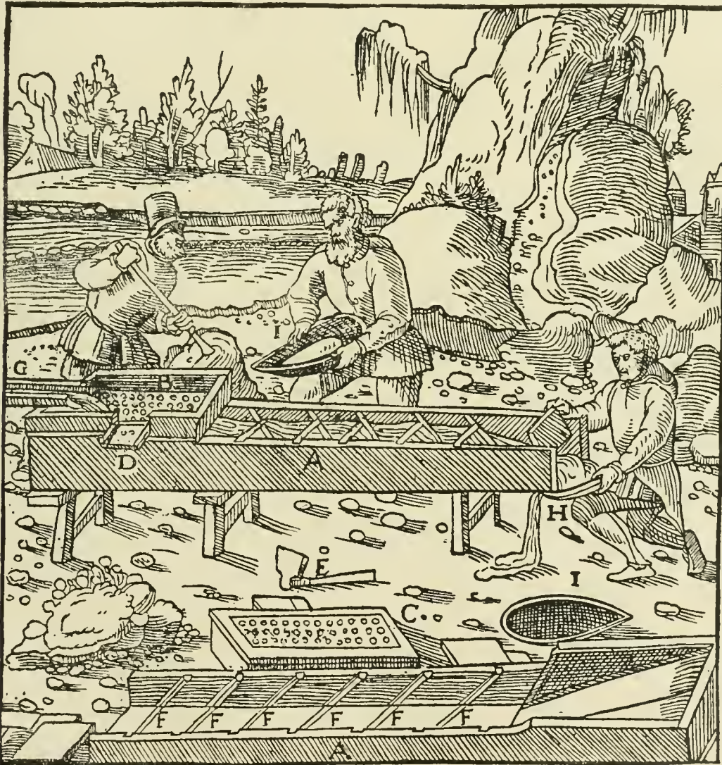
A—SLUICE. B—BOX. C—BOTTOM OF INVERTED BOX. D—OPEN PART OF IT. E—IRON HOE. F—RIFFLES. G—SMALL LAUNDER. H—BOWL WITH WHICH SETTLEMENTS ARE TAKEN AWAY. I—BLACK BOWL IN WHICH THEY ARE WASHED.
