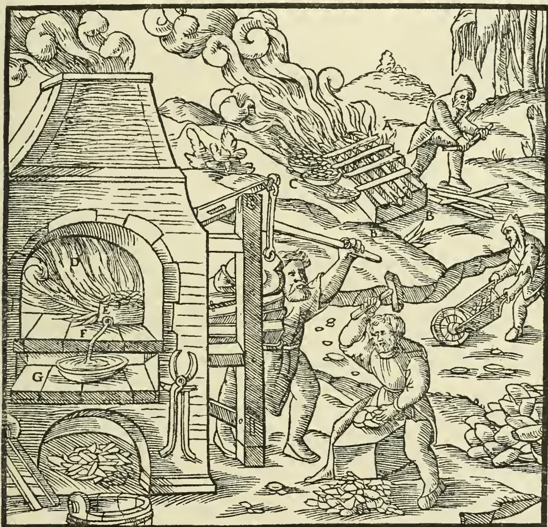
A—WOOD. B—BRICKS. C—PANS. D—FURNACE. E—CRUCIBLE. F—PIPE. G—DIPPING-POT.
