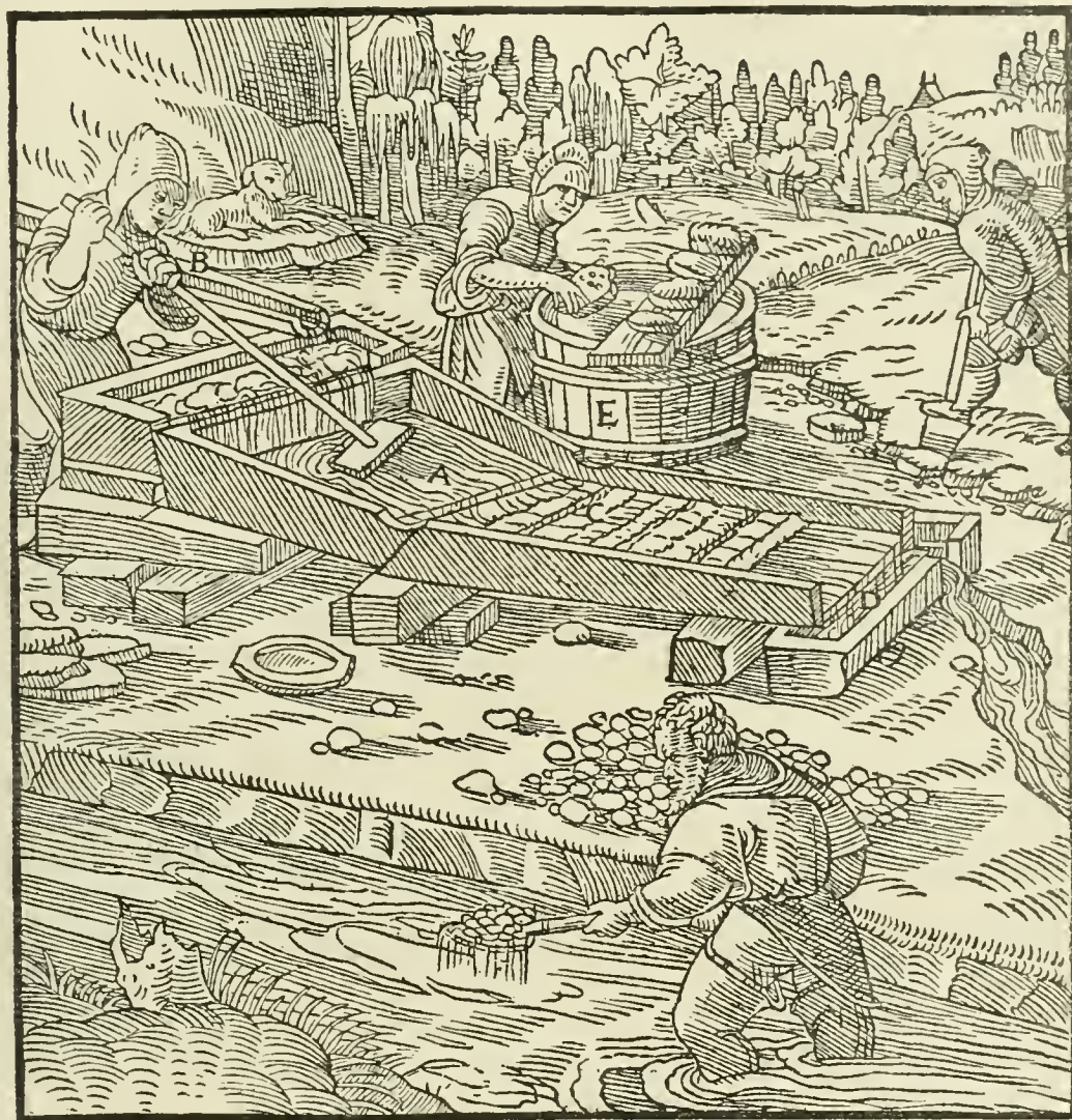
A—HEAD OF FRAME. B—SMALL LAUNDER THROUGH WHICH WATER FLOWS INTO HEAD OF FRAME. C—PIECES OF TURF. D—TROUGH PLACED UNDER FRAME. E—TUB IN WHICH PIECES OF TURF ARE WASHED.
