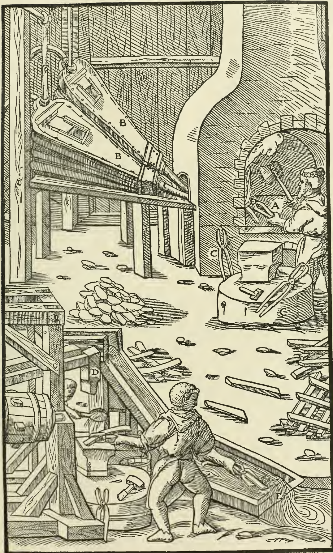
A—FORGE. B—BELLOWS. C—TONGS. D—HAMMER. E—COLD STREAM.
