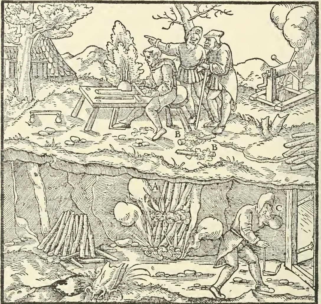
A—KINDLED LOGS. B—STICKS SHAVED DOWN FAN-SHAPED. C—TUNNEL.
