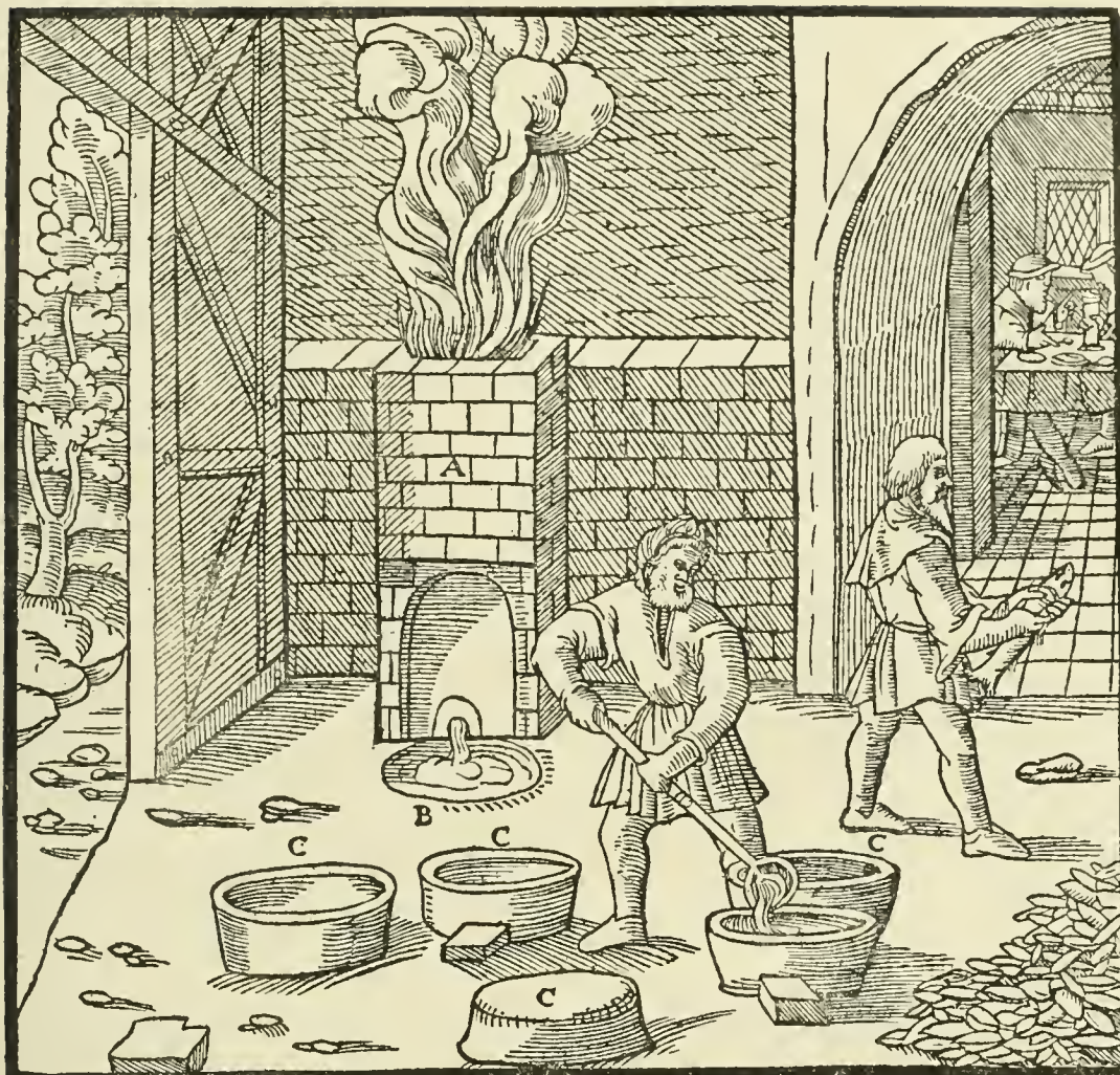
A—FURNACE. B—FOREHEARTH. C—OBLONG MOULDS.
