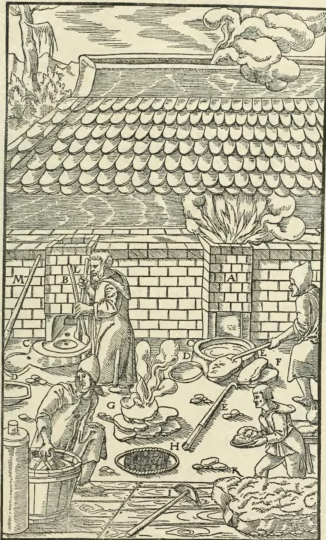
A, B—Two FURNACES. C—FOREHEARTH. D—DIPPING-POT. THE SMELTER STANDING BY THE FIRST FURNACE DRAWS OFF THE SLUGS WITH A HOOKED BAR. E—HOOKED BAR. F—SLUGS. G—THE ASSISTANT DRAWING A BUCKET OF WATER WHICH HE POURS OVER THE GLOWING SLUGS TO QUENCH THEM. H—BASKET MADE OF TWIGS OF WOOD INTERTWINED. I—RABBLE. K—ORE TO BE SMELTED. THE MASTER STANDS AT THE OTHER FURNACE AND PREPARES THE FOREHEARTH BY RAMMING IT WITH TWO RAMMERS. M—CROWBAR.
