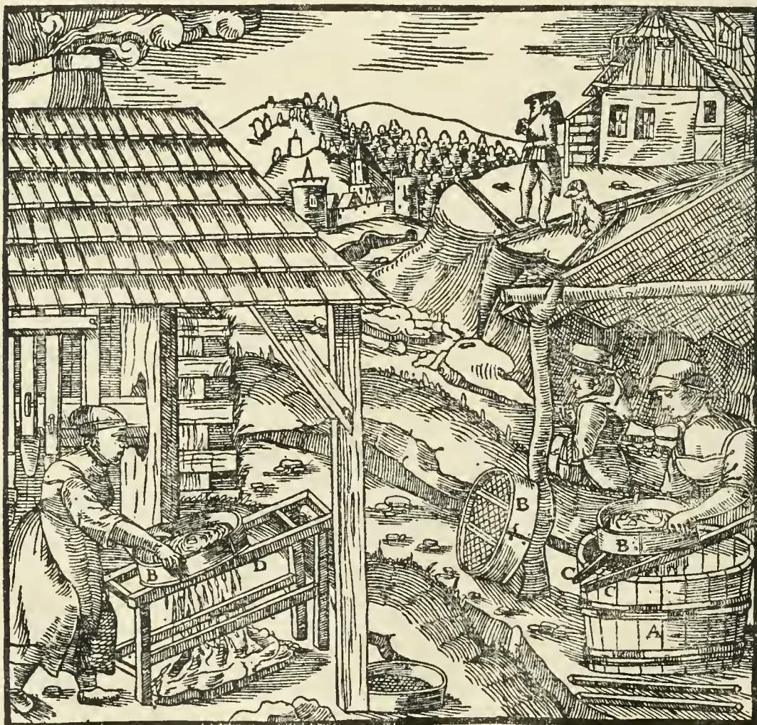
A—TUB. B—SIEVE. C—RODS. D—BENCH-FRAME.
