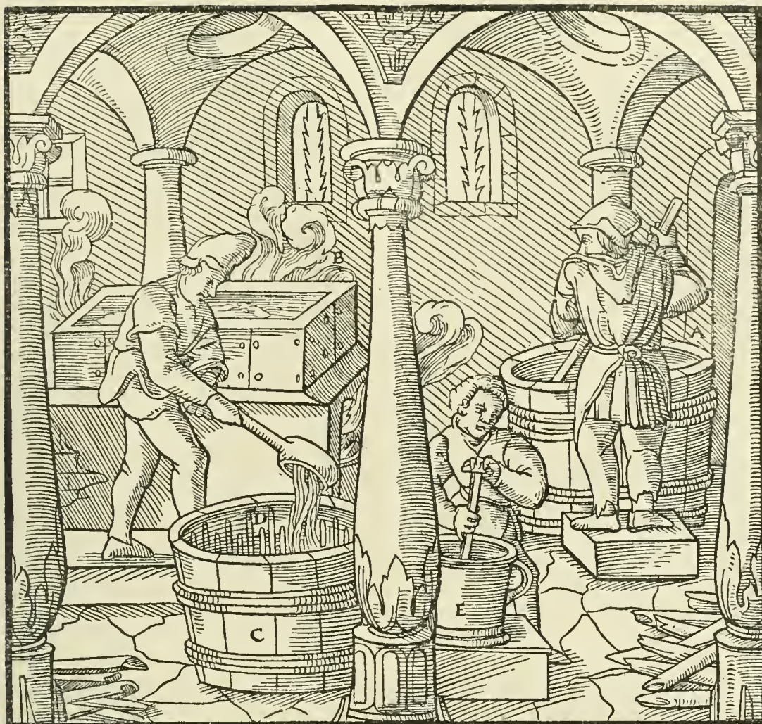
A—VAT IN WHICH THE SODA IS MIXED. B—CALDRON. C—TUB IN WHICH chrysocolia IS CONDENSED. D—COPPER WIRES. E—MORTAR.
