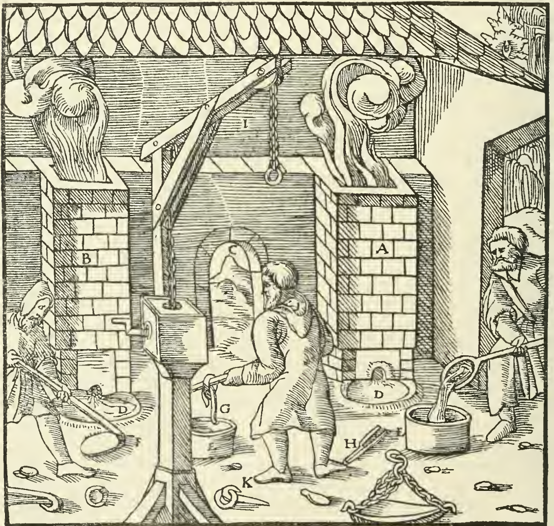
A—FURNACE IN WHICH “SLAGS” ARE RE-SMELTED. B—FURNACE IN WHICH COPPER IS ALLOYED WITH LEAD. C—DOOR. D—FORE-HEARTH ON THE GROUND. E—COPPER MOULDS. F—RABBLE. G—HOOK. H—CLEFT STICK. I—ARM OF THE CRANE. K—THE HOOK OF ITS CHAIN.
