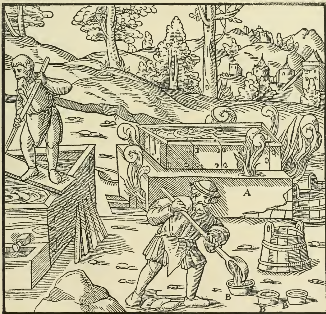
A—CALDRON. B—MOULDS. C—CAKES
