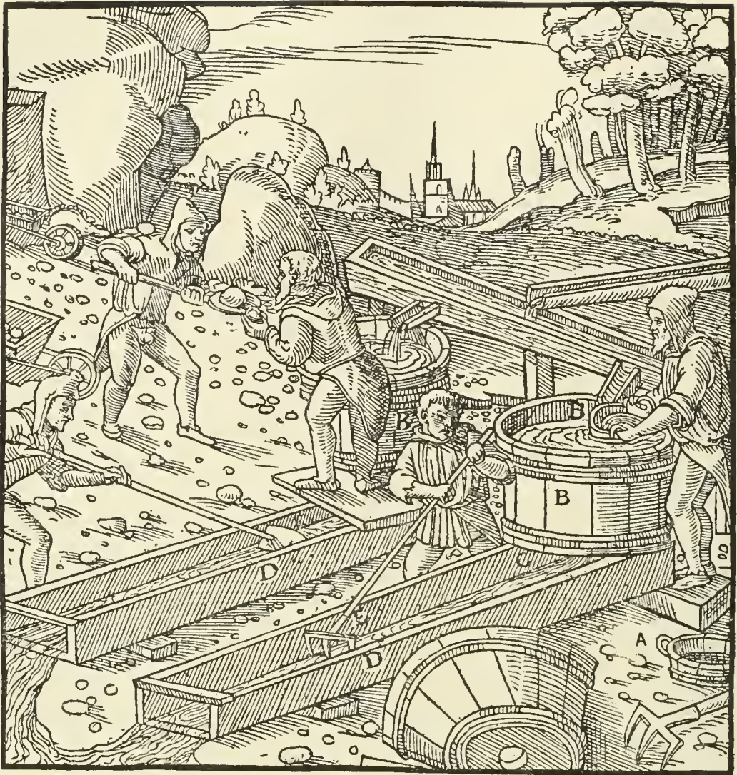
A—SIEVE. B—TUB. C—WATER FLOWING OUT OF THE BOTTOM OF IT. D—STRAKE. E—THREE-TOOTHED RAKE. F—WOODEN SCRUBBER.
