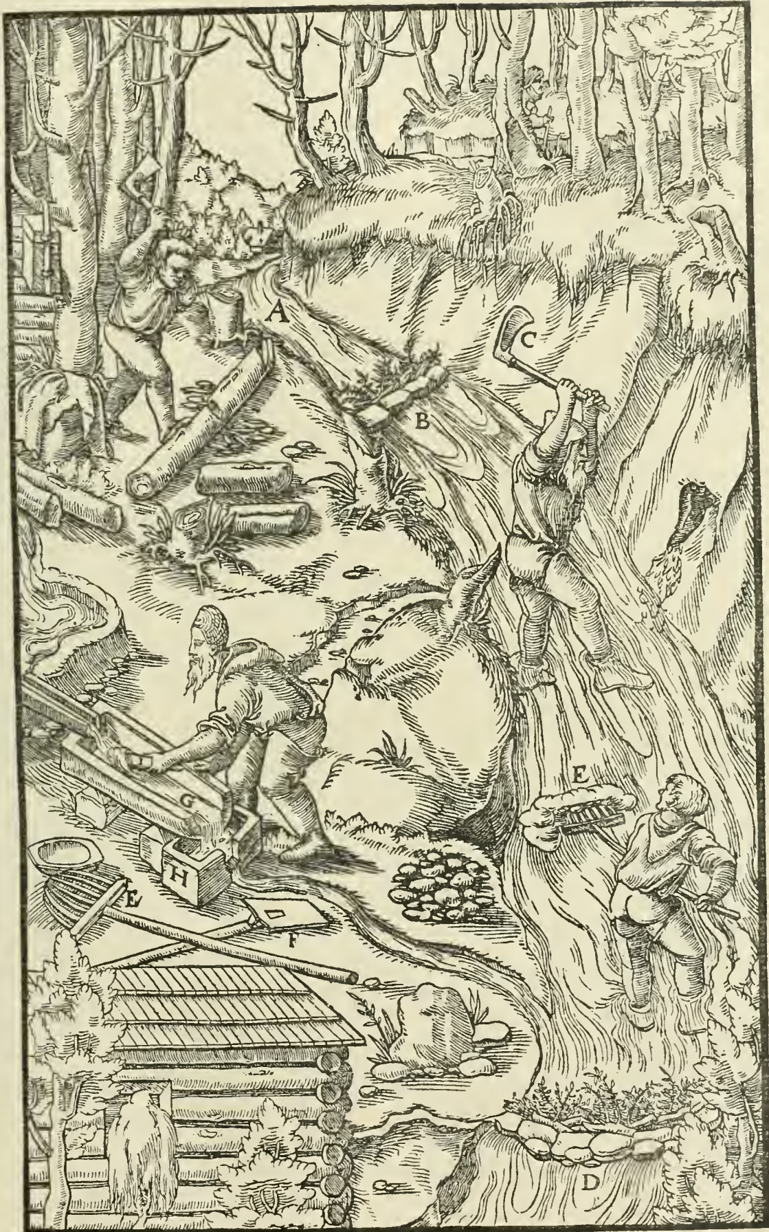
A—STREAM. B—DITCH. C—MATTOCK. D—PIECES OF TURF. E—SEVEN-PRONGED FORK. F—IRON SHOVEL. G—TROUGH. H—ANOTHER TROUGH BELOW IT. I—SMALL WOODEN TROWEL.
