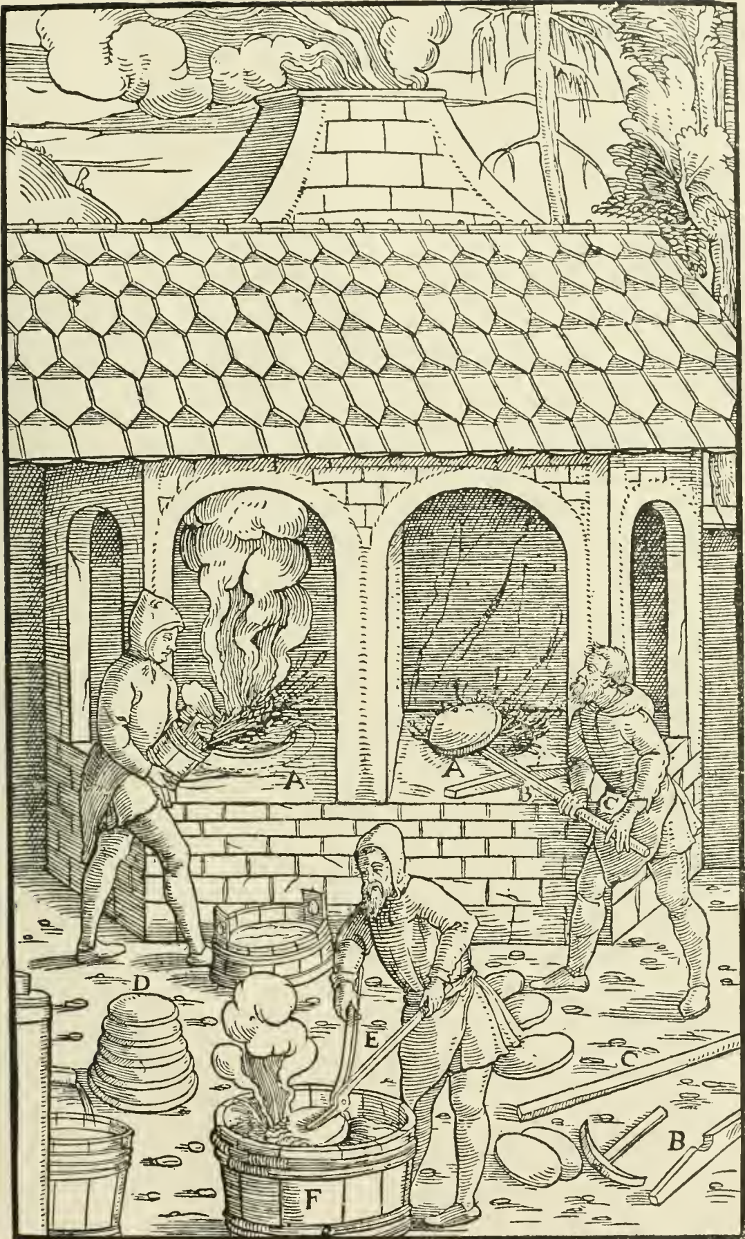
A—CRUCIBLE. B—BOARD. C—WEDGE-SHAPED BAR. D—CAKES OF COPPER MADE BY SEPARATING THEM WITH THE WEDGE-SHAPED BAR. E—TONGS. F—TUB.
