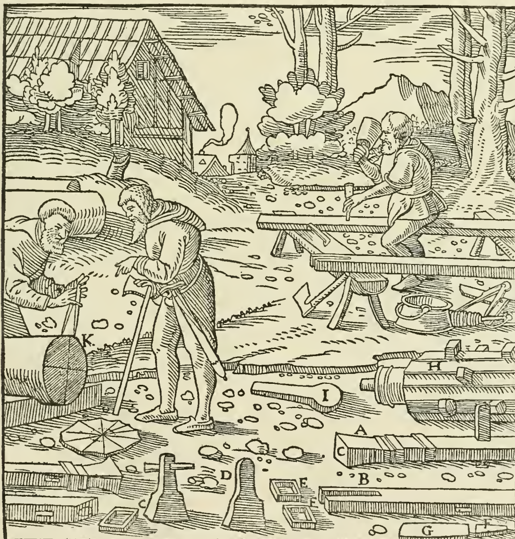
A—STAMP. B—STEM CUT OUT IN LOWER PART. C—SHOE. D—THE OTHER SHOE, BARBED AND GROOVED. E—QUADRANGULAR IRON BAND. F—WEDGE. G—TAPPET. H—ANGULAR CAM-SHAFT. I—CAMS. K—PAIR OF COMPASSES.
