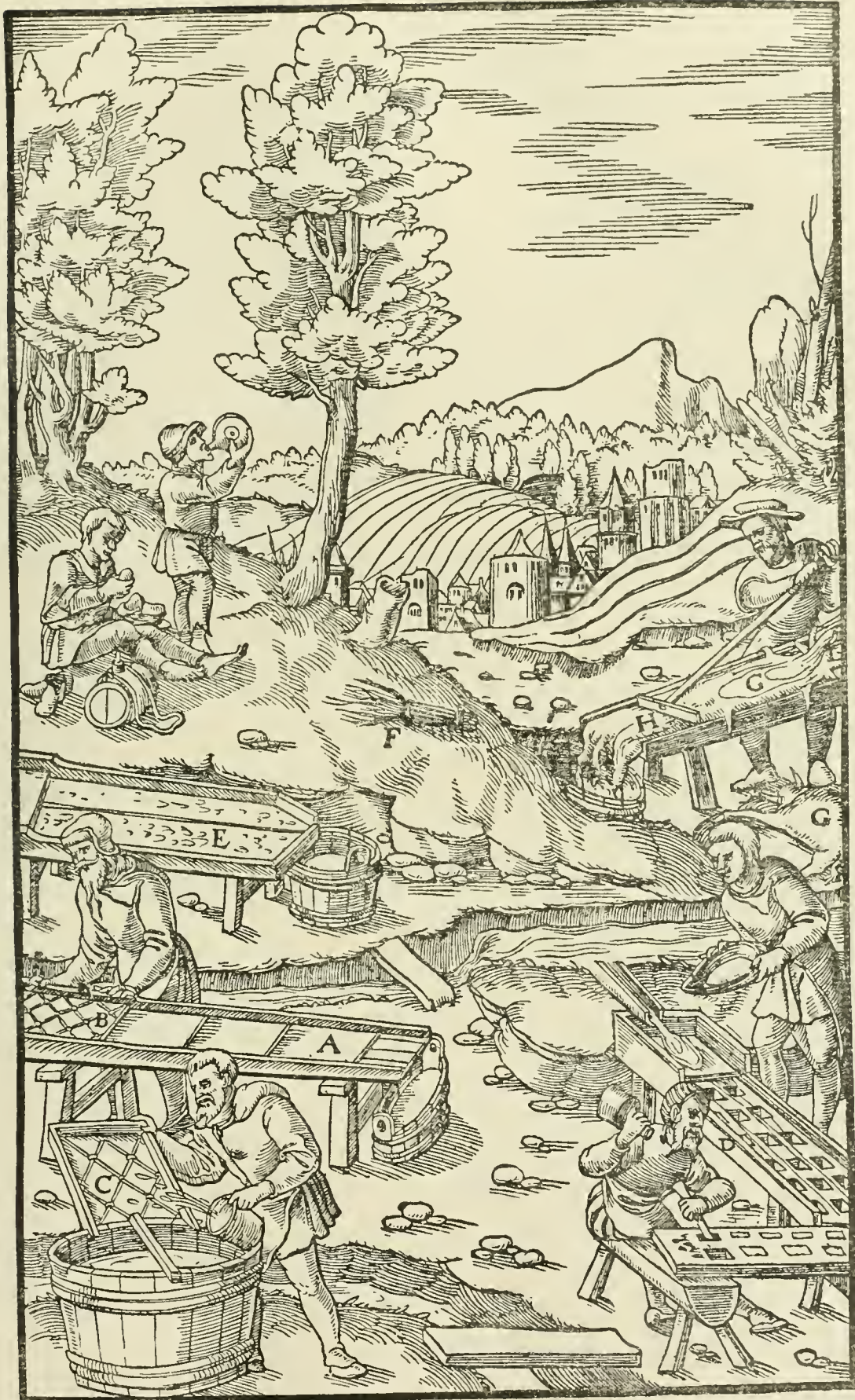
A—SLUICE COVERED WITH CANVAS. B—ITS HEAD FULL OF POCKETS AND GROOVES. C—HEAD REMOVED AND WASHED IN A TUB. D—SLUICE WHICH HAS SQUARE POCKETS. E—SLUICE TO WHOSE PLANKS SMALL SHAVINGS CLING. F—BROOM. G—SKINS OF OXEN. H—WOODEN SCRUBBER.
