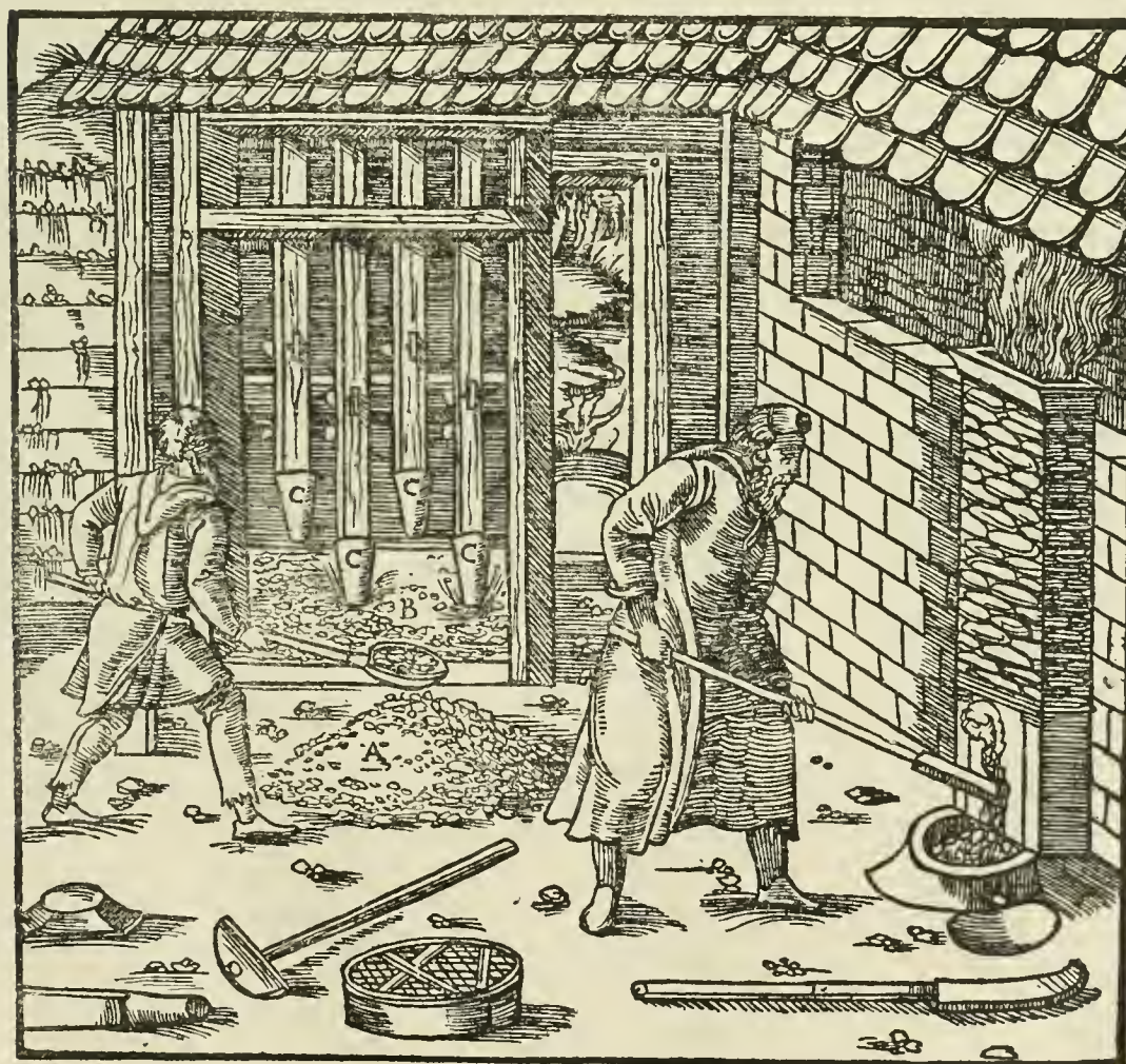
A—CHARCOAL. B—MORTAR-BOX. C—STAMPS.
