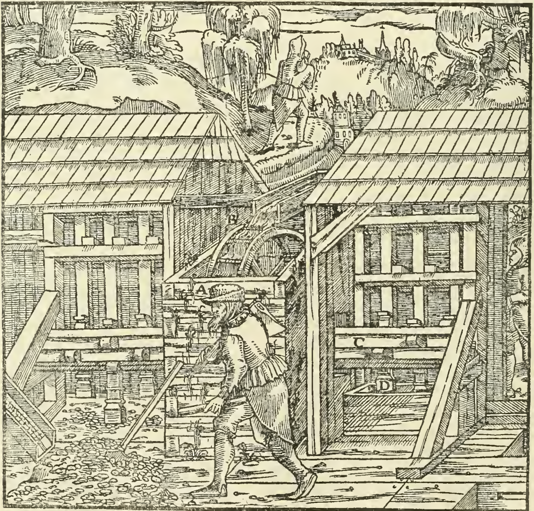
A—Box. ALTHOUGH THE UPPER PART IS NOT OPEN, IT IS SHOWN OPEN HERE, THAT THE WHEEL MAY BE SEEN. B—WHEEL. C—CAM-SHAFT. D—STAMPS.
