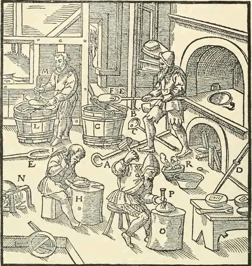
A—IMPLEMENT WITH A RING. B—LADLE. C—ITS HOLE. D—POINTED BAR. E—FORKS. F—CAKE OF SILVER LAID UPON THE IMPLEMENT SHAPED LIKE TONGS. G—TUB OF WATER. H—BLOCK OF WOOD, WITH A CAKE LAID UPON IT. I—HAMMER. K—SILVER AGAIN PLACED UPON THE IMPLEMENT RESEMBLING TONGS. L—ANOTHER TUB FULL OF WATER. M—BRASS WIRES. N—TRIPOD. O—ANOTHER BLOCK. P—CHISEL. Q—CRUCIBLE OF THE FURNACE. R—TEST STILL SMOKING.
