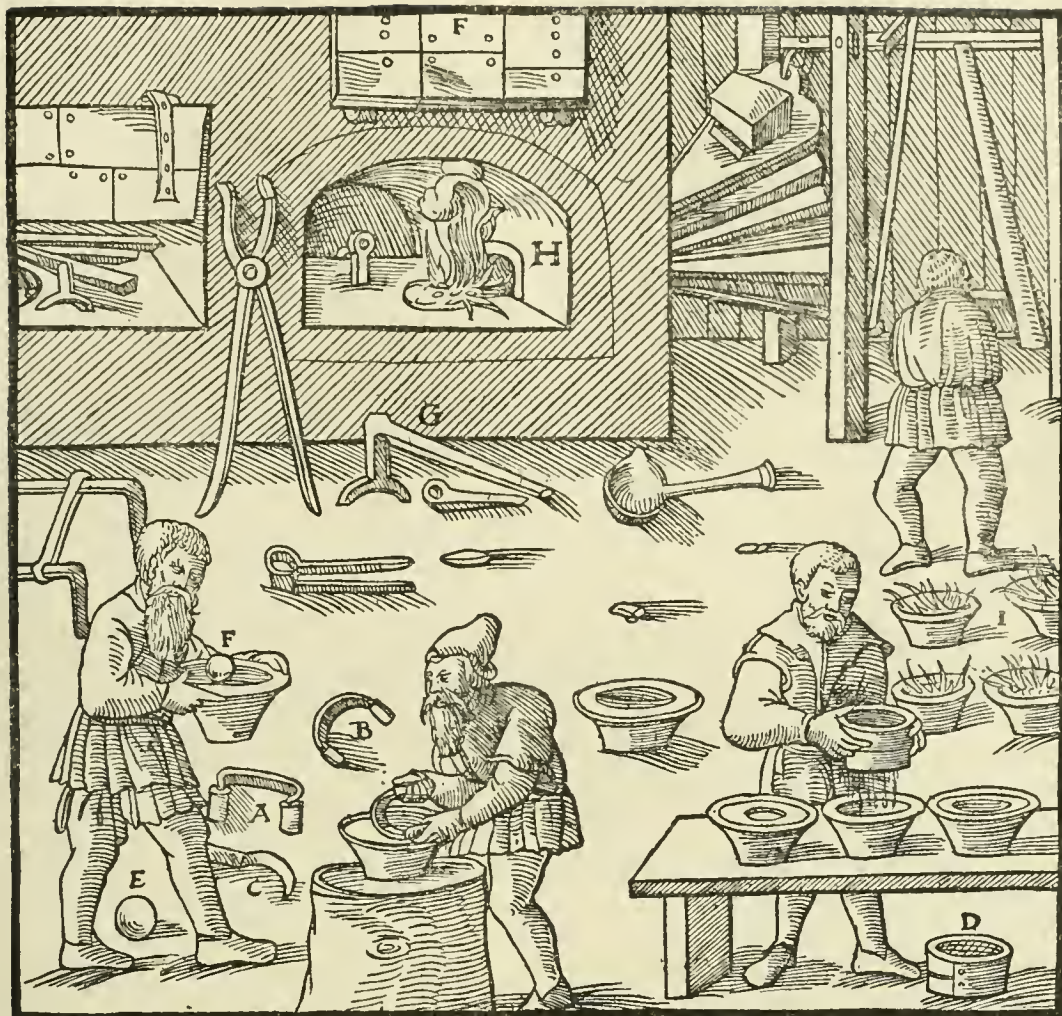
A—STRAIGHT KNIFE HAVING WOODEN HANDLES. B—CURVED KNIFE LIKEWISE HAVING WOODEN HANDLES. C—CURVED KNIFE WITHOUT WOODEN HANDLES. D—SIEVE. E—BALLS. F—IRON DOOR WHICH THE MASTER LETS DOWN WHEN HE REFINES SILVER, LEST THE HEAT OF THE FIRE SHOULD INJURE HIS EYES. G—IRON IMPLEMENT ON WHICH THE WOOD IS PLACED WHEN THE LIQUID SILVER IS TO BE REFINED. H—ITS OTHER PART PASSING THROUGH THE RING OF ANOTHER IRON IMPLEMENT ENCLOSED IN THE WALL OF THE FURNACE. I—TESTS IN WHICH BURNING CHARCOAL HAS BEEN THROWN.
