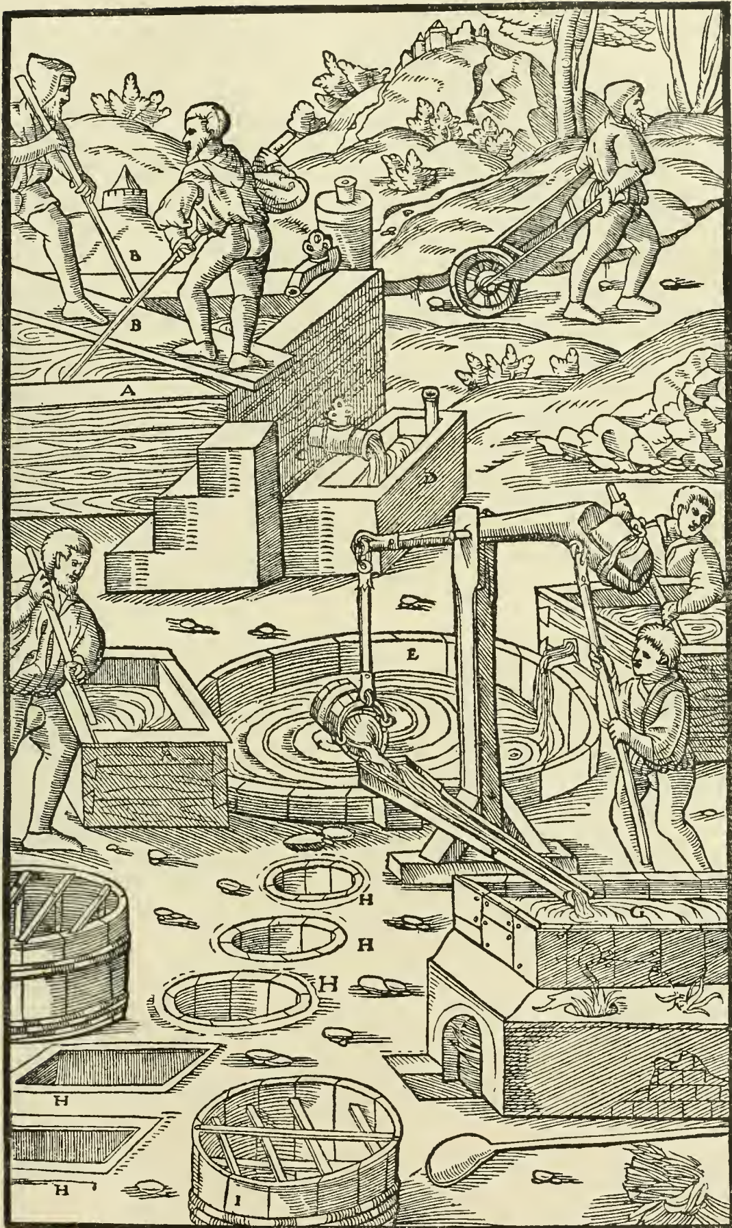
A—TANKS. B—STIRRING POLES. C—PLUG. D—TROUGH. E—RESERVOIR. F—LAUNDER. G—LEAD CALDRON. H—WOODEN TUBS SUNK INTO THE EARTH. I—VATS IN WHICH TWIGS ARE FIXED.
