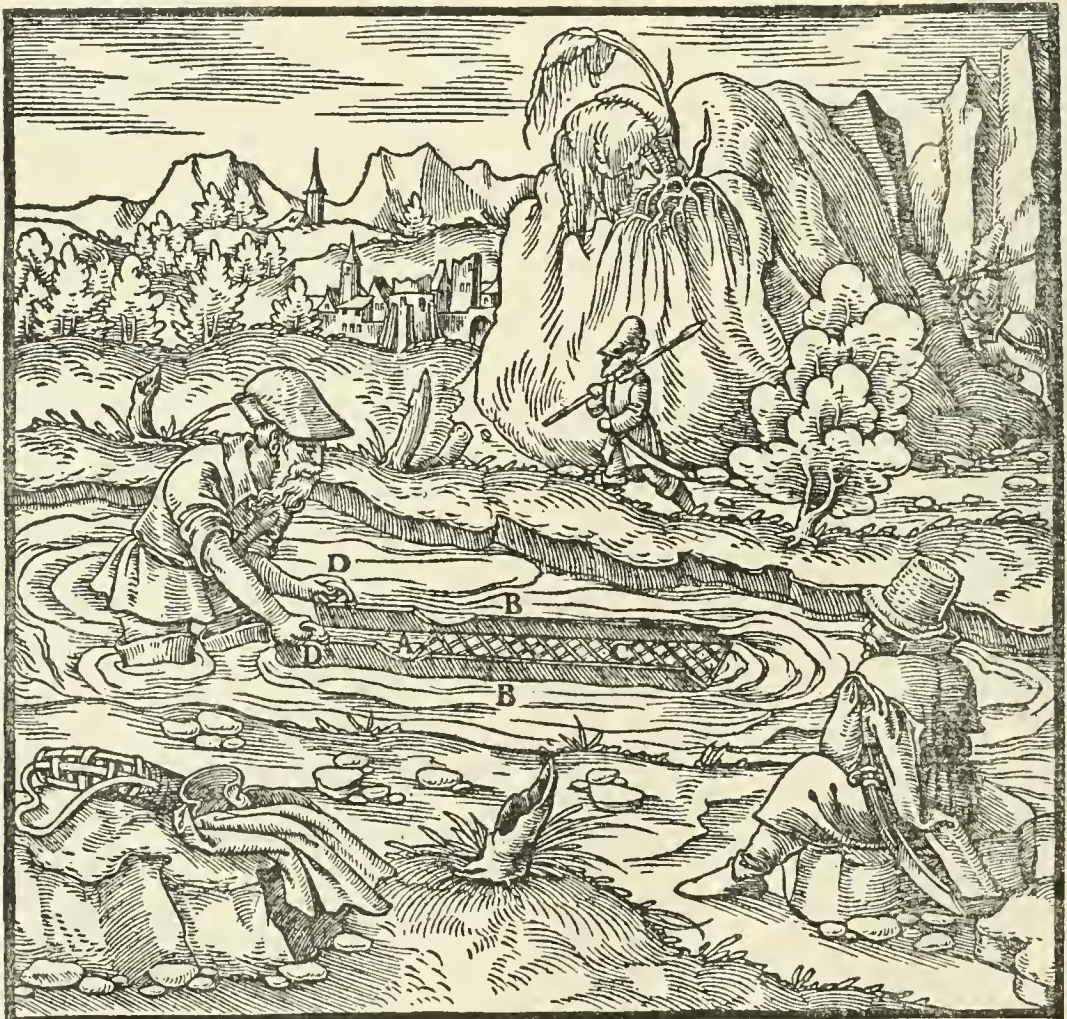
A—PLANK. B—SIDE-BOARDS. C—IRON WIRE. D—HANDLES.
