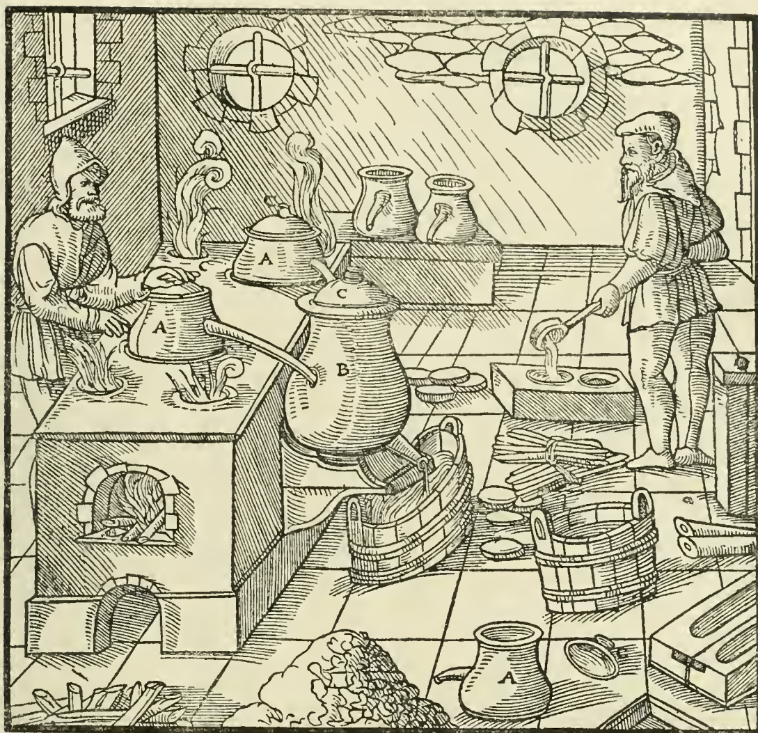
A—POTS HAVING SPOUTS. B—POTS WITHOUT SPOUTS. C—LIDS.
