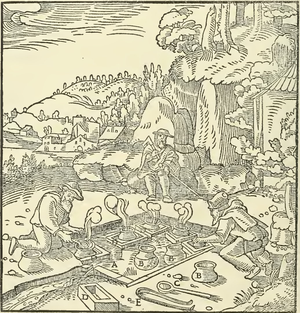
A—POOL. B—POTS. C—LADLE. D—PANS. E—TONGS.
