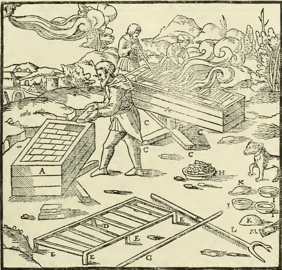
A—Box. B—PIVOT. C—TRANSVERSE WOOD BEAMS. D—GRATE. E—ITS FEET. F—BURNING WOOD. G—STICK. H—PANS IN WHICH THE BISMUTH IS MELTED. I—PANS FOR MOULDS. K—CAKES. L—FORK. M—BRUSH.
