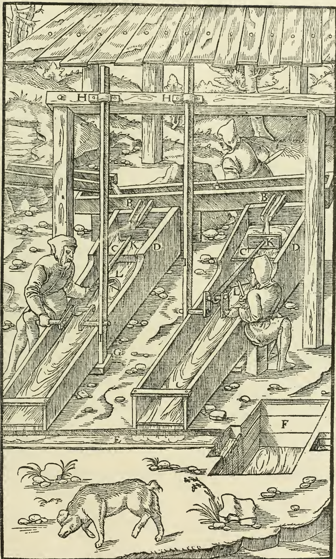
A—UPPER CROSS LAUNDER. B—SMALL LAUNDERS. C—HEADS OF STRAKES. D—STRAKES. E—LOWER TRANSVERSE LAUNDER. F—SETTLING PIT. G—SOCKET IN THE SILL. H—HALVED IRON RINGS FIXED TO BEAM. I—POLE. K—ITS LITTLE SCRUBBER. L—SECOND SMALL SCRUBBER.
