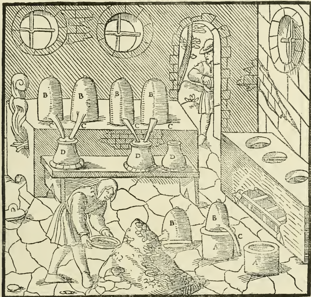
A—POTS. B—OPERCULA. C—NOZZLES. D—GOURD-SHAPED EARTHENWARE VESSELS.
