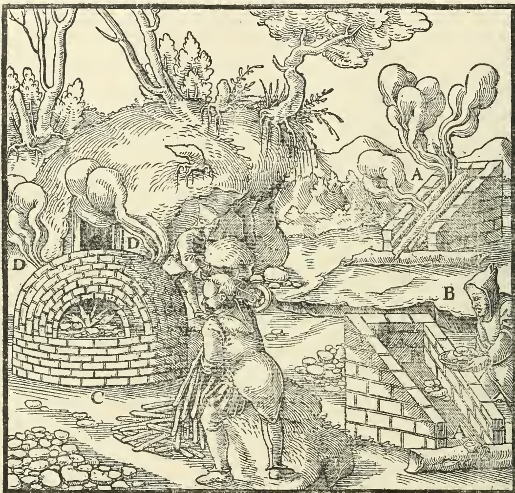
A—BURNING PYRE WHICH IS COMPOSED OF LEAD ORE WITH WOOD PLACED ABOVE IT. B—WORKMAN THROWING ORE INTO ANOTHER AREA. C—OVEN-SHAPED FURNACE. D—OPENINGS THROUGH WHICH THE SMOKE ESCAPES.
