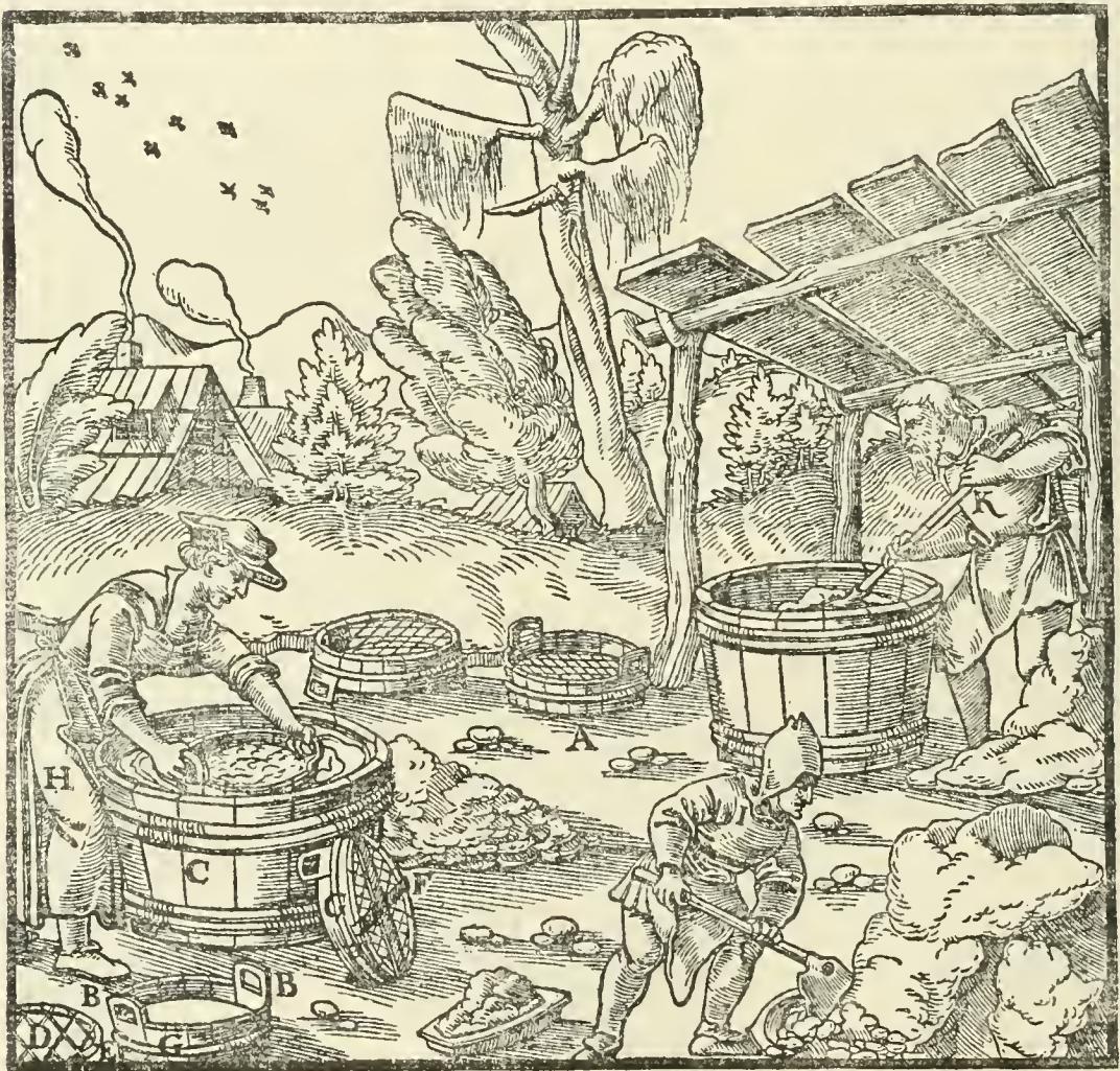
A—SIEVE. B—ITS HANDLES. C—TUB. D—BOTTOM OF SIEVE MADE OF IRON WIRES. E—HOOP. F—RODS. G—HOOPS. H—WOMAN SHAKING THE SIEVE. I—BOY SUPPLYING IT WITH MATERIAL WHICH REQUIRES WASHING. K—MAN WITH SHOVEL REMOVING FROM THE TUB THE MATERIAL WHICH HAS PASSED THROUGH THE SIEVE.
