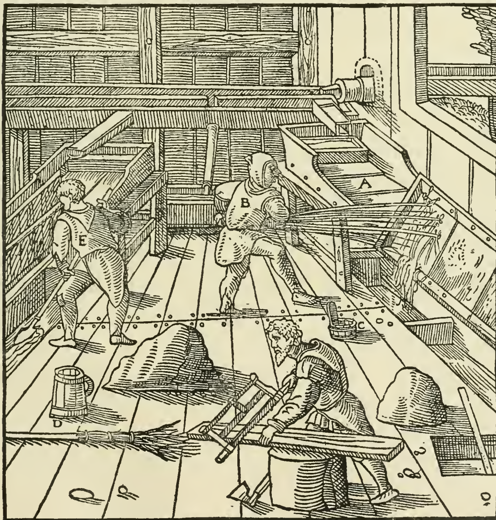
A—CANVAS STRAKE. B—MAN DASHING WATER ON THE CANVAS. C—BUCKET. D—BUCKET OF ANOTHER KIND. E—MAN REMOVING CONCENTRATES OR TIN-STONE FROM THE TROUGH.
