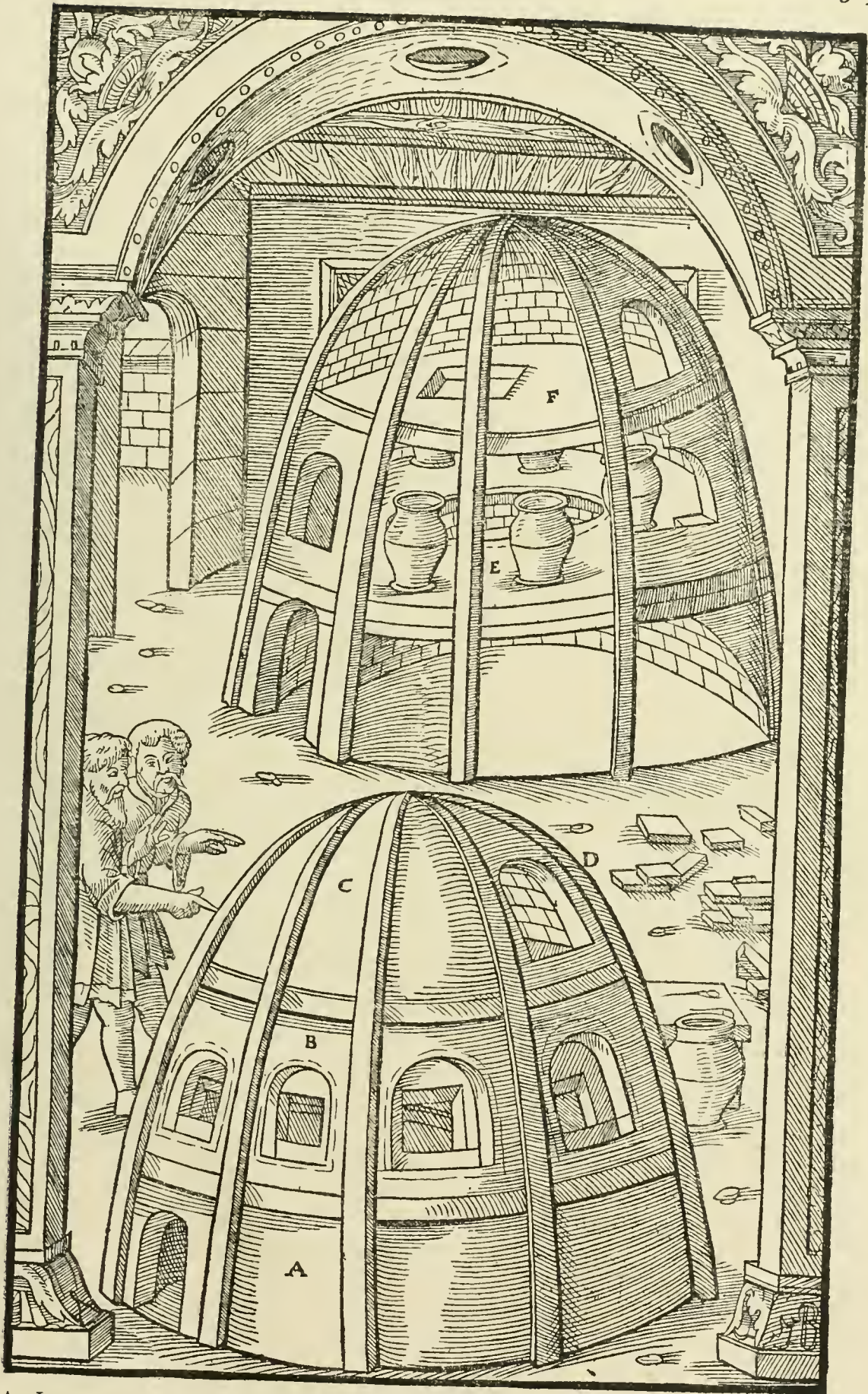
A—LOWER CHAMBER OF THE OTHER SECOND FURNACE. B—MIDDLE ONE. C—UPPER ONE. D—ITS OPENING. E—ROUND OPENING. F—RECTANGULAR OPENING.
