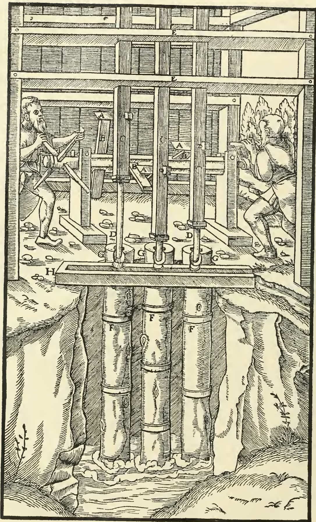
A—TAPPETS OF PISTON-RODS. B—CAMS OF THE BARREL. C—SQUARE UPPER PARTS OF PISTON-RODS. D—LOWER ROUNDED PARTS OF PISTON-RODS. E—CROSS-BEAMS. F—PIPES. G—APERTURES OF PIPES. H—TROUGH. (Fifth kind of pump—see p. 181).
