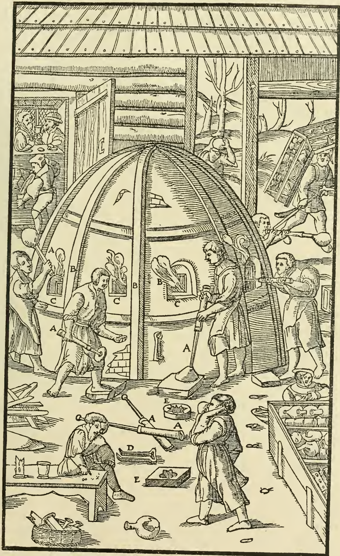
A—BLOW-PIPE. B—LITTLE WINDOW. C—MARBLE. D—FORCEPS. E—MOULDS BY MEANS OF WHICH THE SHAPES ARE PRODUCED.
