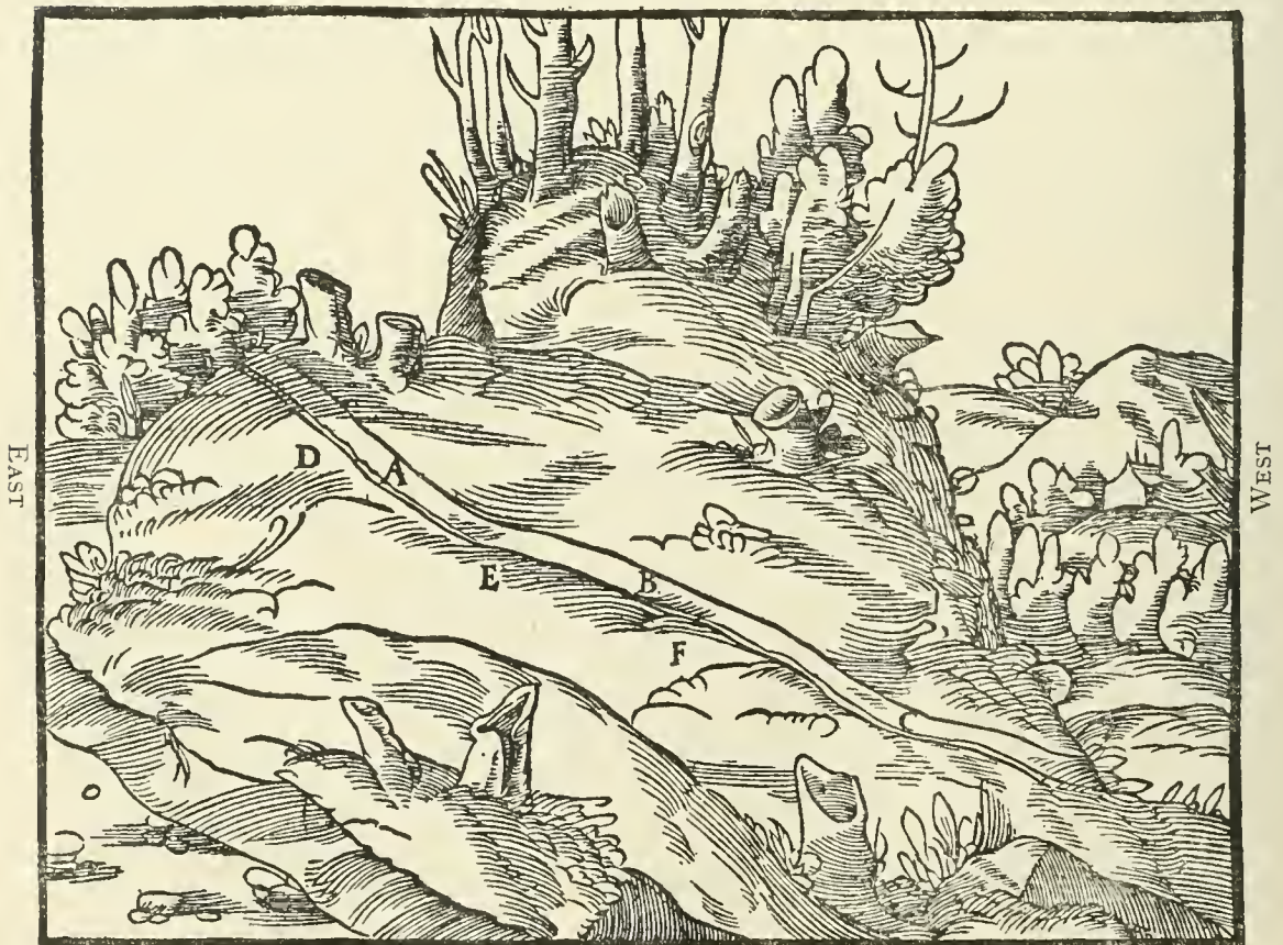
A, B, C—VEIN. D, E, F—SEAMS IN THE ROCK ( Commissurae Saxorum ). NORTH
