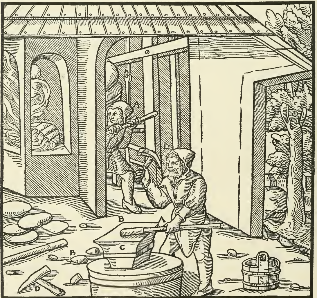
A—POINTED BAR. B—THIN COPPER LAYER. C—ANVIL. D—HAMMER.
