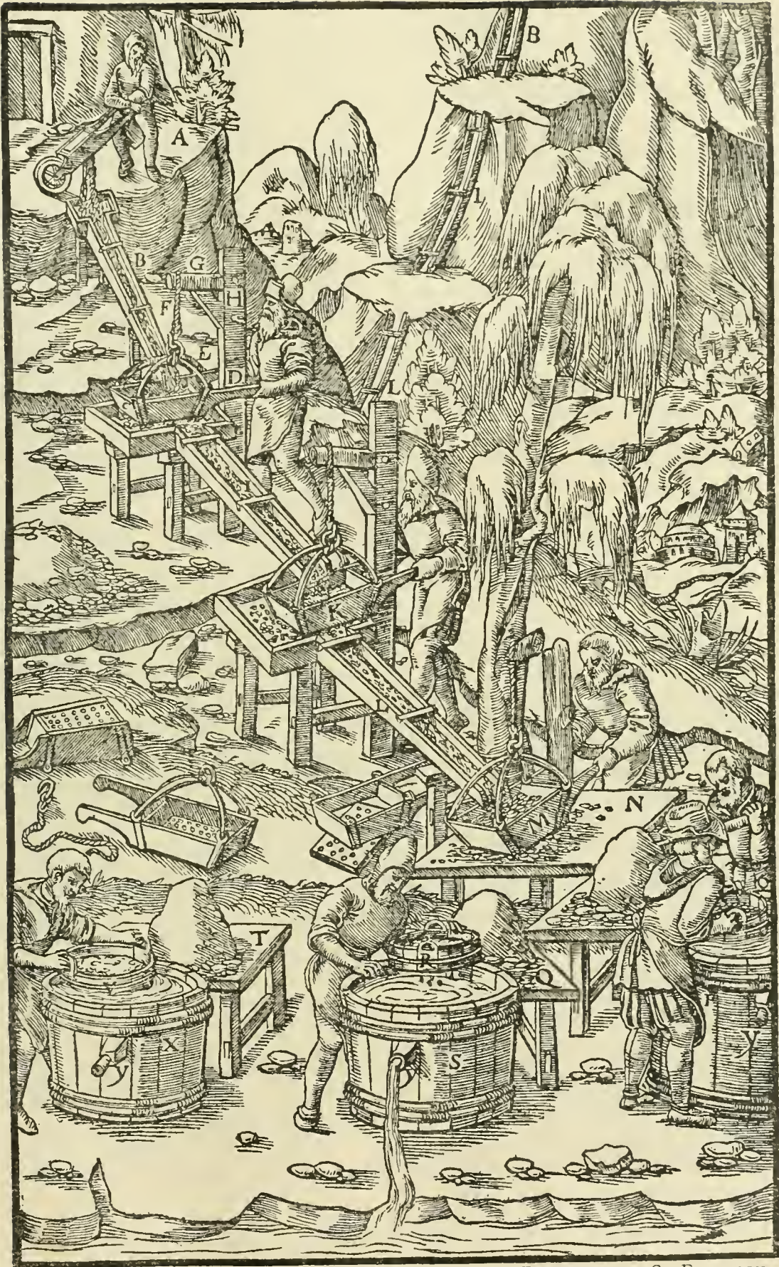
A—WORKMAN CARRYING BROKEN ROCK IN A BARROW. B—FIRST CHUTE. C—FIRST BOX. D—ITS HANDLES. E—ITS BALES. F—ROPE. G—BEAM. H—POST. I—SECOND CHUTE. K—SECOND BOX. L—THIRD CHUTE. M—THIRD BOX. N—FIRST TABLE. O—FIRST SIEVE. P—FIRST TUB. Q—SECOND TABLE. R—SECOND SIEVE. S—SECOND TUB. T—THIRD TABLE. V—THIRD SIEVE. X—THIRD TUB. Y—PLUGS.
