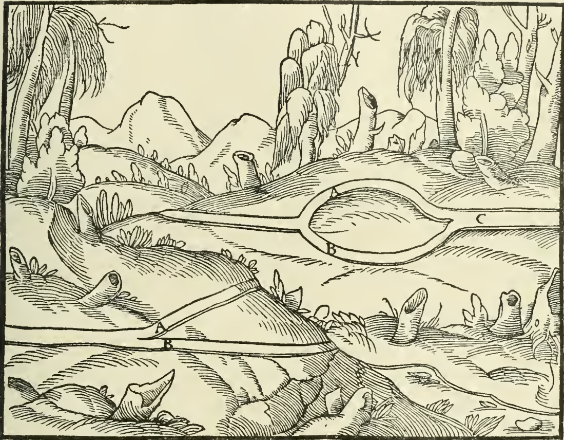
A, B—VEINS DIVIDING. C—THE SAME JOINING.
