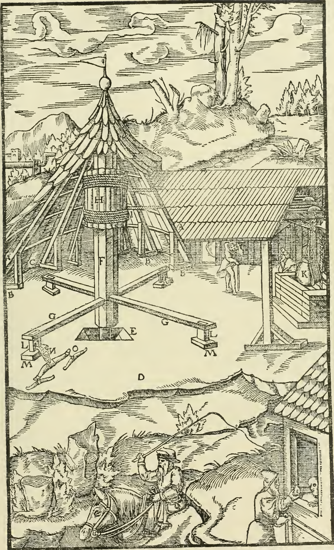
A—UPRIGHT BEAMS. B—SILLS LAID FLAT UPON THE GROUND. C—POSTS. D—AREA. E—SILL SET AT THE BOTTOM OF THE HOLE. F—AXLE. G—DOUBLE CROSS-BEAMS. H—DRUM. I—WINDING-ROPE. K—BUCKET. L—SMALL PIECES OF WOOD HANGING FROM DOUBLE CROSS-BEAMS. M—SHORT WOODEN BLOCK. N—CHAIN. O—POLE BAR. P—GRAPPLING HOOK. (Some members mentioned in the text are not shown).
