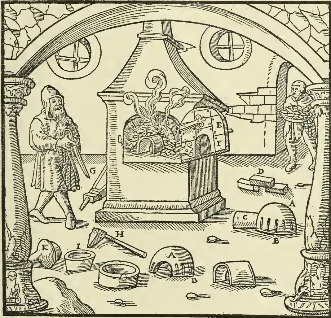
A—MUFFLE. B—ITS LITTLE WINDOWS. C—ITS LITTLE BRIDGE. D—BRICKS. E—IRON DOOR. F—ITS LITTLE WINDOW. G—BELLOWS. H—HAMMER-CHISEL. I—IRON RING WHICH SOME USE INSTEAD OF THE TEST. K—PESTLE WITH WHICH THE ASHES PLACED IN THE RING ARE POUNDED.
