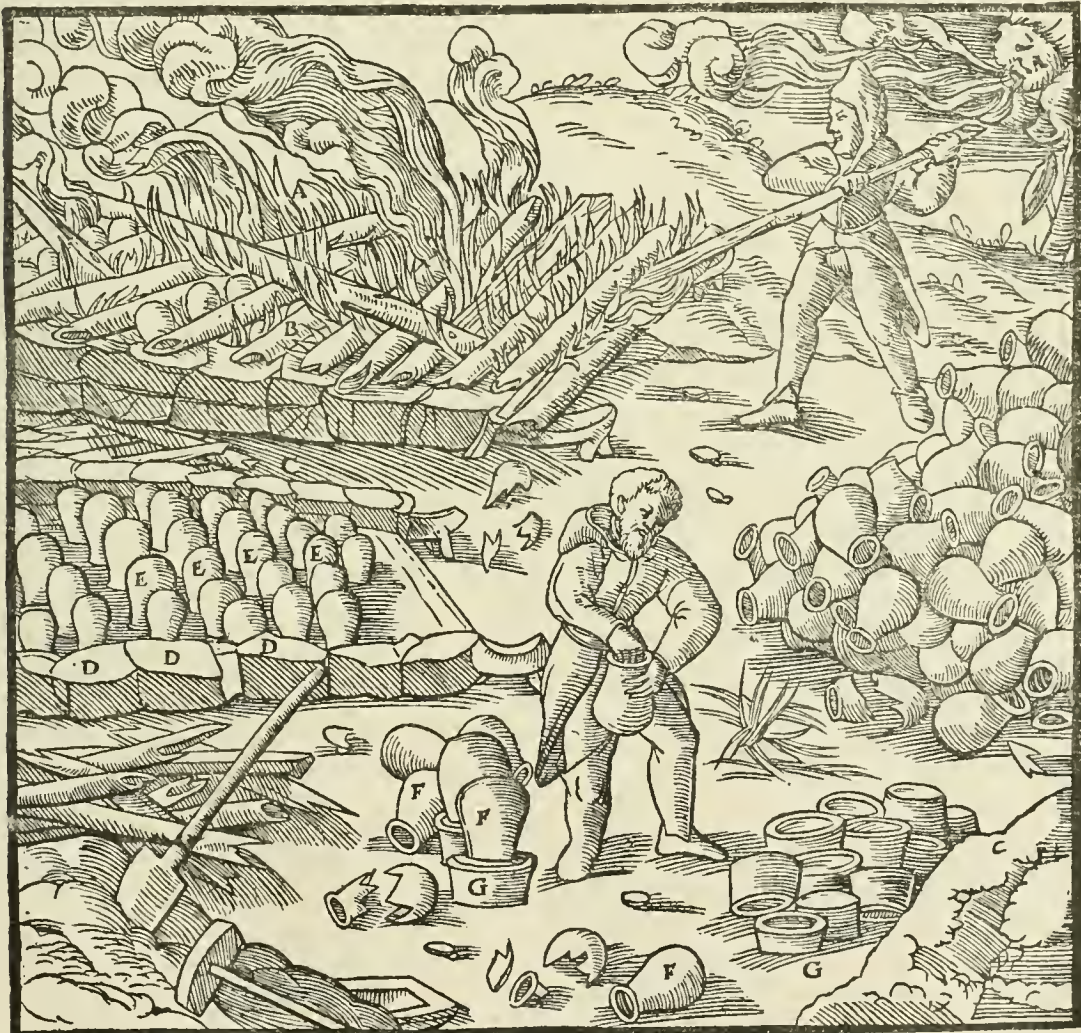
A—HEARTH. B—POLES. C—HEARTH WITHOUT FIRE IN WHICH THE POTS ARE PLACED. D—ROCKS. E—ROWS OF POTS. F—UPPER POTS. G—LOWER POTS.
