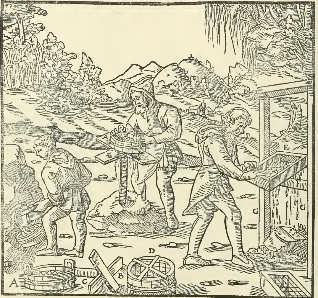
A—SIEVE. B—SMALL PLANKS. C—POST. D—BOTTOM OF SIEVE. E—OPEN BOX. F—SMALL CROSS-BEAM. G—UPRIGHT POSTS.
