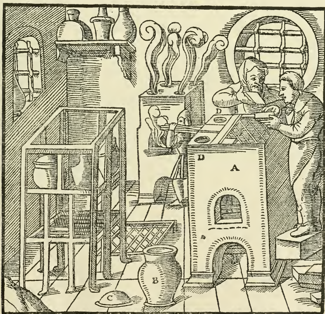
A—FURNACE. B—POT. C—LID. D—AIR-HOLES.
