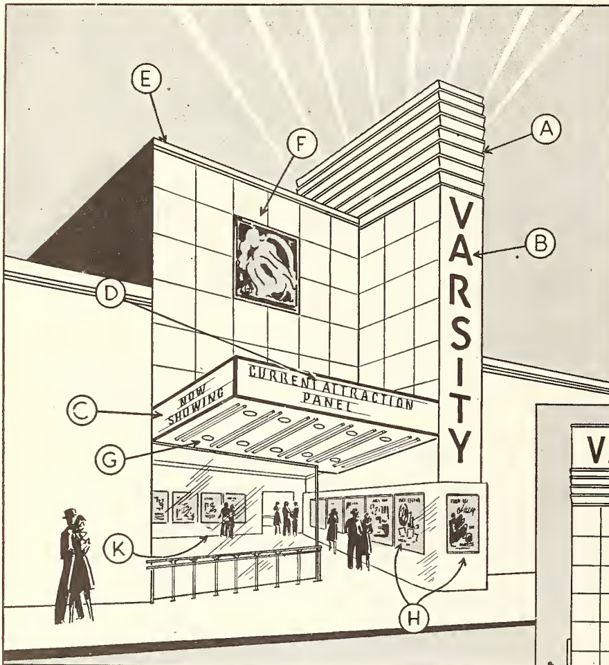
FIGURE 5: Architectural and promotional lighting for the Front.
