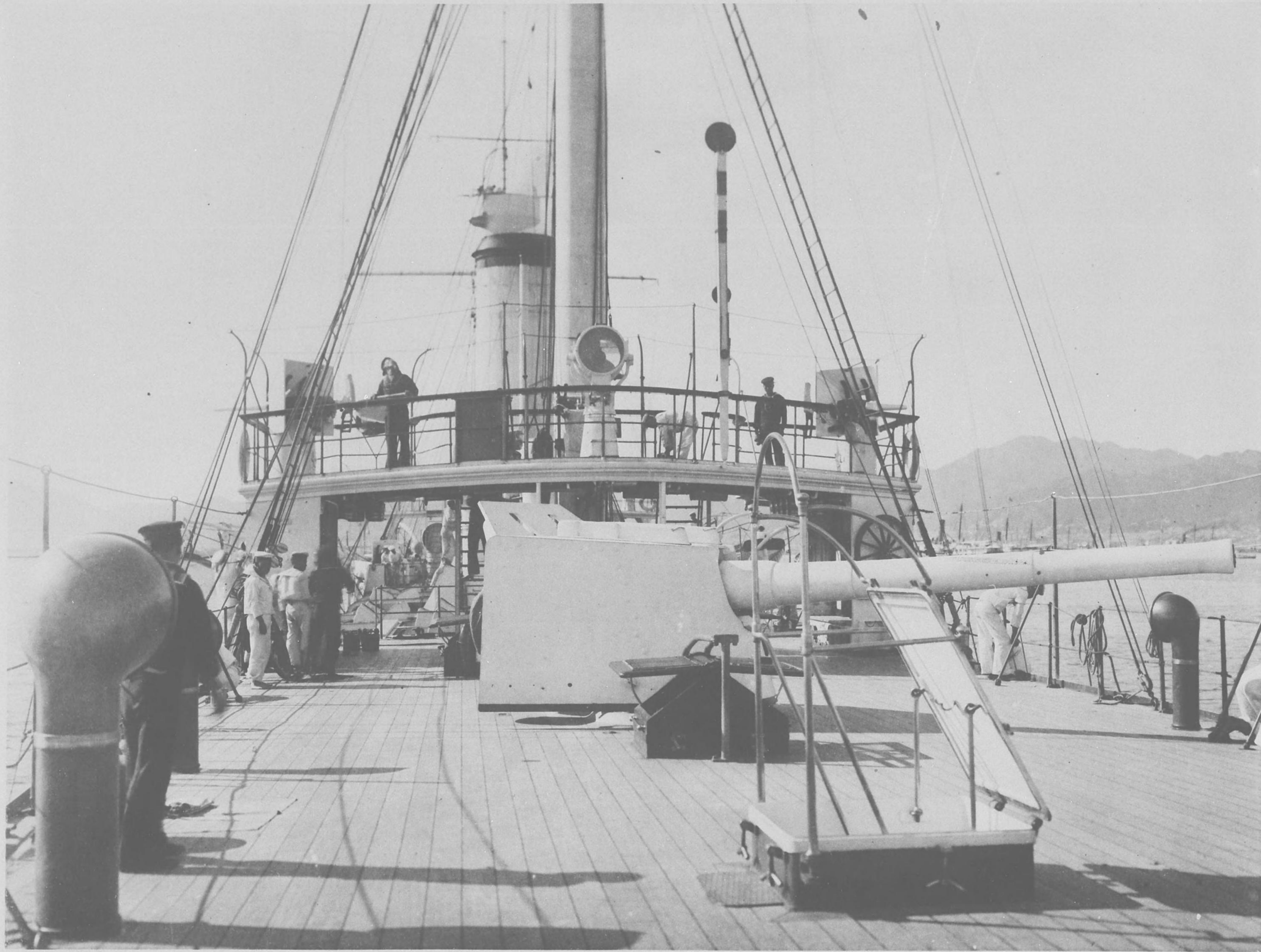
砲射速珊五十式安磨須艦軍 The 6-in Armstrong quick firing gun of "Suma."
