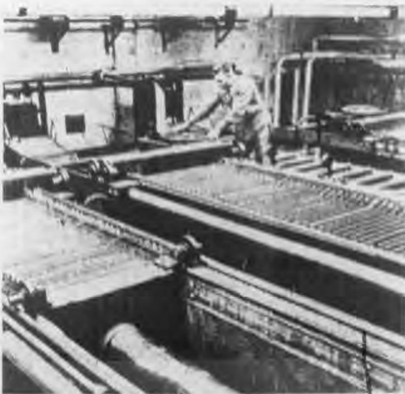
After its first chemical bath the cellulose is introduced into these huge drying presses. Later it is mashed and begins its way through a number of chemical solutions.
