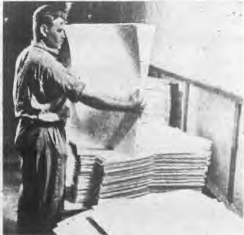
Cellulose cards are shuffled. Cards from different shipments are well mixed in order to assure uniformity in the production of artificial silk.
