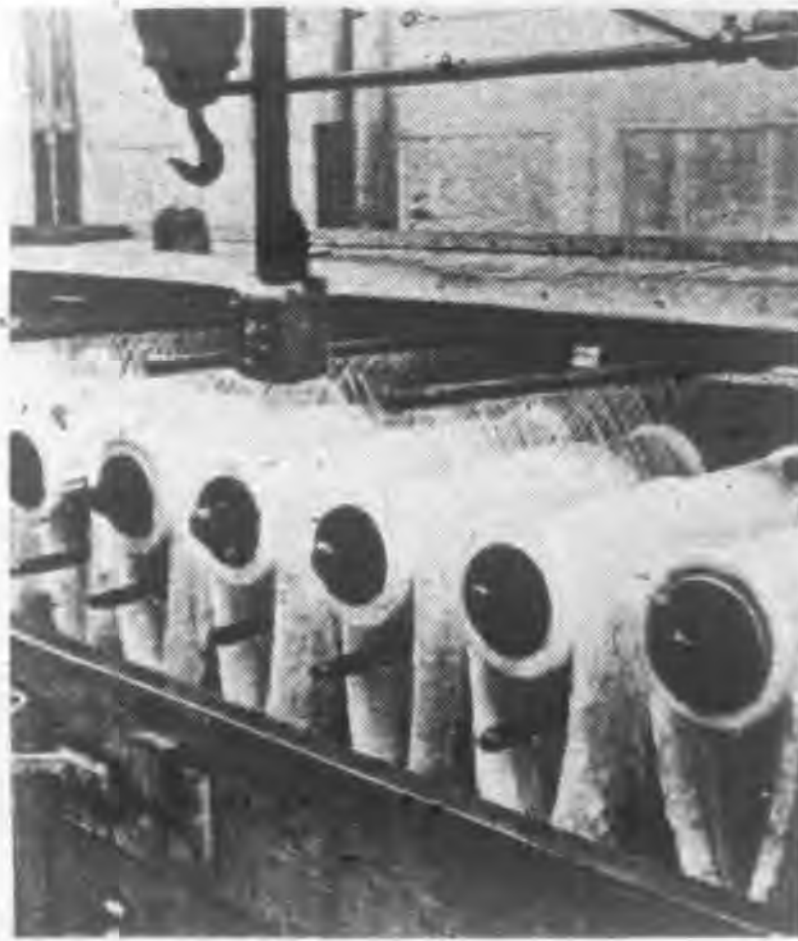
○機持絲人吹白，洗 器種之造乾，漂潔 This special machine washes, bleaches and dries the silk. The manufacturing process is nearly completed.
