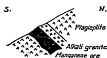
Fig. 5. Section south of Heitzeitzu, showing the contact of alkali granite with manganese ore.
