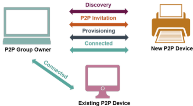
Figure 10. Adding a Device to P2P Group by Invitation. Source: Wi-Fi Alliance (n.d.).
