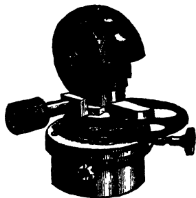
FIG. 111 — Beck's New Achromatic Condenser.
