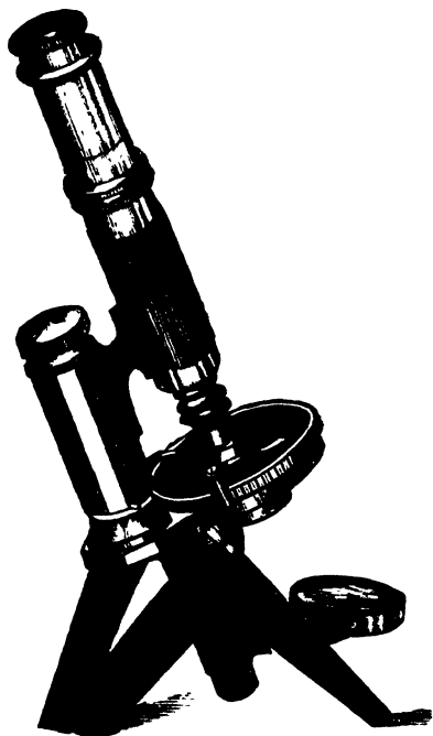
FIG 53 — Baker's Model Histological Microscope.
