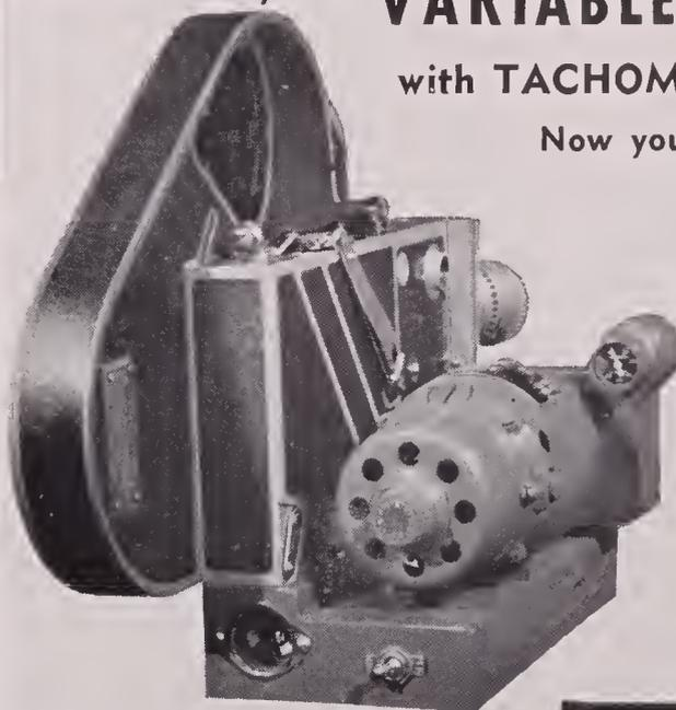
Tachometer is mounted in clear view of operator. It is calibrated from 16 frames per second to 64 fps. with a definite RED marking for 24 fps. Electrical governor control for adjusting speeds. Steady operation at ALL speeds. "OFF-ON" switch built into motor base. No adaptors required, except motor coupling which attaches to camera and couples to motor.
