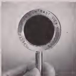
This 2% density optical viewing glass, shows the highlight and shadow details of scenes exactly as reproduced on color film. Changes in illumination of subjects to be photographed may be made as indicated by the use of this viewing glass.
