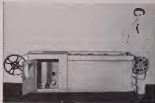
heating elements and neoprene lined steel tanks of two-gallon capacity.
