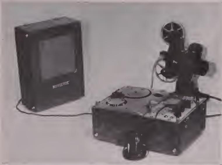
Movievox recorder synchronized with Bell & Howell 8mm. projector. Synchronism is maintained through flexible shaft connecting both machines, each operating under own power.
