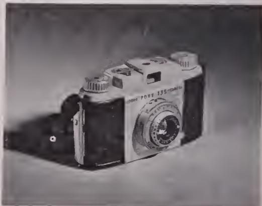
51mm., f/4.5. Lens diaphragm control can be stopped down to f/22. Cocking type shutter provides speeds of 1/25, 1/50, 1/100, 1/200, and "B" for time exposures. It sells for \$34.50.
