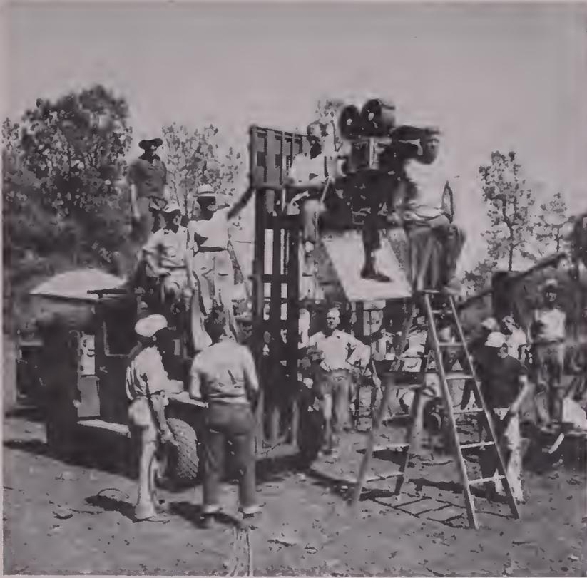
NEW MOTORIZED hydraulic "uplift" camera car is combination 4-wheel-drive army truck and freight-loading fork lift, makes possible use of blimped Technicolor camera in the most rugged of locations, and permits use of camera from ground level to height of fifteen feet.
