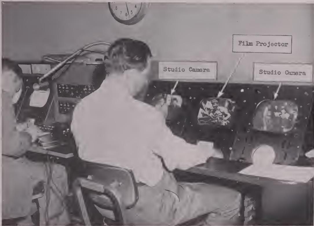
IT'S A SIMPLE MATTER for the television engineer to mix motion pictures with live action at the monitor console and make it appear that both actions originate at the same source. Here an exterior scene, filmed especially for the program, is intercut between action picked up by two studio television cameras.
