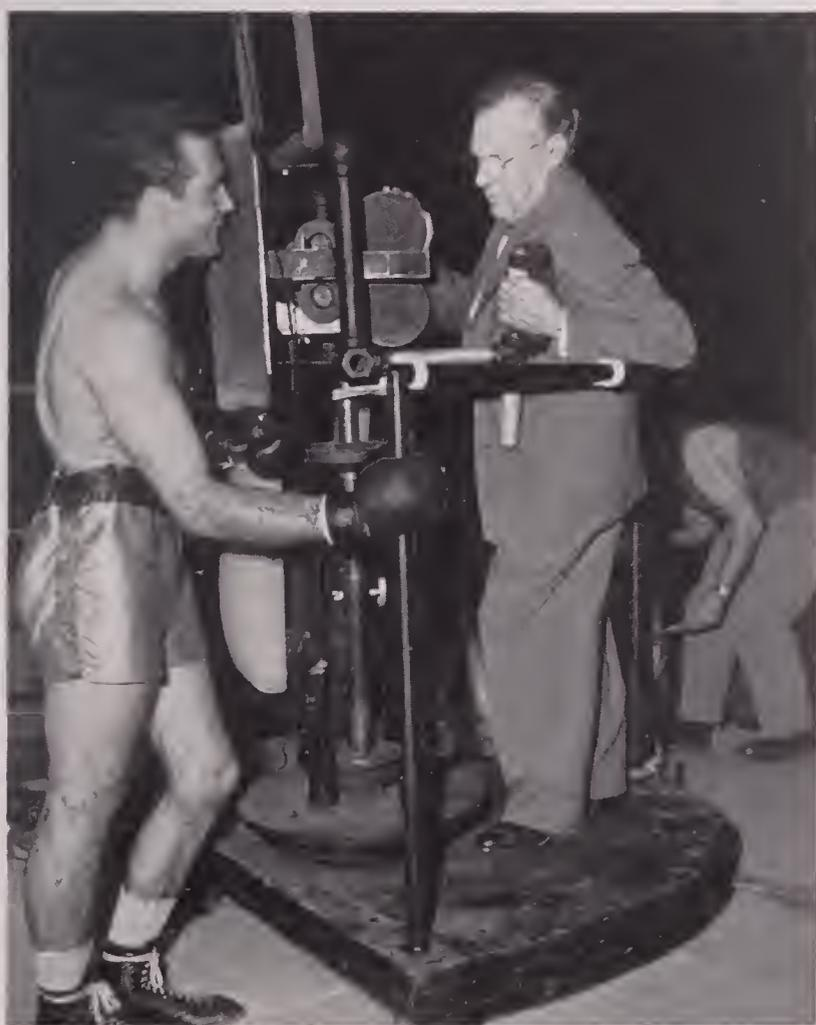
NORBERT BRODINE explains operation of the boxing camera dolly to Ricardo Montalban, star of M-G-M's "Right Cross." Action is photographed with an Eyemo camera operating at 32 f.p.s. Note padded body rest for camera operator.
