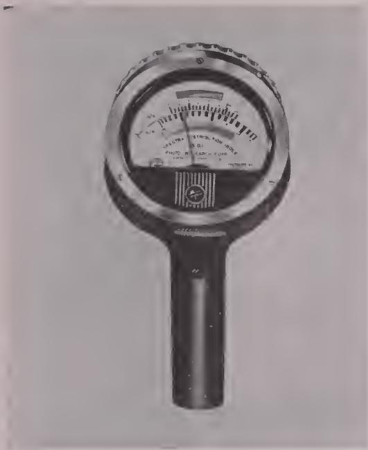
FIG. 1—The new Spectra 3-Color Meter which measures the proportionate amounts of all three primary colors of light.
