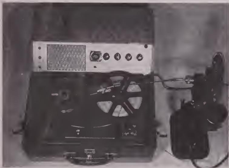
SHOWING Brush Soundmirror hookup with 8mm. projector to provide "lip-sync" sound for silent home movie films. Both recording and playback are effected through same instrument.
