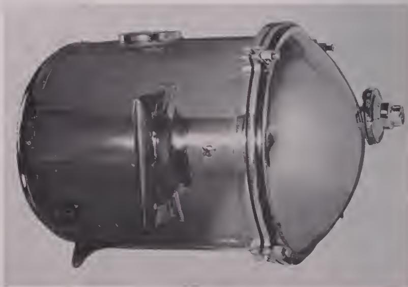
**SUBMARINE** housing for electrically-driven 35mm. motion picture camera described by author. Camera is Vinton model "K" movement which takes 200 foot film magazines, is fitted with 25mm. f/2 Cooke "Panchro" lens, and operated by remote control in handgrip.
