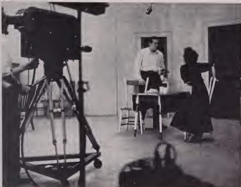
THE SINGLE TV camera employed on many budget video shows is made to do the work of two or three by means of a dolly which enables the operator to follow the action in long, sustained shots, but with variety in the camera angles. It also requires a cameraman figuratively mounted on roller skates to keep up with demands of the changing action.
