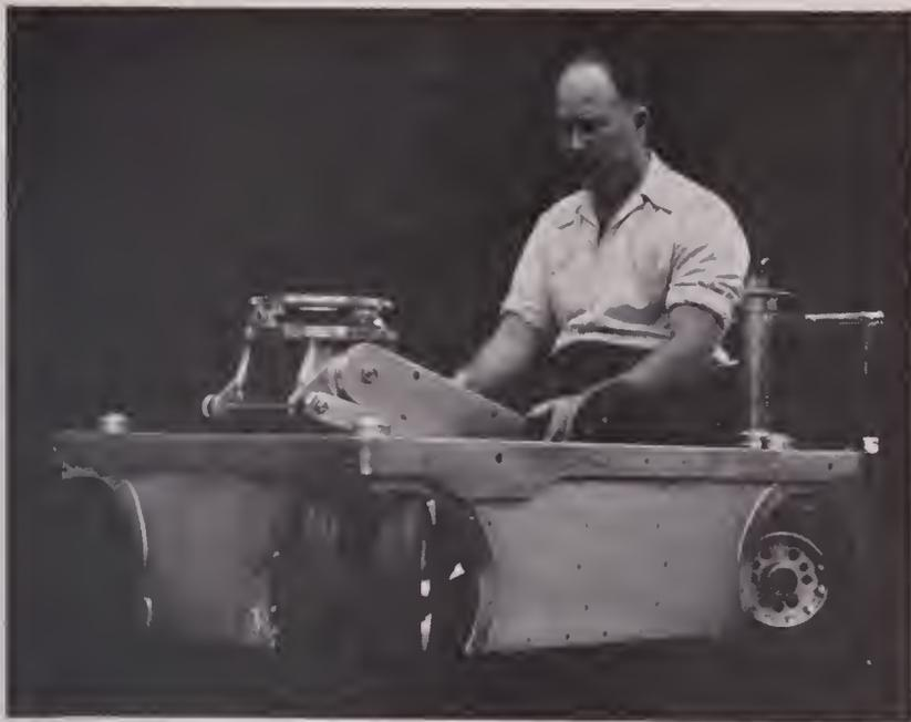
DESIGNER-builder, Steve Krilanovich, demonstrates important feature of his Dual Steering Camera Dolly which permits operator to sit in well, behind camera. When fully retracted, base of camera is but 15 inches from floor.
