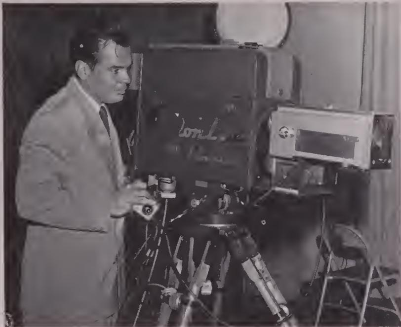
TINY MOTOR drives zooming mechanism of the Electra-Zoom lens, first of kind to be so controlled. Zoom may be stopped at any point within the lens' range at discretion of cameraman operating pushbutton remote control, as he watches results in camera's electronic viewfinder.
