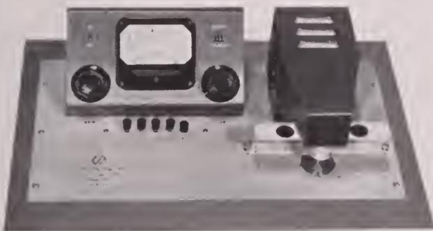
The P.R.C. Color Densitometer is a precision instrument which will do anything other transmission type densitometers will do, but in addition will measure with equal precision the density at any point in the visible spectrum of color film or any other transparent colored materials. Used by leading color film processing laboratories.
