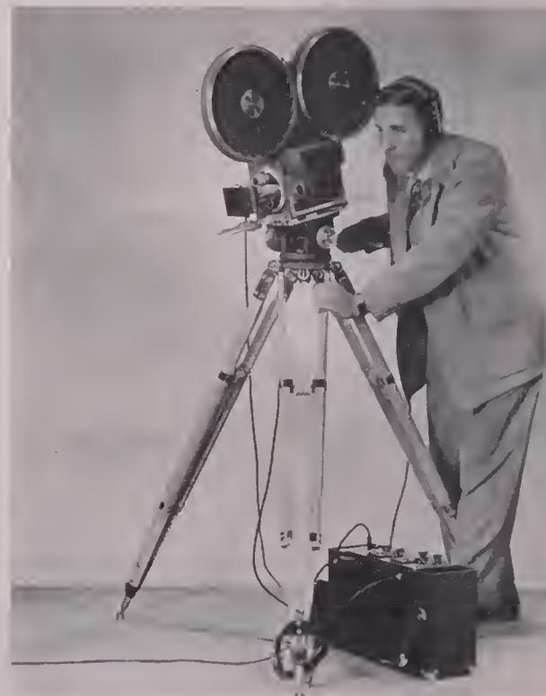
THE AURICON single-system 16mm. sound camera of wide popularity. Sound track is recorded in the camera, with the cameraman usually monitoring the sound with aid of head-set and amplifier and mixing panel on floor.
