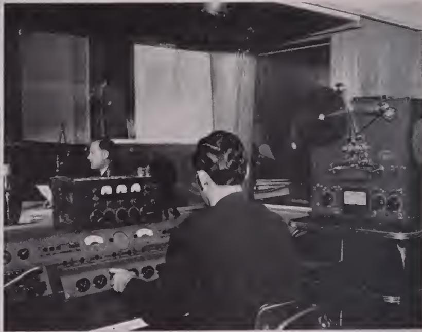
TYPICAL setup of a commercial sound laboratory. Here tape recorder is at technician's right while in the sound booth, narrator speaks into microphone as he watches film unfold on the screen (not shown).
