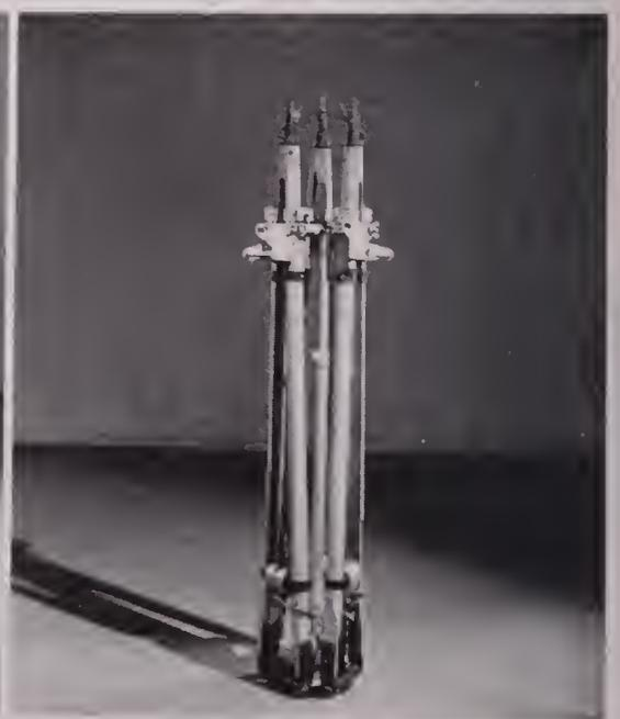
FIG. 4—The Easi-Lift may be left attached to tripod and folded for storage or easy carrying when not in use.
