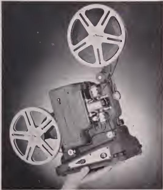
at \$167.25. Features include rapid, positive "snap" threading; gate can be opened and cleaned while film is running; automatic loop former; room-light coupling for automatically turning room light on and off; filtered light to prevent heat damage to film; 500 watt lamp; simple motor rewind, and coated 20mm. f/1.6 Kern-Paillard projection lens.
