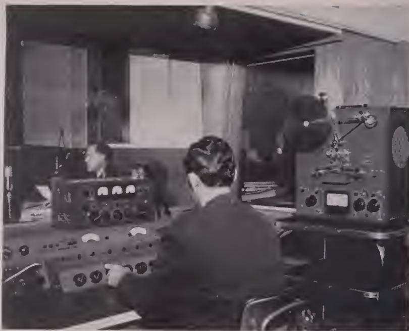
**RECORDING** commentary for a two-reel industrial film at Telefilm's sound studio, using one of the Kinevox magnetic film recorders, which is part of that company's modern sound equipment.
