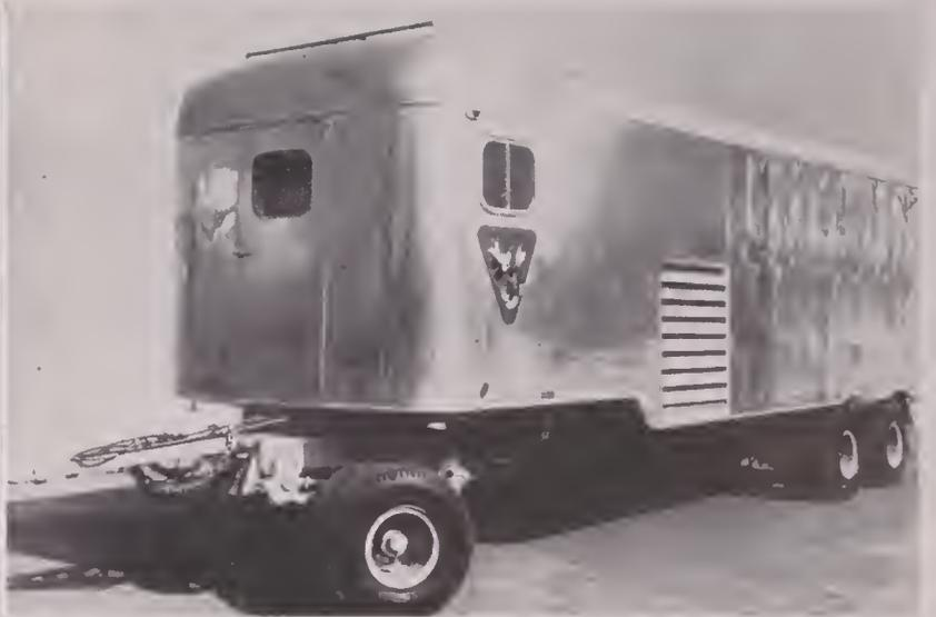
**TODAY** — This compact Westinghouse motor-generator set packs a punch—600 kilowatts worth. Disney Studio engineers designed it with an eye to safety and efficiency. So perfectly insulated is the housing that generator may be operated close to scene of shooting with safety.
