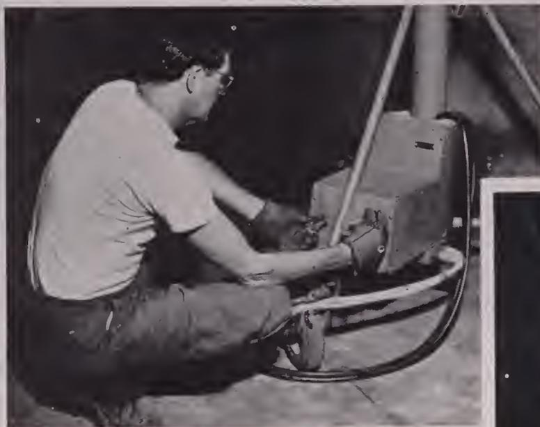
OPERATOR at hydraulic controls. A flick of switch will elevate lamp stand to desired height; opening valve at left will allow it to descend.
