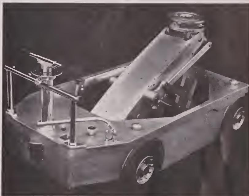
BUSINESS-end of dolly, showing steering arm, gear shift, directional adjustments, and hydraulic lever for raising the retractable camera support. Only 32 inches wide, dolly will negotiate the average doorway on sets.
