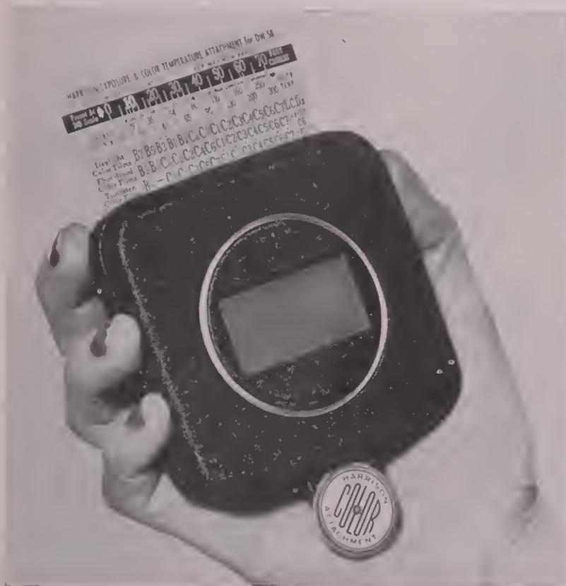
INTO THE rectangular opening in center of Harrison Color Attachment the G. E. exposure meter is snapped in place to provide a combination instrument that gives both color temperature and light intensity readings for color photography. Conversion tables at top give data on CC filters to use for color correction.
