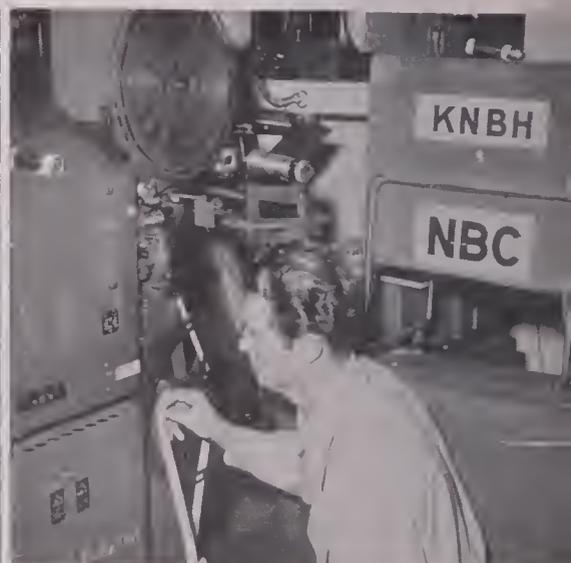
THE PROCESSED film is threaded in the special TV projector, which is started on cue from the monitor engineer.
