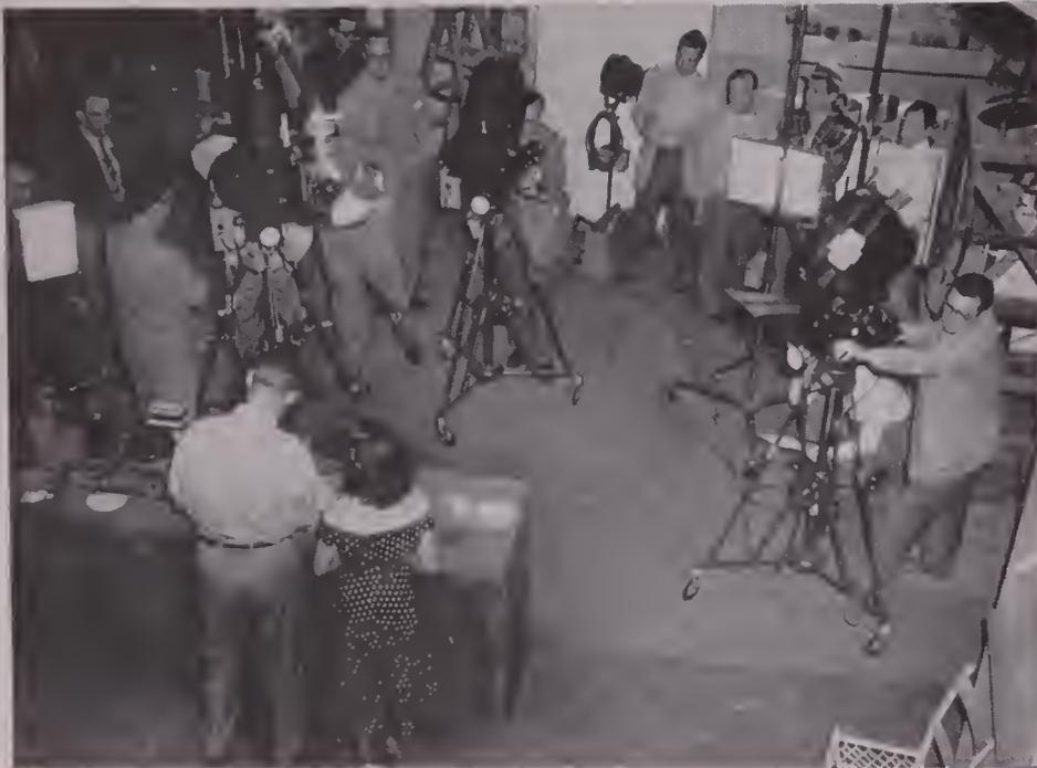
FIG. 1—Typical multiple-camera setup for shooting television films in the Jerry Fairbanks' studio in Hollywood. Cameras film continuous action from three or more different angles, supplying variety of shots for intercutting without need for new camera setups for medium and closeup shots. Method speeds production and nets better performances by players.
