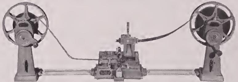
For amateur or professional, here's a new-type splicer . . . for 16mm or 8mm . . . sound or silent . . . color or black-and-white film. Gives you a film-saving straight cut at the frame line. And lowest visibility. Splice is only .070" wide!
