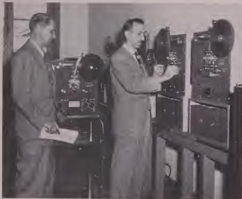
**SIMPLICITY** of dubbing magnetic film to picture track is demonstrated by Telefilm's sound engineer, Peter Gioga, to Jim Pinkham, company's ad head. Equipment shown is Kinevox.
