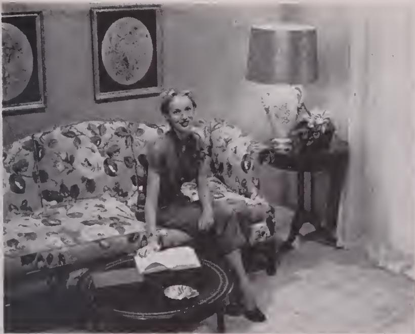
**TYPICAL** studio set for a TV film in which large un'form'y toned areas have been broken up by a pattern design, in order to reduce the "horizontal smear" effect frequently seen in the receiver image.
