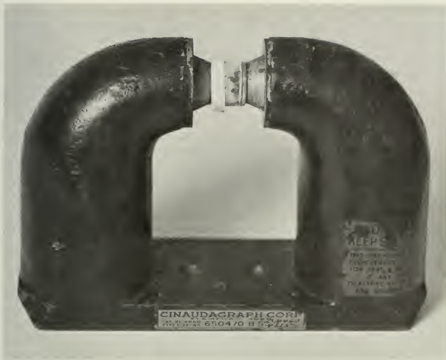
Fig. 1. Permanent magnet with rearing unit in place between the poles of the magnet.
