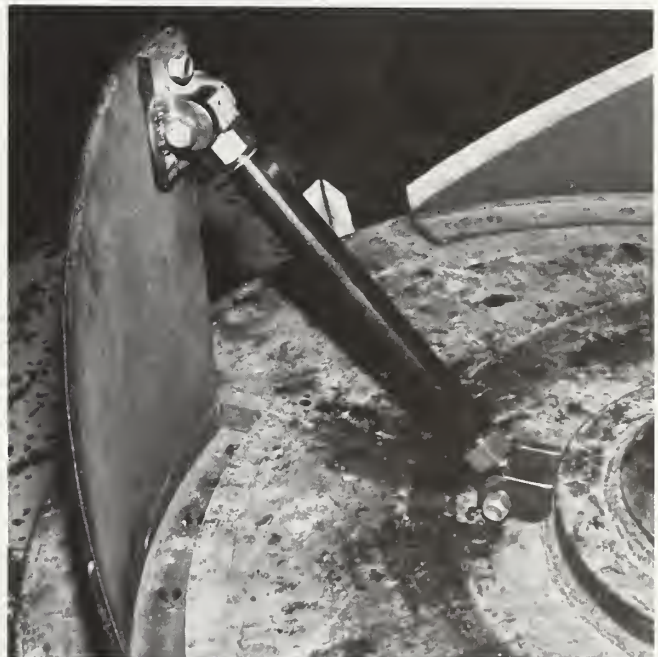
Figure 19.—Rear support added to blade to reduce blade damage and fatigue cracks. The device did not help remedy the problem.
