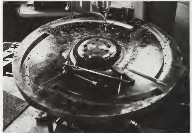
Figure 15.—Cutter wheel showing two different cutting pitches. Only two opposite grooves are used at one time.
