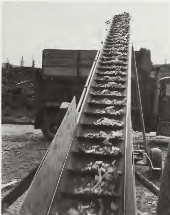
Figure 5.—Chunks loaded with conveyor instead of being blown into transport as is done with conventional chippers.
