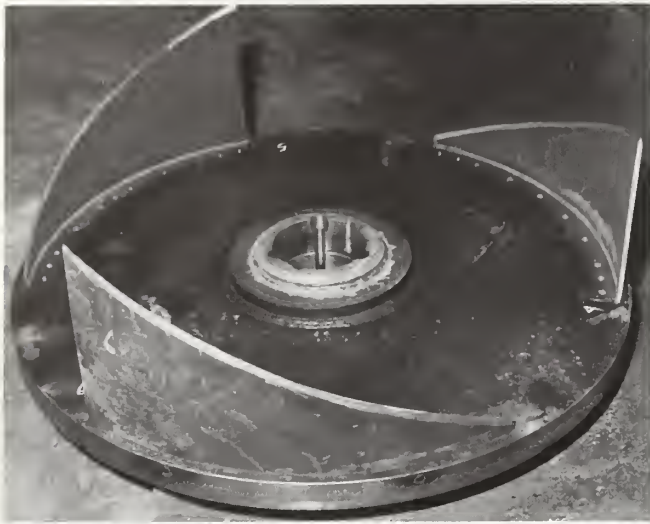
Figure 14.—Cutter blade with three blades and no pitch offset. (Pitch is the radial distance between the leading and trailing edges of the blade.)
