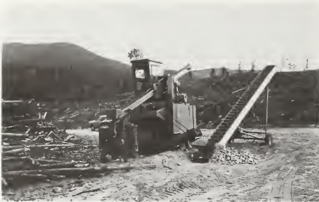
Figure 3.—MTDC wood chucker (modified Morback Model 20 Wood Chipper).
