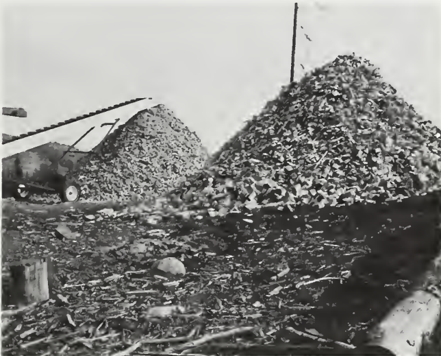
Figure 17.—Chunks in foreground are from green material and are larger and more intact. Chunks in background are from dry material. The fibers are approximately the same length but are smaller in size and more fragmented.
