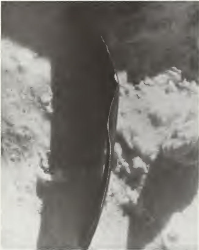
Figure 20a.—Blade damage sustained while cutting frozen hardwood.
