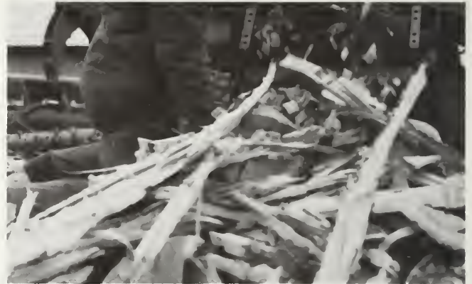
Figure 20b.—Banana peels or slivers occurred as a result of flexing on the bottom of the blade.
