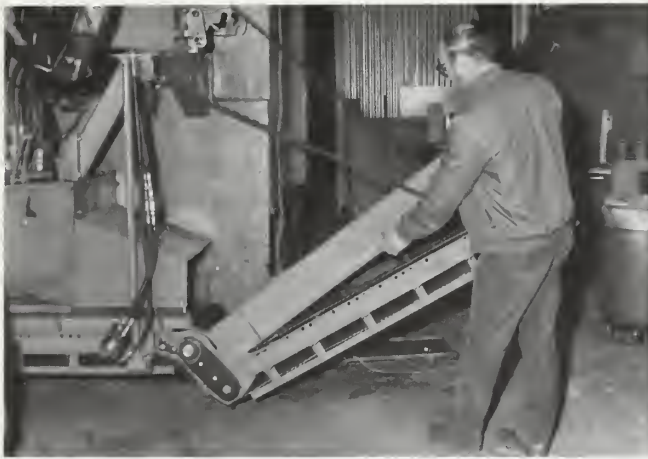
Figure 9.—Chunker incline conveyor in operating position.
