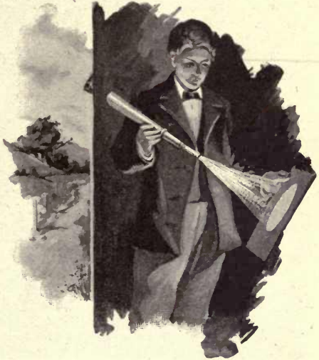
FIG. 56. — Showing how an image of the sun may be thrown on a screen with a spyglass.
