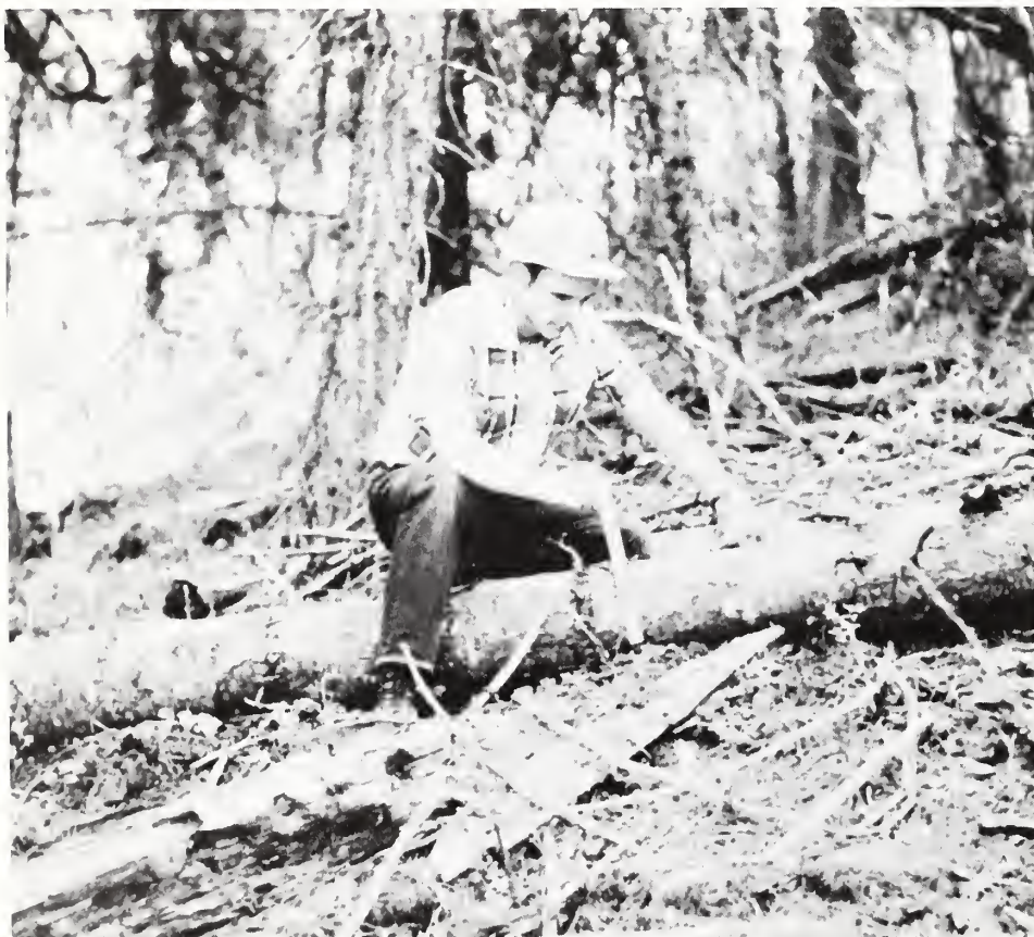
Scientist samples and measures dead-down woody materials by diameters and number of intercepts to establish fuel loading relationships.
