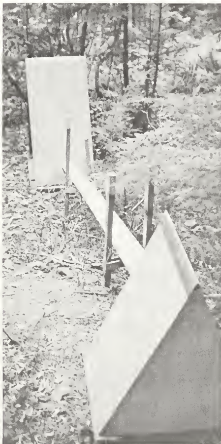
A slow-moving earth slide has split a cedar tree. Progress of the slide is being measured by a crack meter and related to factors such as rainfall.
