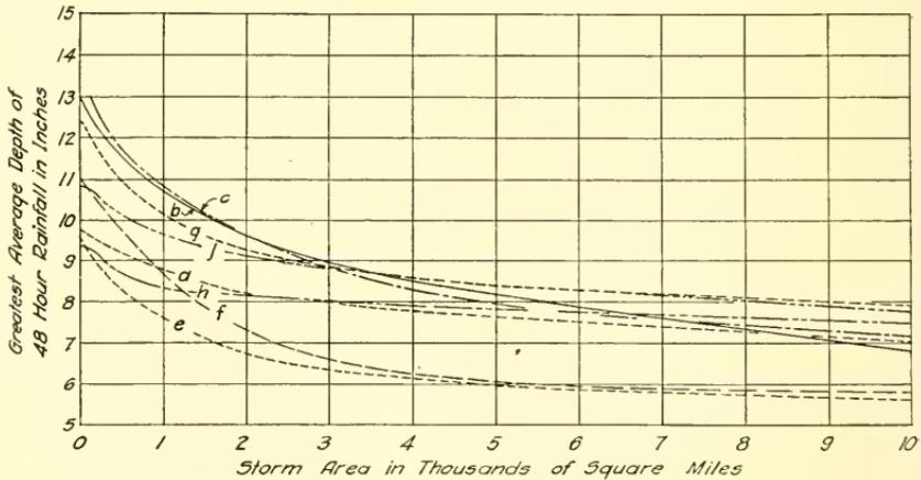
FIG. 156.—Time-Area-Depth Curve for 48-Hour Storm.
