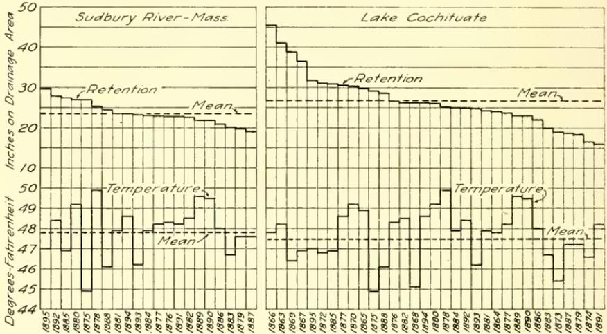
FIG. 297.—Diagrams of Retention and Temperature for Two Streams in Eastern United States. After G. W. Rafter.
