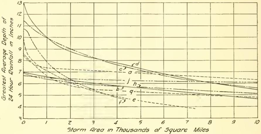
FIG. 155.—Time-Area-Depth Curve for 24-Hour Storm.
