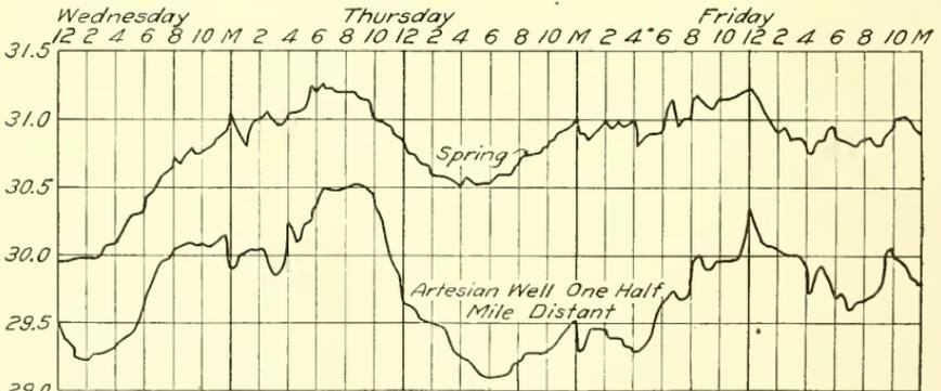
D Effect of Barometric Pressure on Discharge of Springs and Wells (King)
