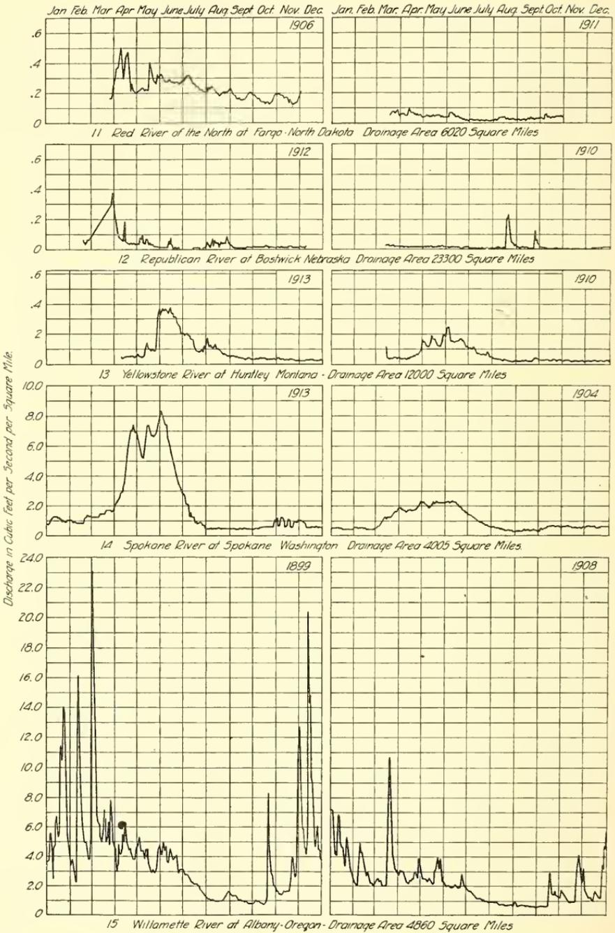
FIG. 260.—Hydrographs of Various Streams for Years of High and Low Flow.
