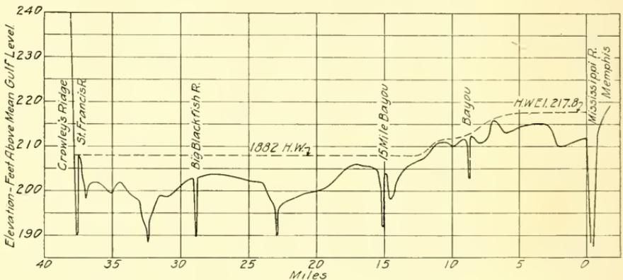
FIG. 338.—Profile of the Alluvial Flood Plain of the Mississippi River from Memphis, Tenn., to Crowley's Ridge, Ark., along the C. R. I. & P. Ry. After Mississippi River Commission.
