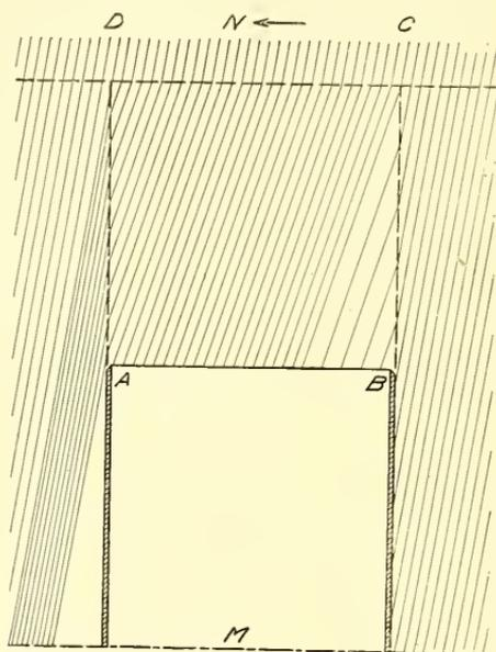
Fig. 107.—Effect of Wind upon the Catchment of the Rain Gage (See page 191).
