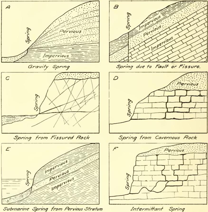
FIG. 233.—Geological Conditions which give Rise to Various Classes of Springs (see page 399).
