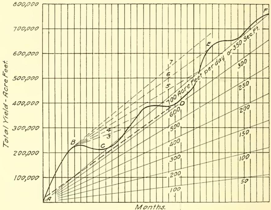
FIG. 298.—Diagram of Rippl Method of Storage Calculations.
