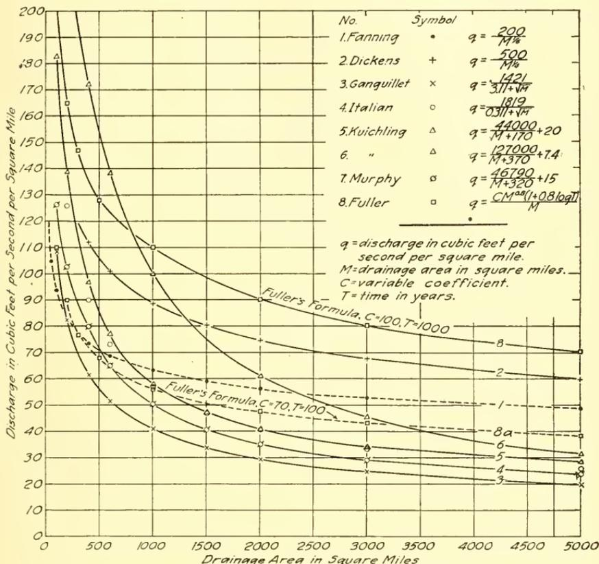
Fig. 340.—A Comparison of Various Runoff Formulas.
