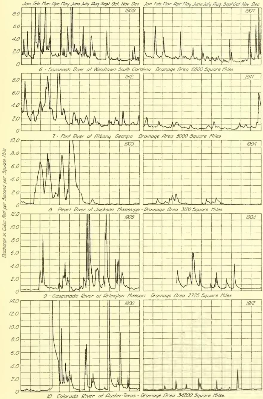
FIG. 259.—Hydrographs of Various Streams for Years of High and Low Flow.
