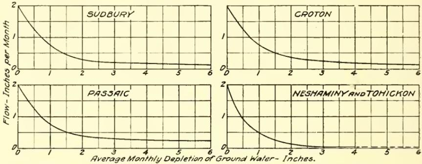
FIG. 289.—Grounds Flow Curves of Eastern Streams. After C. C. Vermuele.
