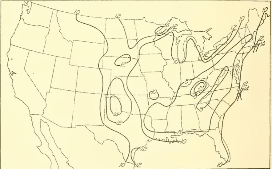
Fig. 34.—Average Hourly Velocity of Wind Estimated for Elevation of 100 feet above Surface<sup>5</sup> (see page 71).
