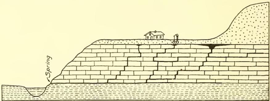
FIG. 248.—Pollution of Spring from Surface and Subsurface Drainage (see page 415).
