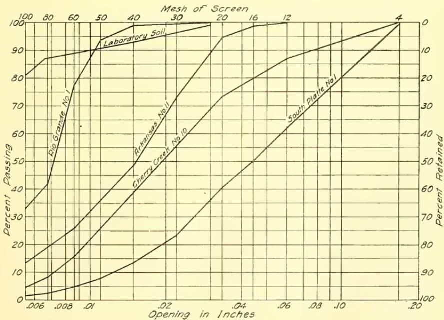
FIG. 87.—Mechanical Analysis of River Bed Materials.
