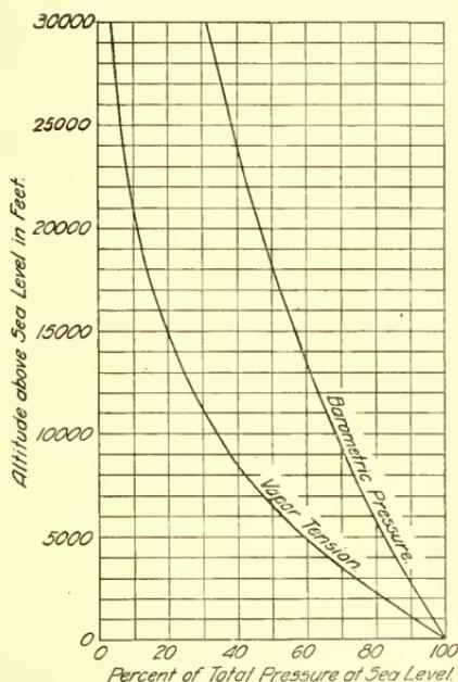
FIG. 65.—Decrease of Vapor Tension and Pressure with Increase in Altitude. in atmospheric pressure is given in percentages of such tension and pressure at sea level.<sup>7</sup>
