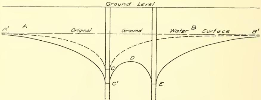
FIG. 255.—Illustration of the Interference of Wells.
