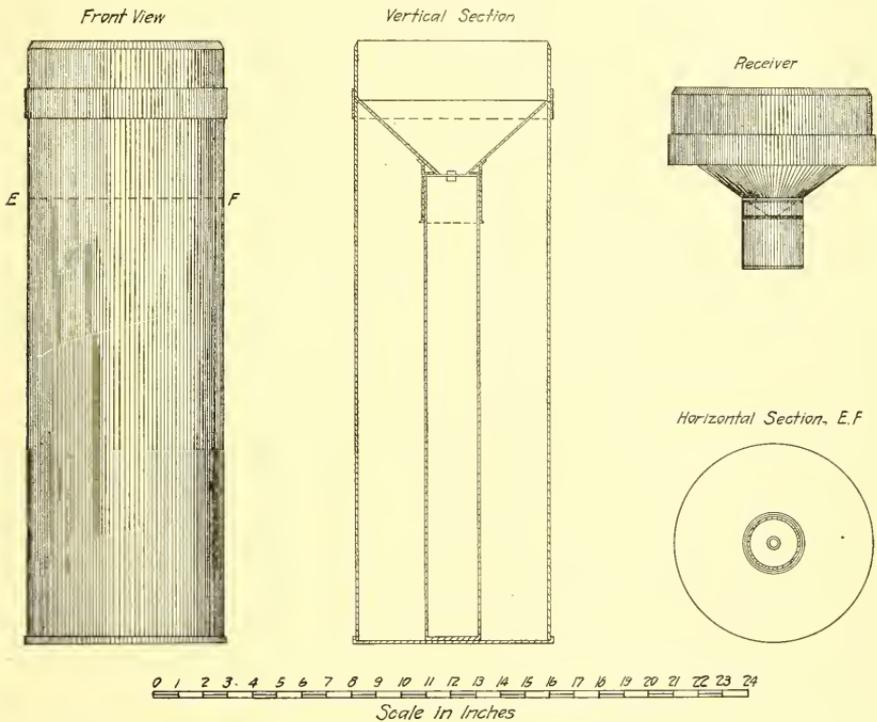
FIG. 106.—The Ordinary Form of Rain Gage
