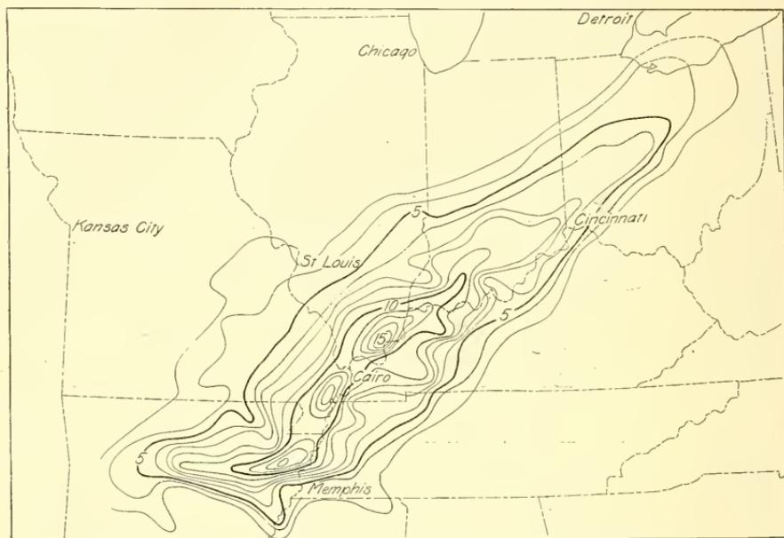
FIG. 150.—Isohyetal Lines for Storm of October 4-7, 1910.
