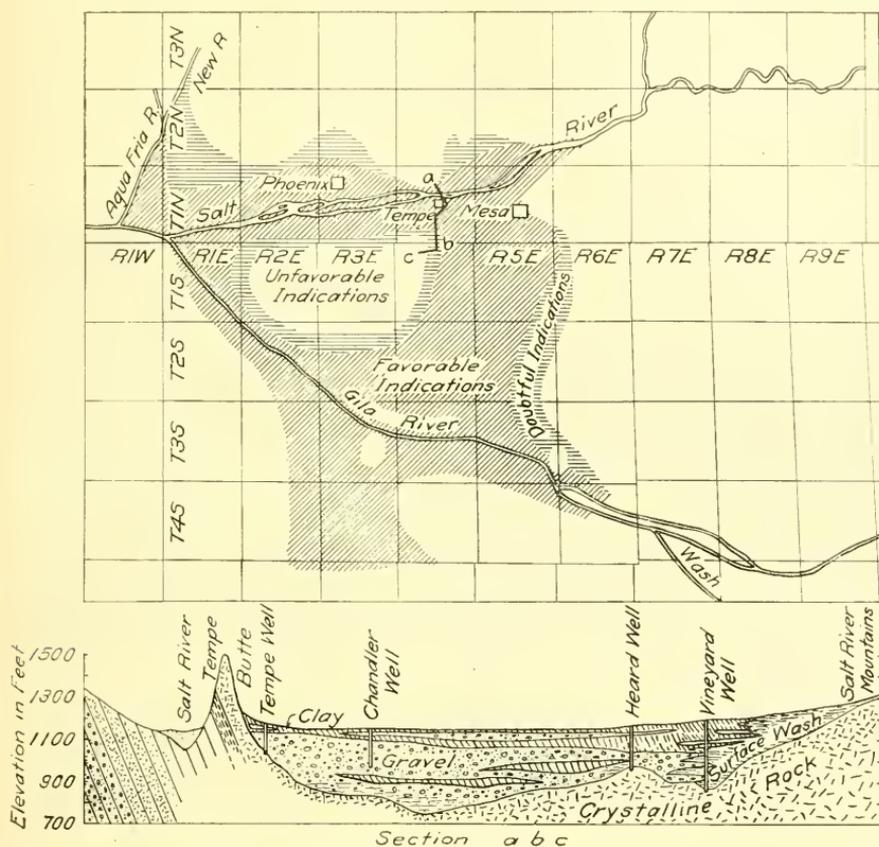
FIG. 242.—Map and Section Showing Ground Water Conditions in the Gila and Salt River Valleys. After Lee. (See page 408.)
