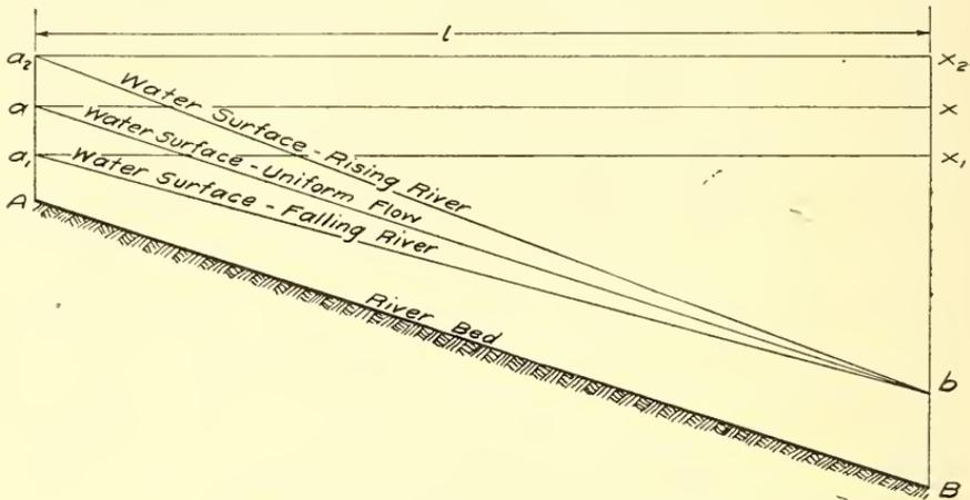
FIG. 281.—Flow in a Uniform Channel.
