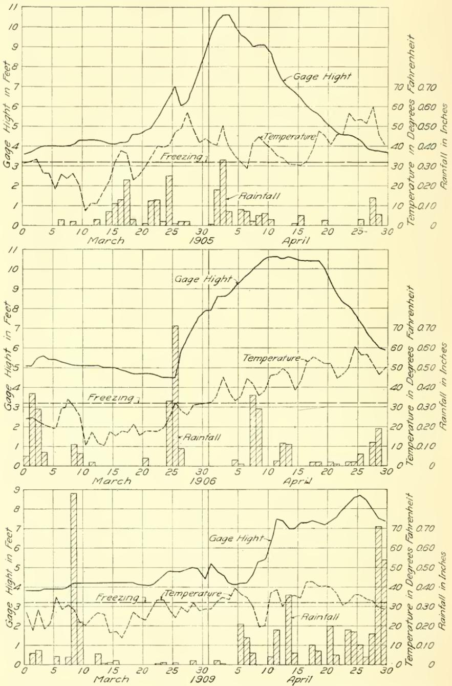
FIG. 267.—The Relations between Stream Flow and Rising Temperatures.
