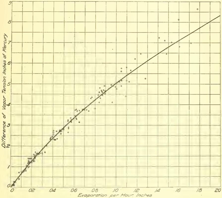
FIG. 75.—Effect of Vapor Tension on Evaporation.
