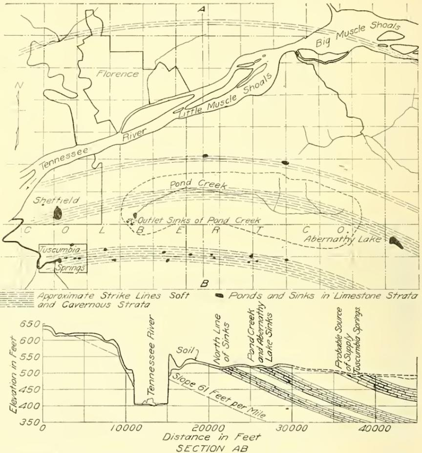
FIG. 237.—Map and Section near Sheffield, Alabama, Showing Conditions which give Rise to Disappearing Streams and to Springs.
