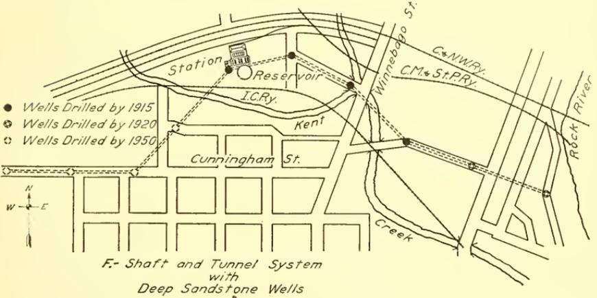
FIG. 345.—Possible Sources of Water Supply for Rockford, Illinois. yield a sufficient quantity and which seems reasonably feasible of development should be considered. In considering such various sources it is necessary to take into account not only the quantity obtainable from each but also the methods by which each can be developed and
