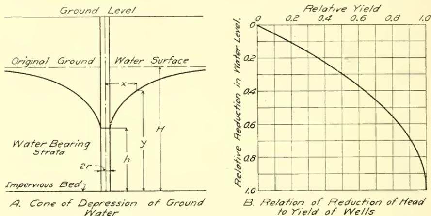
FIG. 252.—Principles of the Hydraulics of Wells.
