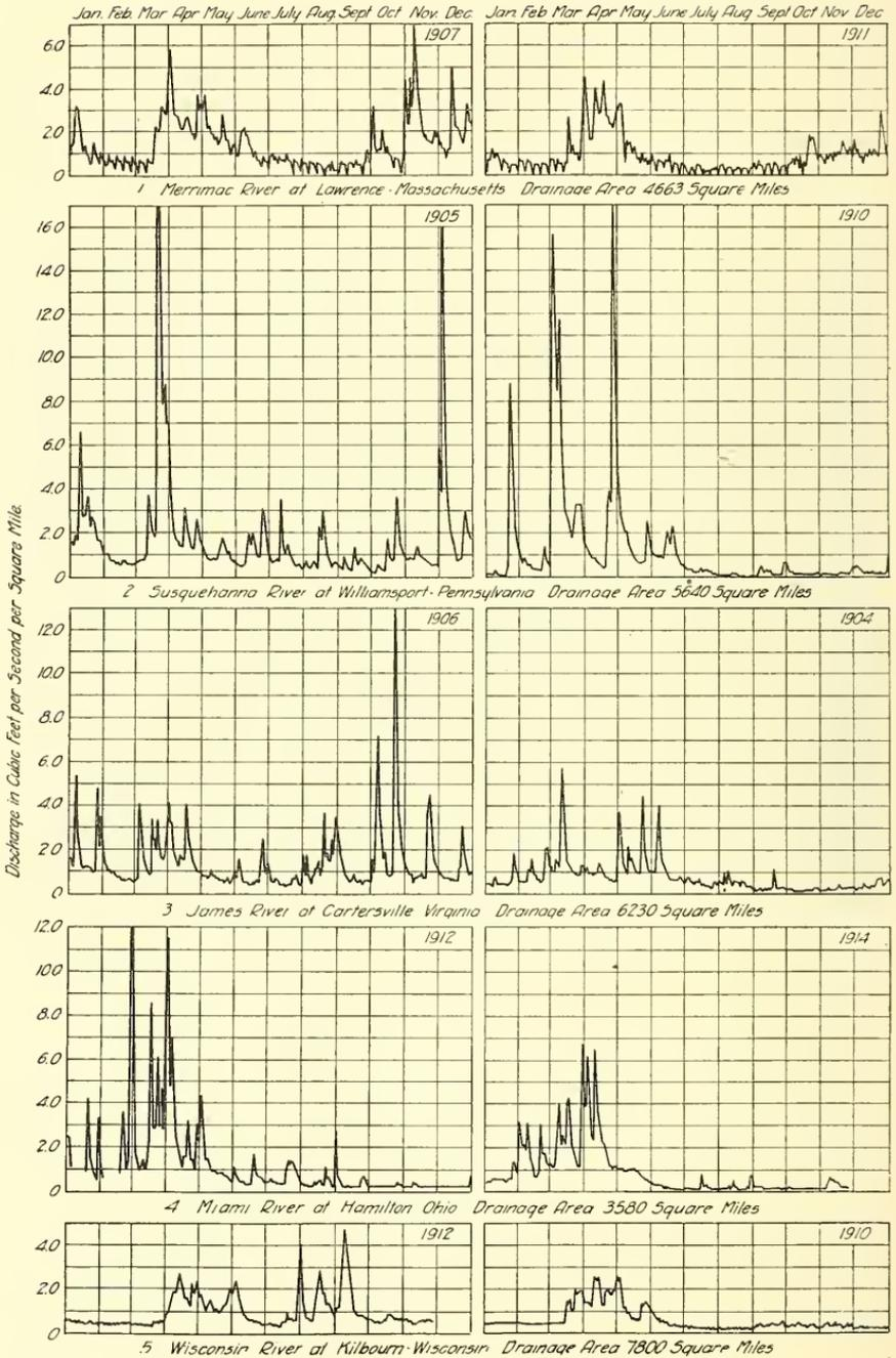
FIG. 258.—Hydrographs of Various Streams for Years of High and Low Flow.
