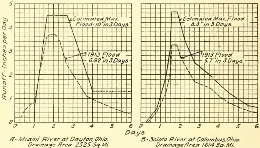
FIG. 343.—Comparison of Actual Floods of March, 1913, with ideal Maximums for which Flood Protection Works are to be designed.<sup>7,8</sup>
