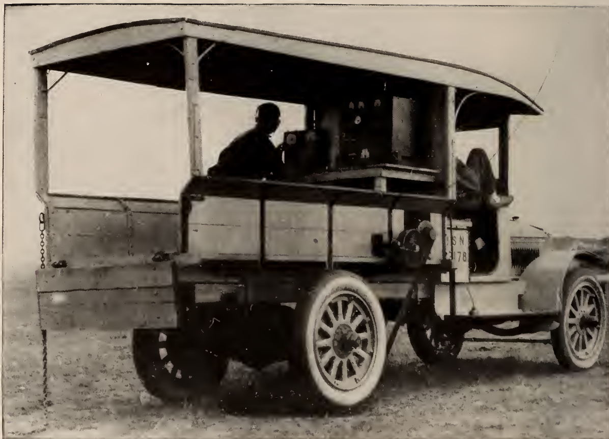
EARLY FORERUNNER OF THE RADIO JEEP was this 1925 Navy cargo truck, which Marines of Observation Squadron One (at Naval Air Station, North Island, San Diego, California) fitted with radio equipment to produce the first air-ground communications vehicle. Motive power for the system's electrical generator was furnished by a jacked-up right rear wheel and a belt drive.
