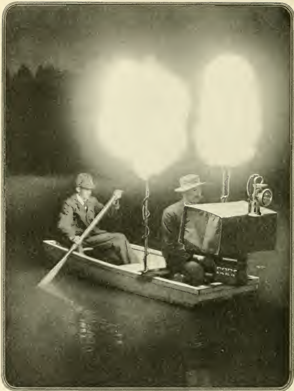
An outfit for photographing animals from the bow of the boat. A wooden revolving camera bed, large enough to carry two cameras, is secured to a ball-bearing support which is rigid, absolutely noiseless and enables the camera to be swung through an angle of one hundred and eighty degrees. When the lantern shines on the animal the flash-powder may be fired, provided the distance is correct. If desired, one lamp may be fired after the other successively, to show the animal in different positions. This requires two firing lines and two cameras
