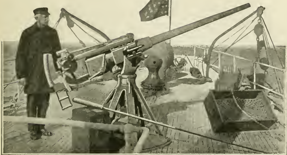
In Line Shooting with the Rapid-Fire Guns a Projectile About Six Feet Long Is Used. The End Which Is Inserted in the Gun Is a Cylindrical Piece of Steel Slightly Smaller Than the Bore of the Gun. The Line Is a Hemp Rope About the Size of a Wash Line
