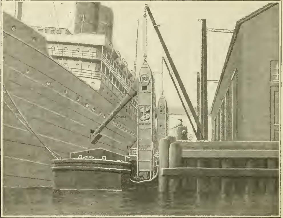
An endless bucket-chain passes into the barge and thence up the conveyor to the discharging point at the top of the chute. This loader has coaled the "Vaterland" in twenty-one hours
