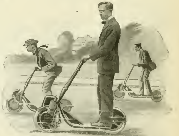
The handlebar controls the speed of the machine, steers it and operates the brake and the clutch
