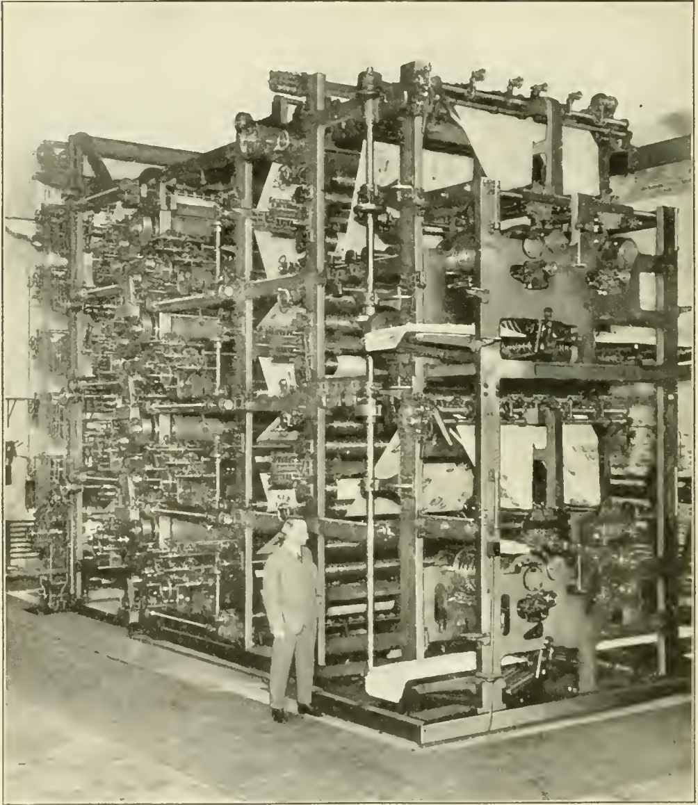
Over two hundred inventions are incorporated in the mechanism of the machine. The coordination of the various parts of the folder was obtained by distributing air pressures and vacuums so that the paper is carried, not pulled, along
