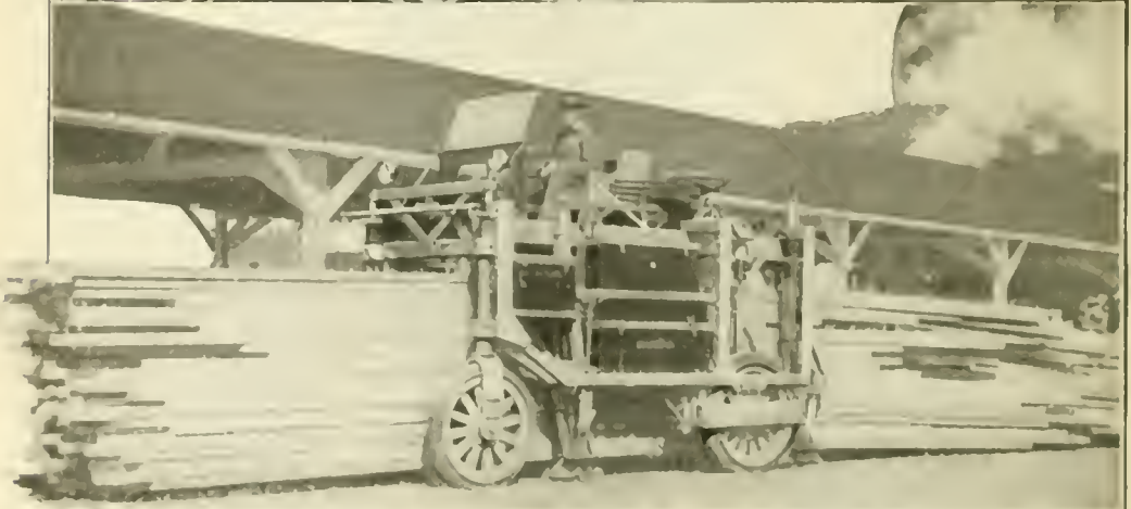
Below: A lumber truck which picks up its load without help
