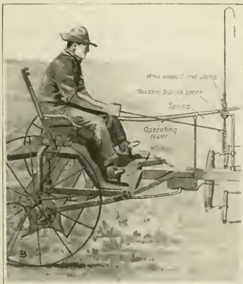
By means of a lever, this whip can be applied in any direction
