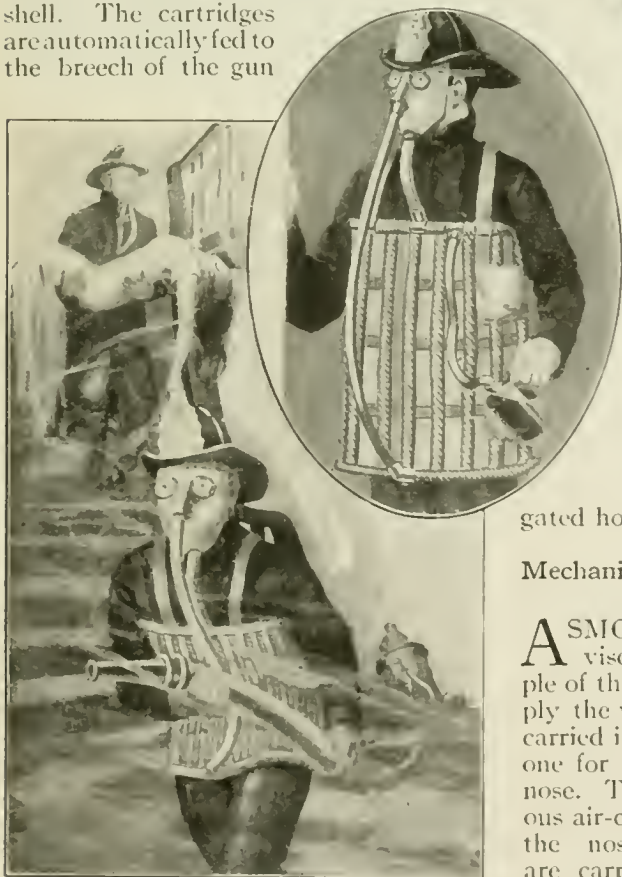
The suit is provided with numerous tubes through which air passes to the wearer
