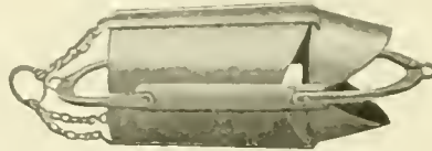
The expansion bucket, which is used with a trolley-jack. The jaws are sharpened for scraping
