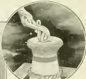
Where large quantities of brass and iron filings accumulate this magnet will be found invaluable for separating them
