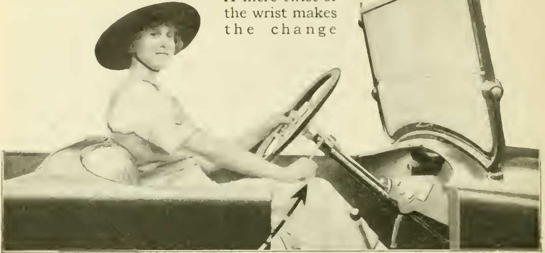
The transformation from a twelve to a six-cylinder automobile is accomplished simply by turning a lever carried under the steering-wheel. This cuts out the left-hand block of six cylinders
