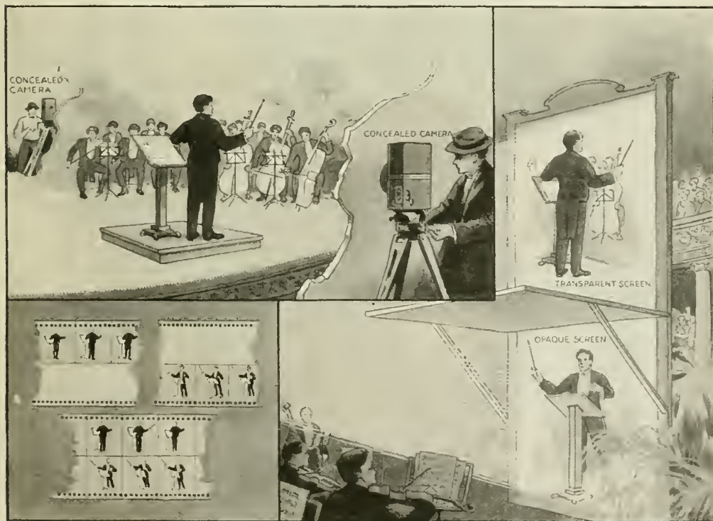
At the upper left the two concealed cameras are shown. Each takes but half a negative, the halves being pieced together as in the lower left picture. A screen having a transparent portion for the audience to see and an opaque portion for the musicians alone, is employed
