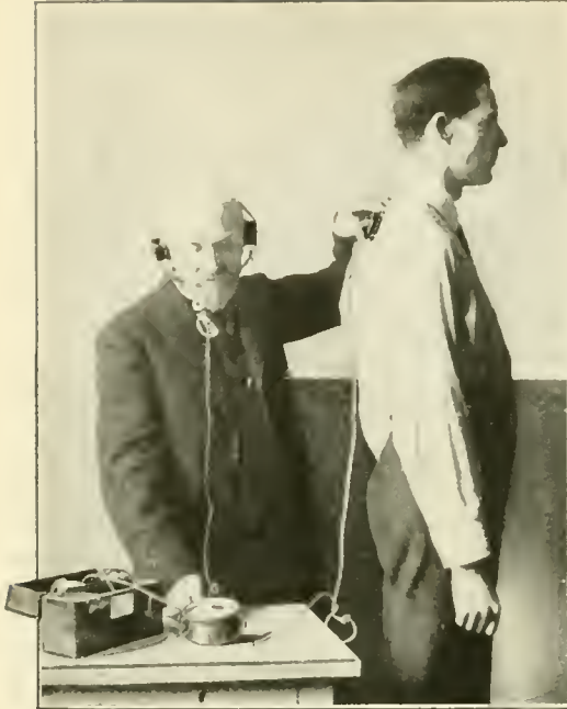
Hold a microphone against your back and it will pick up the sound of your voice
