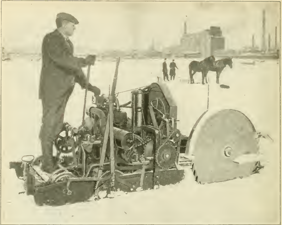
The saw is geared directly to the motor and works in either direction. It will cut thirty thousand cakes of ice per day, thus equaling the work of sixteen men with eight horse-teams
