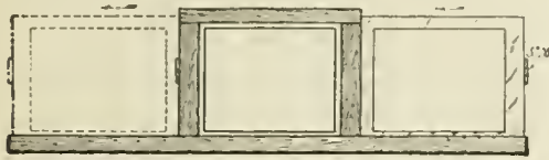
Fig. 3. A slide-carrier of the conventional sort, one of the parts to be purchased
