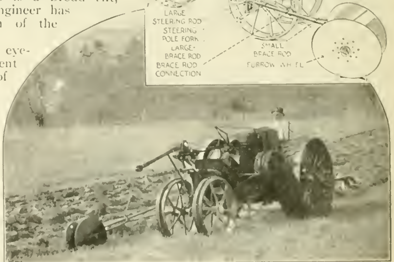
The device is adjustable so that the tractor will run almost any desired distance from the furrow
