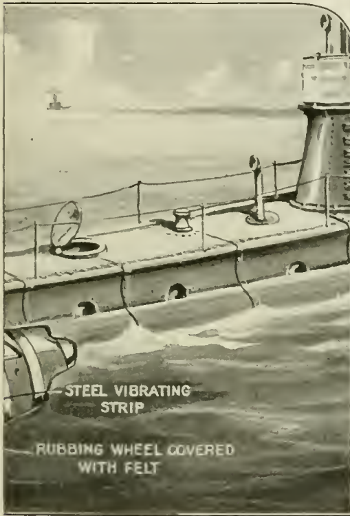
Vibrations from the interior of the ship's hull do not interfere with the signals
