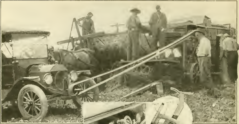
Above: Threshing with a Ford. The power is taken directly off the crankshaft by means of a novel device Below: A lamp socket warmer for engine and radiator during the winter
