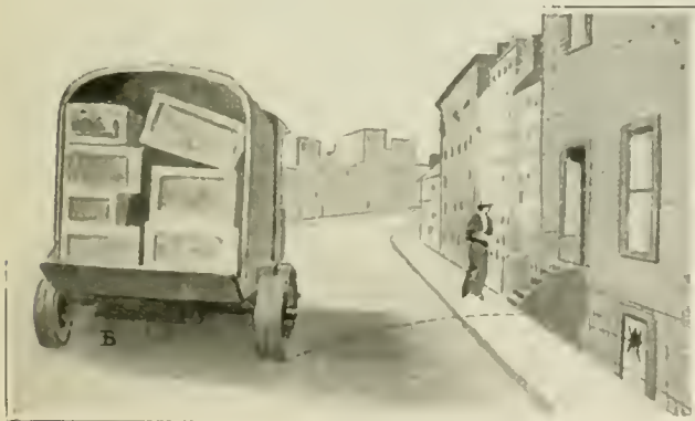
The heavy wheel of a motor-truck shoots pebbles that break unprotected windows
