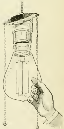
A pull-socket made from a key-socket
