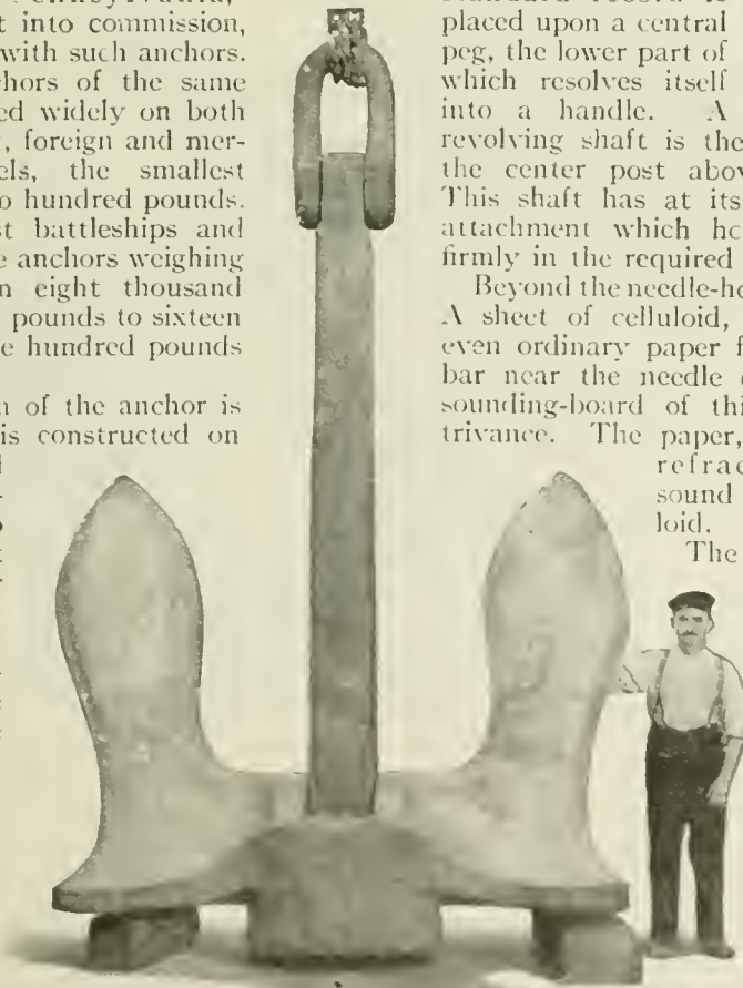
The Anchor Is Constructed on the Principle of a Ball and Socket, with the Fluke or Main Portion in One Piece
