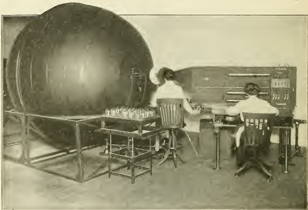
A one hundred-inch sphere photometer used for light-testing work. A sight box, large photometer-bar, movable comparison lamp and scale graduated in millimeters are essential elements
