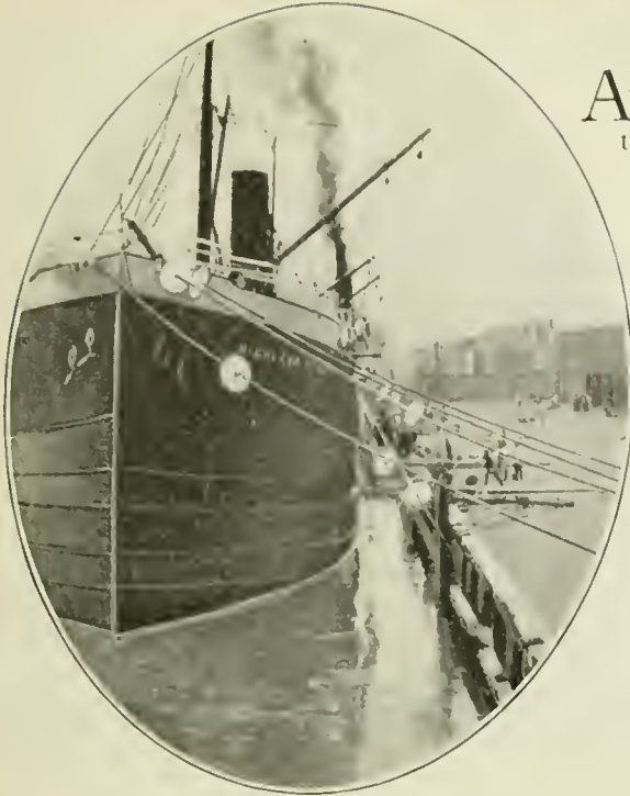
The Rat-Guard Is a Circular Disk of Galvanized Iron About Eighteen Inches in Diameter
