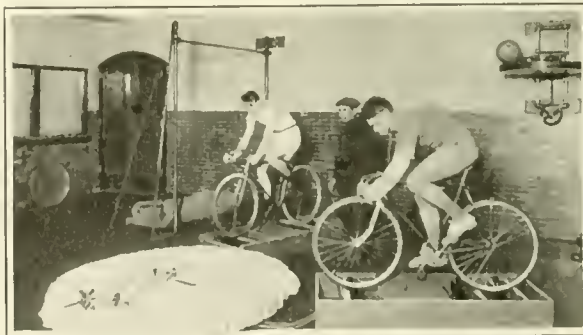
Two miniature bicycle riders race around a miniature track, their speed corresponding to that of the athletes on the bicycles over the rollers
