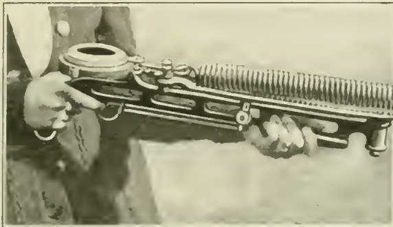
A Clay Bird Trap Operated by Pulling the Trigger. This Is the Most Common Form of Automatic Trap
