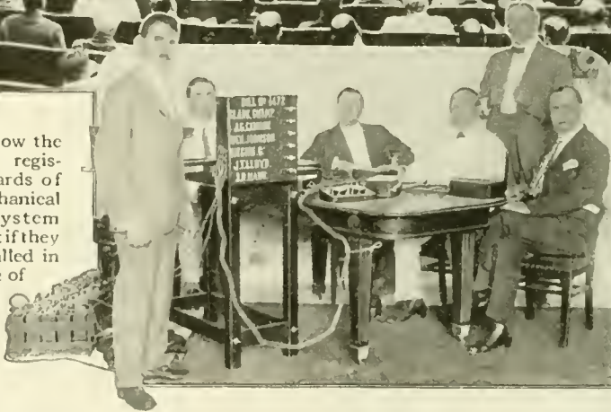
At left: The mechanical voter reduced to a demonstrable size with batteries and connections for a committee examination. It is really a form of telegraph with many key-boards
