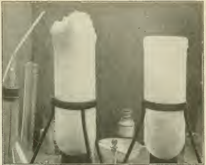
Part of condenser in a laboratory refrigerating apparatus. The chamber is so cold that frost is formed. Yet liquid air would boil briskly if placed on the tubes
