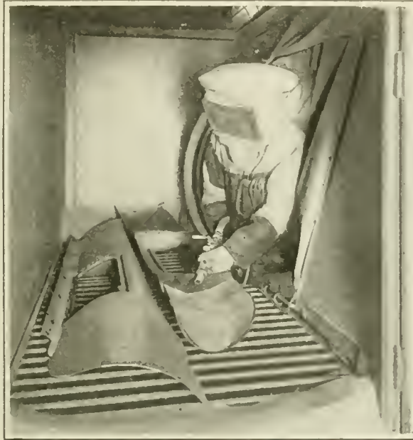
Sand Blasting Automobile Parts with the Modern Head-Dress. The Fresh Air Is Supplied Under Pressure
