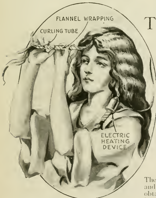
The saturated strands of hair are wrapped in flannel and heated twice by electricity
