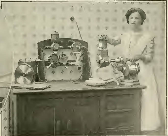
A kitchen utility tool for any number of tasks. It grinds meat and coffee, slices vegetables and freezes cream
