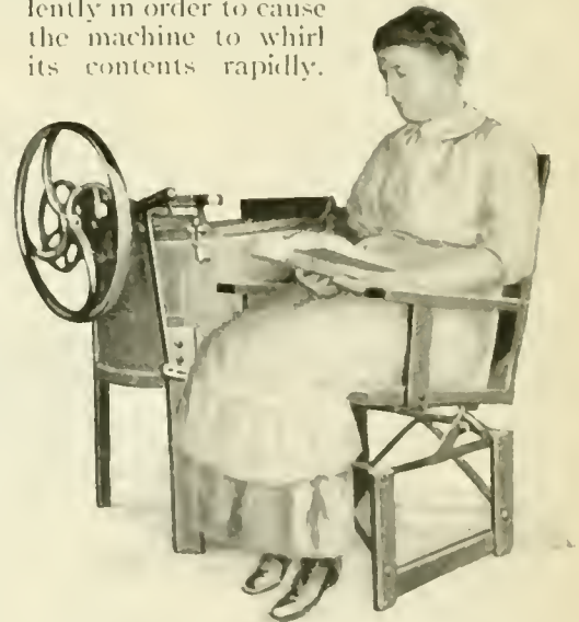
Two springs under the seat of the chair communicate the motion to the washing machine
