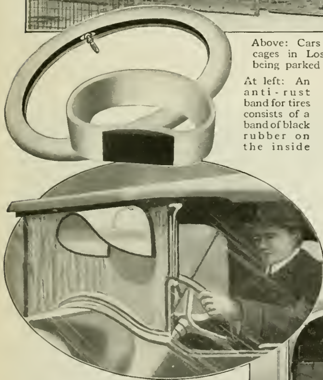
Above: A rain-shield designed to protect the driver from the rain while providing an opening for a good view
