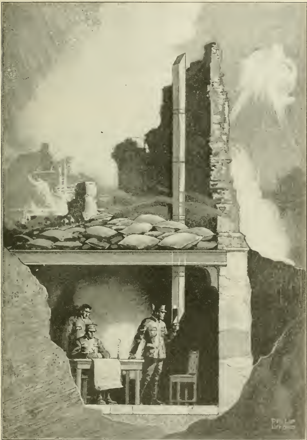
Secreted in their headquarters in the wine cellar of a demolished chateau, the officers are able to watch the battle raging outside with the aid of an immense periscope supported in its place by a wall of masonry. The roof of the cellar is covered with bomb-proof pads
