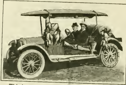
This boat can be carried to any duck pond which is accessible to an automobile; on the road it serves as a canopy
