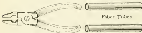
Fiber tubes driven over plier handles to form an insulation for electrical work
