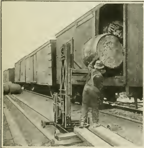
Loading barrels into freight cars is simplified by this portable elevator
