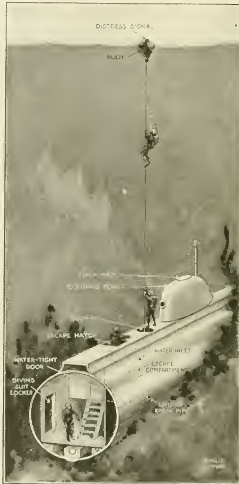
In an emergency in this submarine, the crew put on light diving jackets, escape to the top of the boat through the compartments and hatches, and climb to the surface on the cable attached to a buoy
