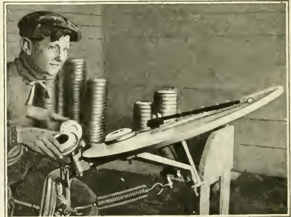
The Operator at the Trap Mechanism Below the Ground. Several Piles of Clay Birds Are Shown
