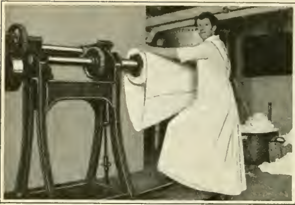
The skirt is guided by the two hands and the machine operated by treadle, to obviate all danger
