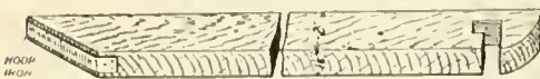
A piece of hoop-iron strengthens the lower end. An L-shaped notch at the upper end holds the line securely
