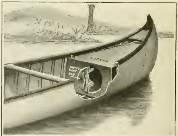
The air-tight locker is a storage place for a camping equipment and also prevents the canoe from sinking
