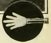
An electric flash-lamp with a bulb in the form of a hand, is one of the latest automobile signals for warning a driver behind at night
