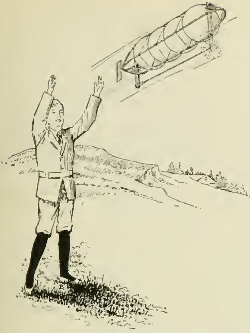
Four rubber balloons in a rattan frame, make a Zeppelin which will actually fly
