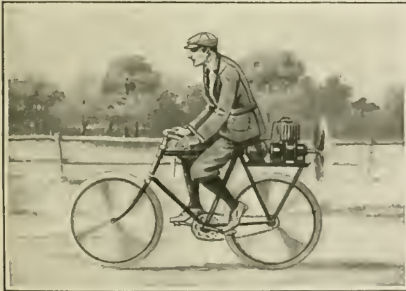
With the air-propeller attachment a speed of thirty miles an hour has been attained
