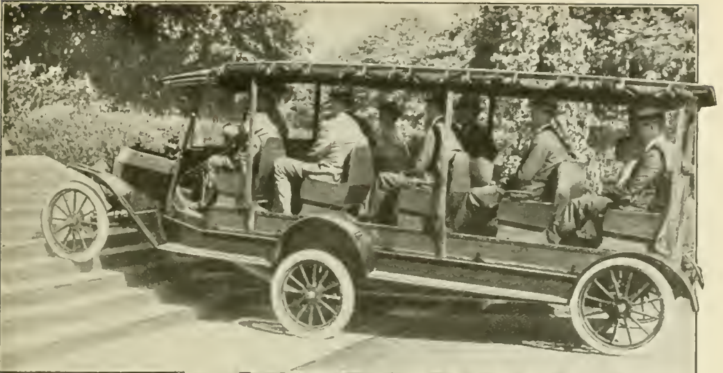
Above: An ingenious six-wheeled automobile, with the body mounted flexibly on the frame at two points (Autoport System)
