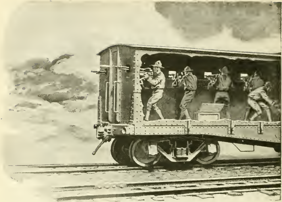
The United States Army's first armored car has twenty port-holes for machine-guns and a well in the center for a three-inch rapid-fire field piece
