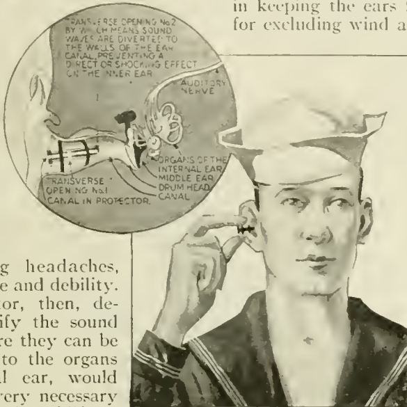
The device is a guard, not a stopper, and does not interfere with the circulation of air in the canal of the ear
