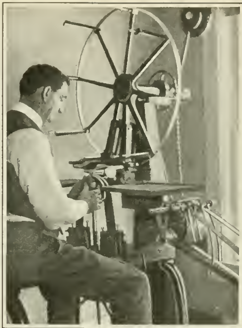
The ingenious baseball sewing-machine which pulls the covers together and stitches them
