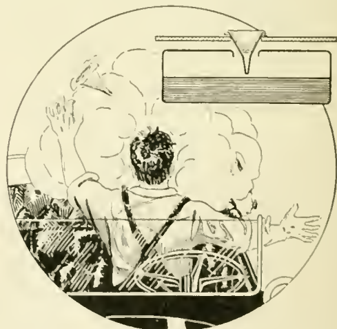
The funnel is held up by the seat board but a spark may jump the gap into the tank
