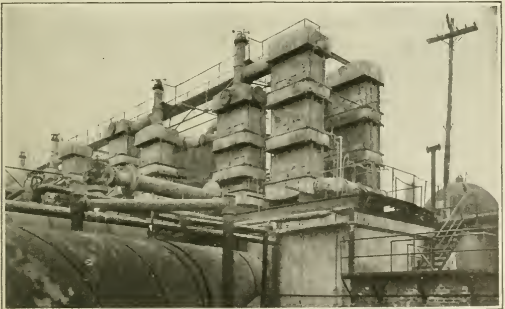
Battery of Aerial Condenser for Automatically Condensing Different Distillates, Which Are Then Conducted Through the Water-Cooled Pipes to Their Respective "Running" Tanks
