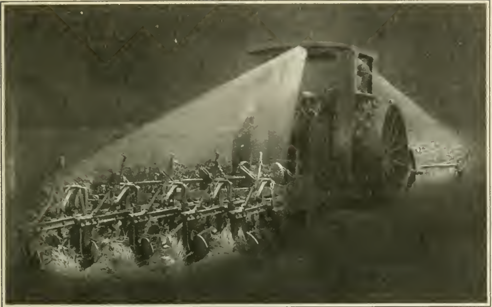
Plowing a field at night with the aid of two powerful lights which enable the operator to see the path ahead of the machine he is driving, and the width of plowed field in its wake
