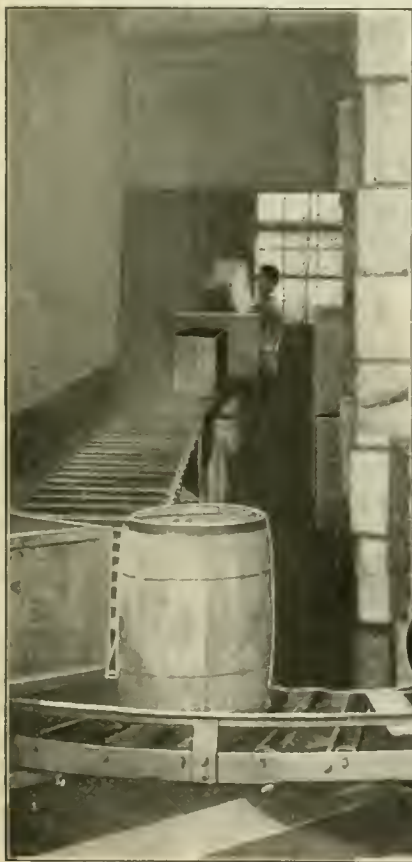
The gravity conveyer reverses the conditions of the bicycle traveling down a smooth road; it contains within itself the wheels
