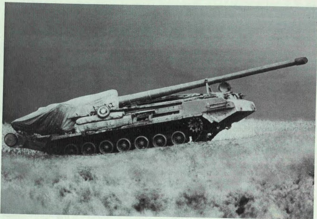
Soviet high-powered artillery such as this 203-mm self-propelled 2S7 gun can disrupt an opponent's defensive preparations by firing nuclear, high-explosive, or improved conventional rounds deep behind his lines.
