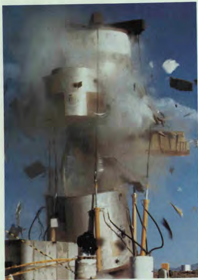
The US recently evaluated laser lethality against a ballistic missile system in a test of some SDI components. The laser used was a large chemical laser, MIRACL (Mid-Infrared Advanced Chemical Laser), which then was the most powerful continuous laser outside the Soviet Union.
