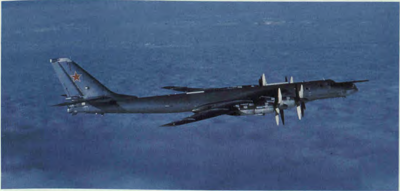
The BEAR H bomber can launch AS-15 nuclear-armed cruise missiles as far as 3,000 kilometers from their targets. These bombers often practice strike missions against North America and are routinely intercepted by North American Aerospace Defense Command fighters.
