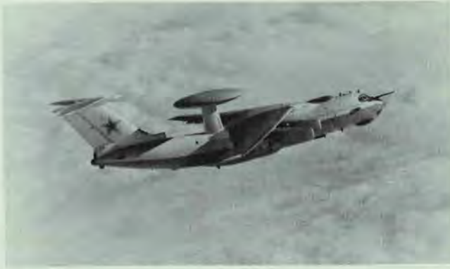
The MAINTAY AWACS aircraft substantially improves Soviet battle management capability by providing early warning against low-altitude penetration and air battle management.
