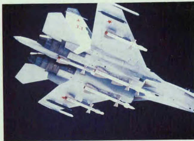
The Soviet Su-27/FLANKER, in combination with the AA-10/ALAMO missile, has true look-down/shoot-down capabilities against aircraft and possibly cruise missiles penetrating at low altitudes.
