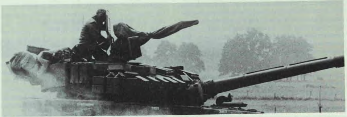
The Soviet T-80 tank, with reactive armor mounted around the turret, poses a challenge to Western antiarmor technology development.
