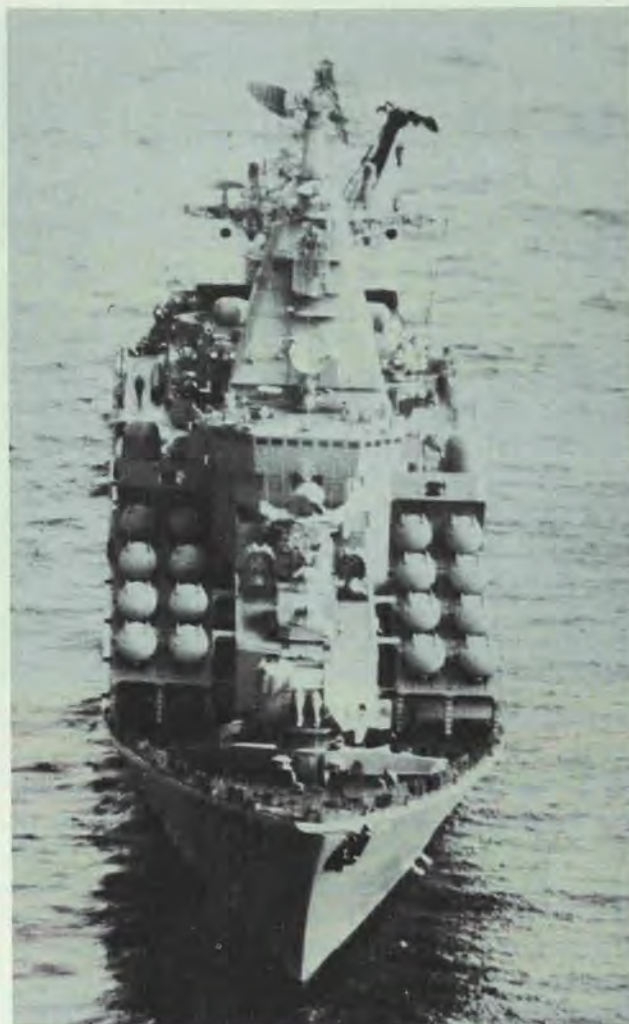
SLAVA-Class guided-missile cruisers, still being produced, are outfitted with surface-to-surface, antisubmarine, and surface-to-air weapon systems.
