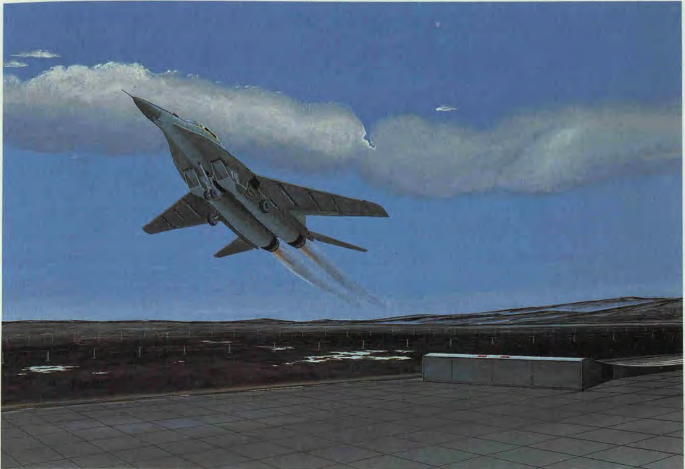
The US Navy has taken fixed-wing aircraft to sea since the early 1920s. The Soviets are now developing the aircraft for their future carriers. FULCRUM and other aircraft are being evaluated for ramp-assisted takeoff at Saki naval airfield on the Crimean Peninsula.
