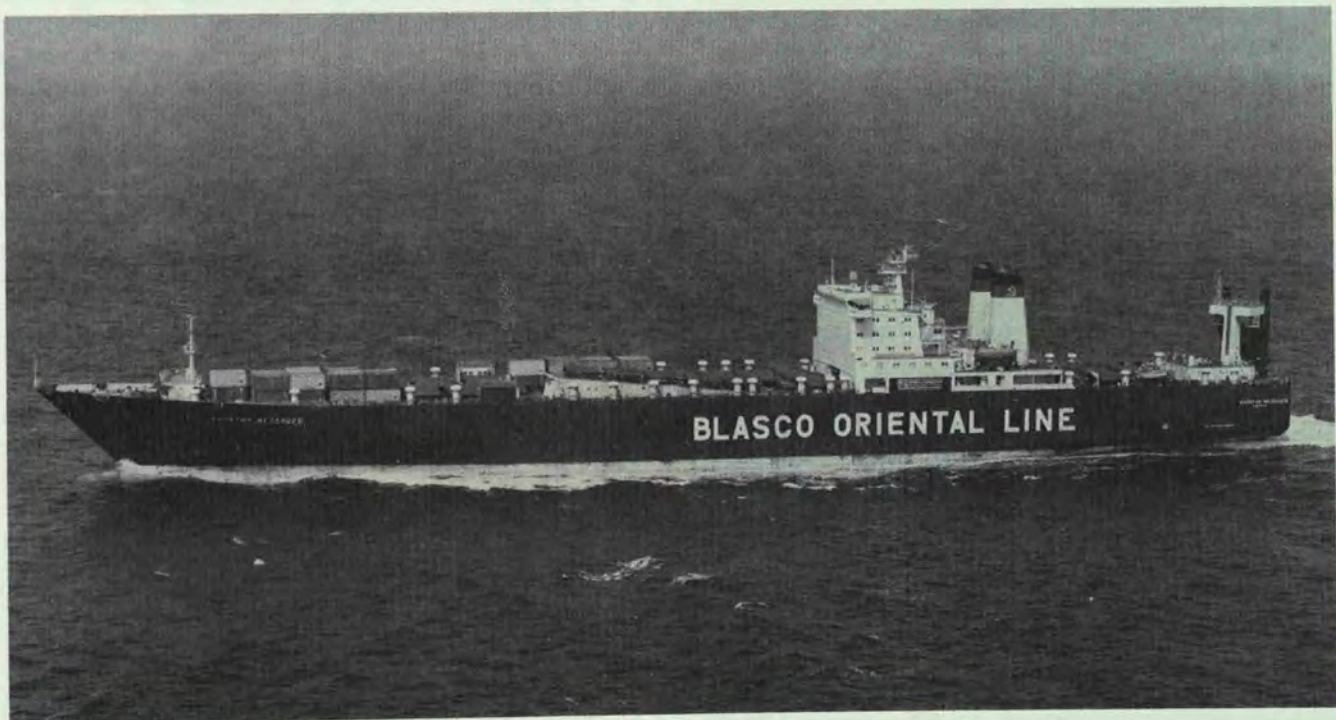
INZHENER YERMOSHKIN is one of four units of the Soviet-built KAPITAN SMIRNOV-Class roll-on/roll-off ships. These 20,000 deadweight ton ships are the fastest ships in the Soviet Merchant fleet. Powered by two gas turbines, they have a cruising speed of 25 knots.
