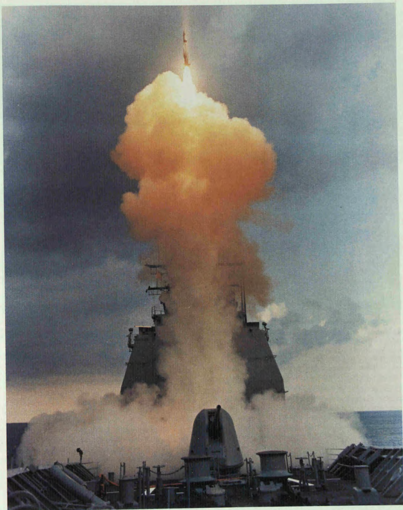
The Vertical Launch System is capable of firing anti-air or anti-surface missiles. Combined with the AEGIS radar, VLS provides the US Navy with quick-reaction, high-firepower, and improved electronic countermeasures.
