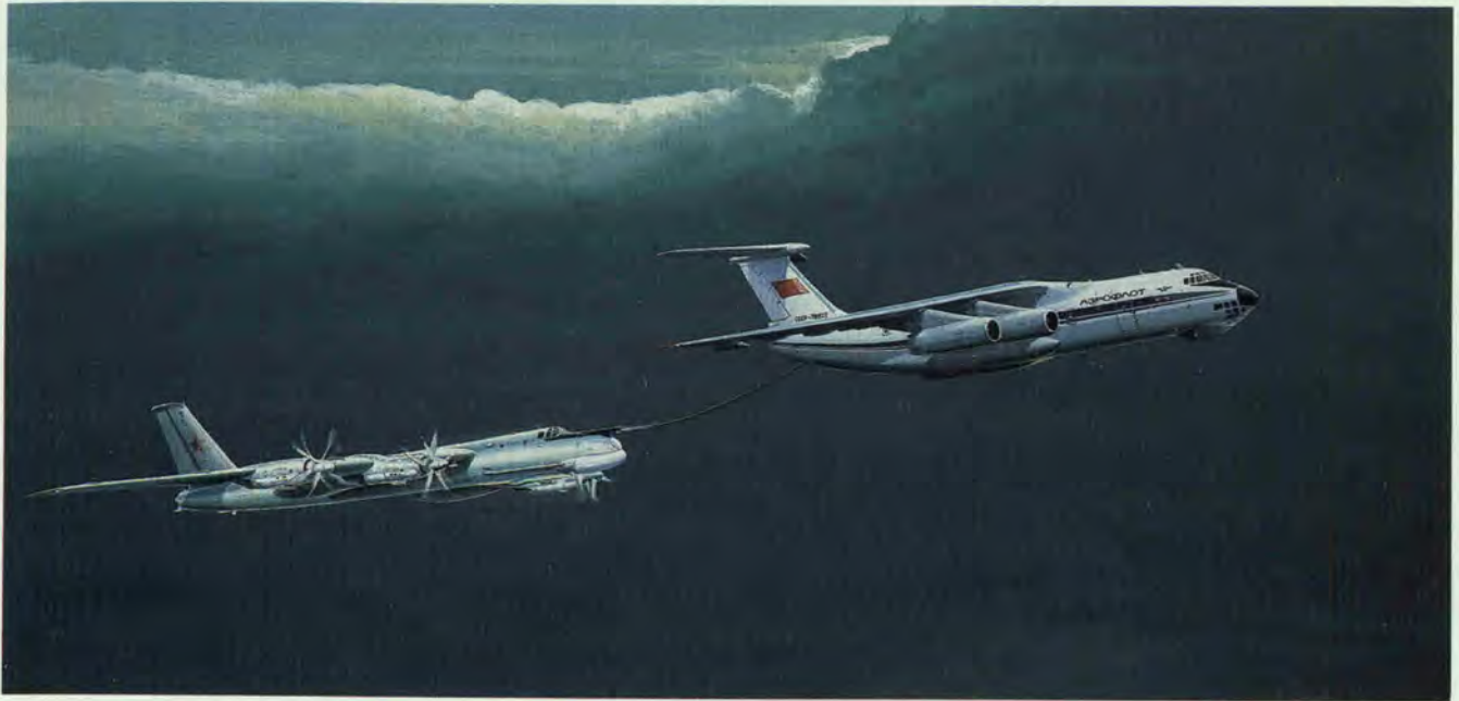
The MIDAS tanker aircraft, which became operational in 1987, will be used to support strategic bombers such as the BEAR H and possibly tactical and air defense aircraft. In peacetime, in-flight refueling extends the Soviets' reach farther from their homeland.
