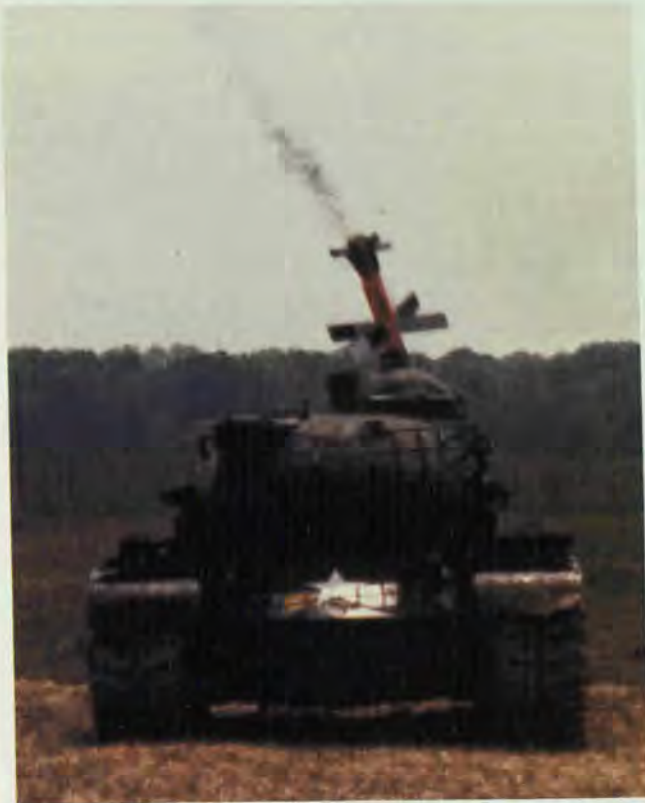
The Fiber-Optic Guided Missile is in development to defeat advanced helicopter and armor threats. Pictured is an early experimental firing demonstrating the potential of its antiarmor mission.
