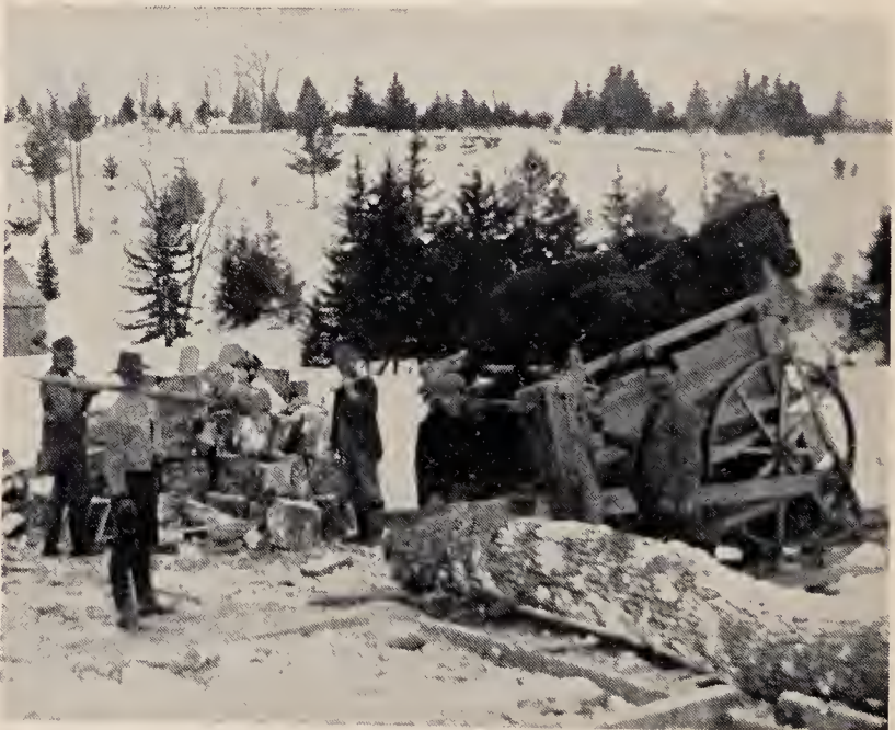
1881 (2 h.p.) horse treadmill saw rig, the most up to date of its day. Owner John Pike made a living with it, farm to farm.
