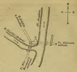
The dotted line in the plan expresses the modern part of the bridge: the strong lines the ancient work. But of the latter, there are only foundations, with the exception of the spur C, which is entire. The upper parts of the piers and the three paved causeways are modern. The causeway AB is twenty-four paces in length. The ancient masonry is of the same regular kind as that of Messene, and is probably of the same date.
