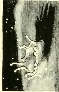
ENGRAVINGS OF INSTANTANEOUS PHOTOGRAPHS OF THE SPLASH OF A DROP OF WATER FALLING 40 CM. INTO MILK. Scale about six-tenths actual size.
