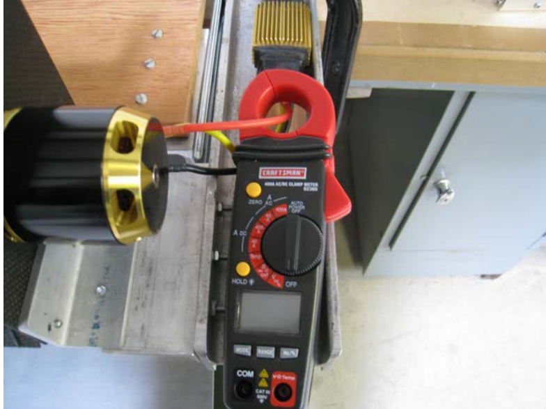
Figure 17. An ammeter measuring the current to the motor.
