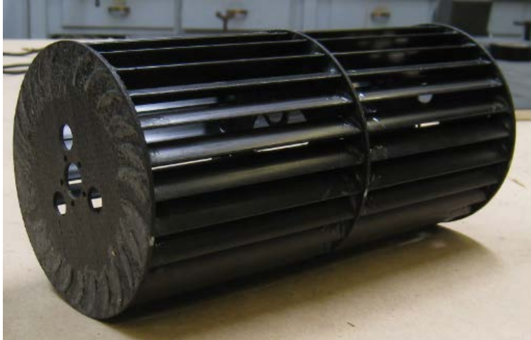
Figure 10. The complete manufactured 26-bladed rotor.
