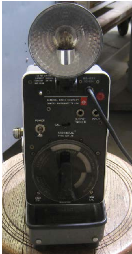
Figure 16. The strobe used to monitor the rotor speed.
