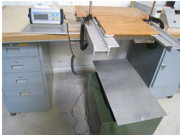
Figure 18. The digital scale used to measure thrust.
