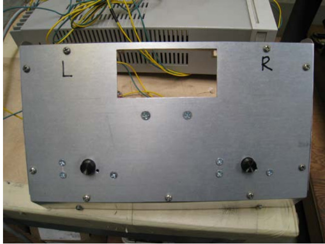
Figure 15. The speed control consoleA Type 1531-AB Strobotac stroboscope, shown in Figure 16, was used to measure the speed of the rotor.
