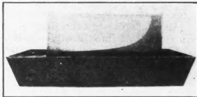
FIG. 1. OIL RISING BETWEEN CONVERGING SURFACES
