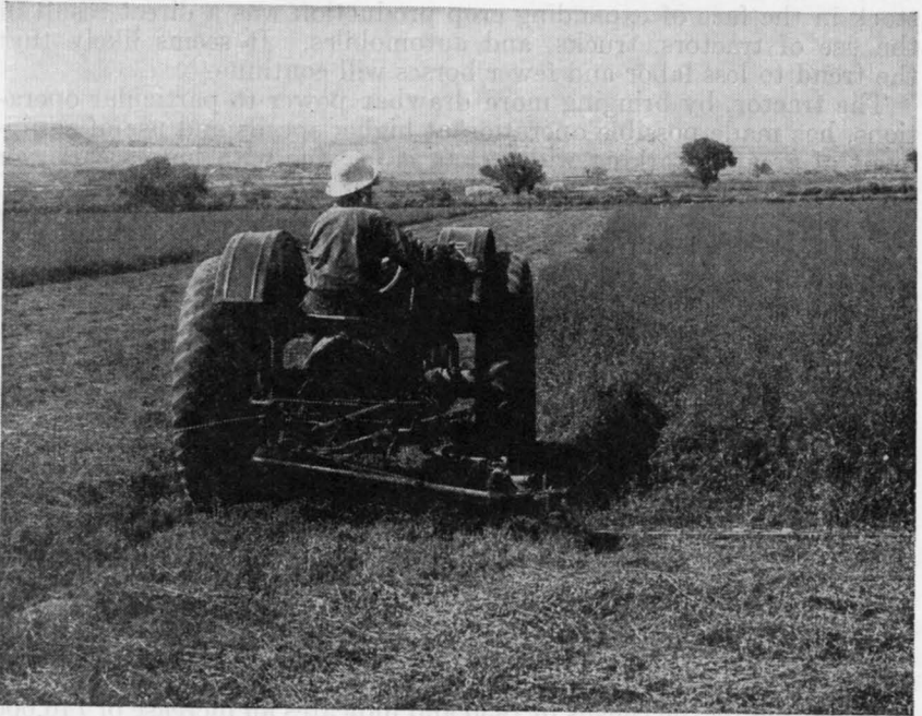
Figure 1.—Tractors equipped with rubber tires have a wider range of usefulness and a longer working life, yet cost less to operate and repair than those not so equipped. Their increased use in the past few years has been revolutionary in the farm machinery field.
