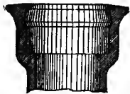
FIG. 197.—Socket of cast-iron special fit- ting of the Durham System.
