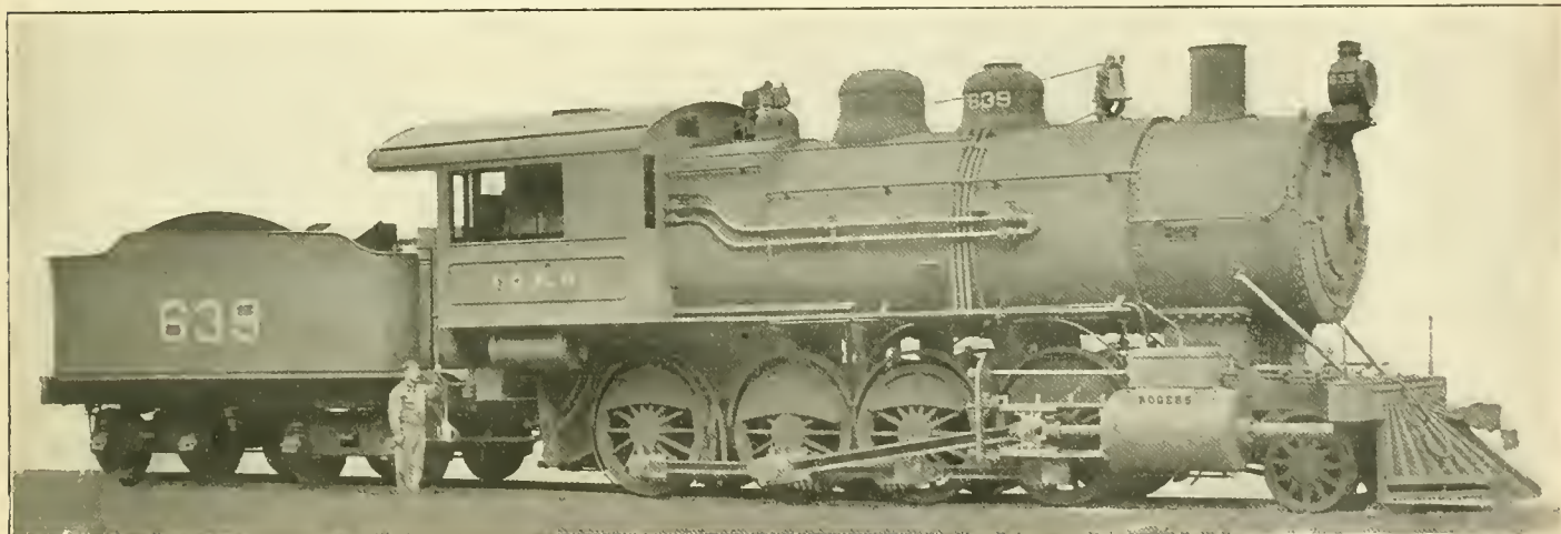
HUGE ROGERS CONSOLIDATION FOR ILLINOIS CENTRAL, BUILT BY ROGERS LOCOMOTIVE COMPANY, PATERSON, N. J., MR. W. RENSHAW SUPERINTENDENT OF MACHINERY.
