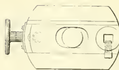
Drill Press Attachment for Turning Rocker Arm Ends
