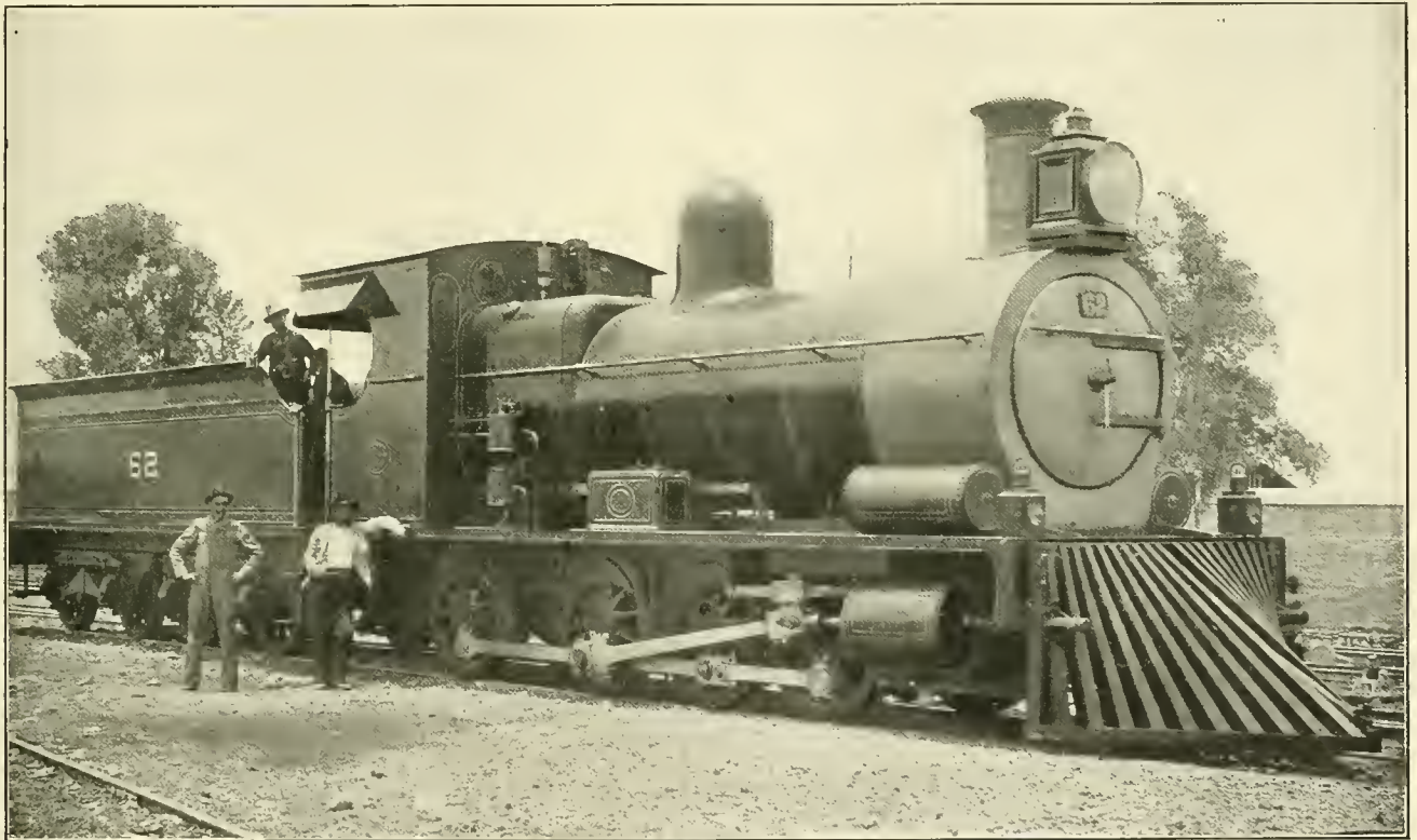
MEXICAN CENTRAL ENGINE—RESERVOIRS OVER CYLINDERS. (KINDNESS OF N. BARRETT.)
