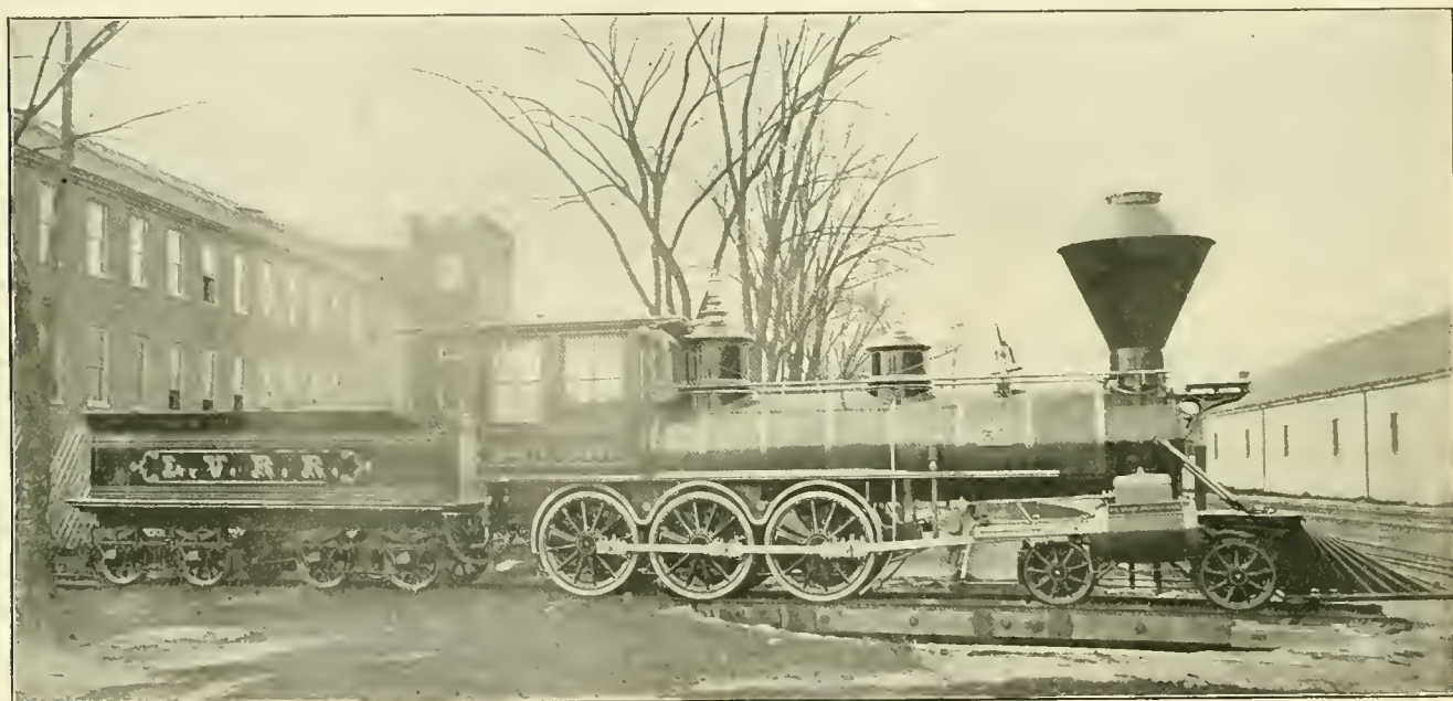
ONE OF THE FIRST TEN-WHEELERS OF THE LEHIGH VALLEY ROAD; MAIN DRIVERS AHEAD.
