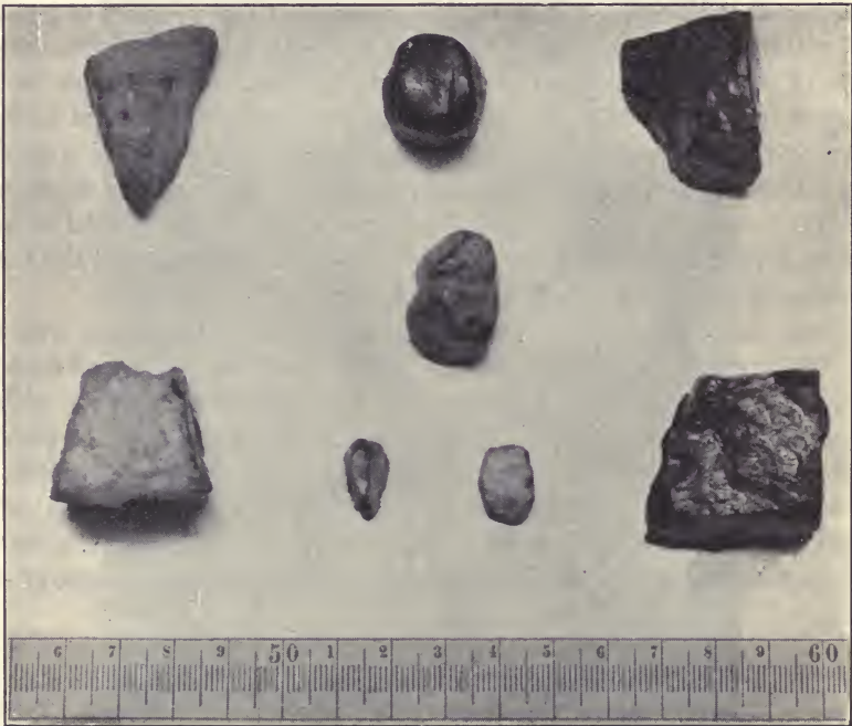
FIG. 1.—SAMPLES OF OIL- AND GAS-BEARING SANDS DIPPED IN PARAFFIN; THE SCALE READS IN CENTIMETERS.
