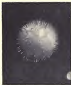
FIG. 2.—OIL FILM AROUND AN AIR BUBBLE. \times 450 .
