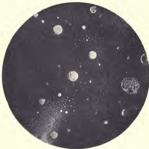
FIG. 8.—PARTLY EMULSIFIED OIL. \times 450 .
