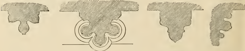
Fig. 1104. NAVE, VAULTING SHAFTS.
