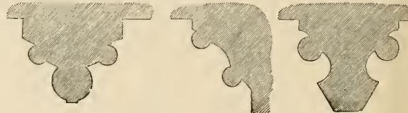
Fig. 1101. NAVE AND AISLES, Aisles, Transverse Rib, and Diagonal. TINTERN ABBEY, VAULTING SHAFTS.
