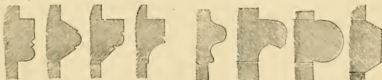
Fig. 1110. Fig. 1110a. Fig. 1110b. Fig. 1110c. Fig. 1115. Fig. 1114. Fig. 1111. Fig. 1112. NORMAN PERIOD. FOUNTAINS ABBEY. SAVE CLERESTORY, AISLE.
